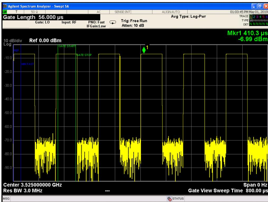
Figure 4-3. Gate View Showing Transmitter Output Power vs Time
