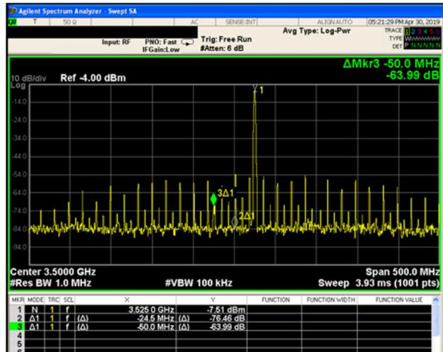
Figure 4-2. Spectrum of Transmitter Output with Gating On vs Off
