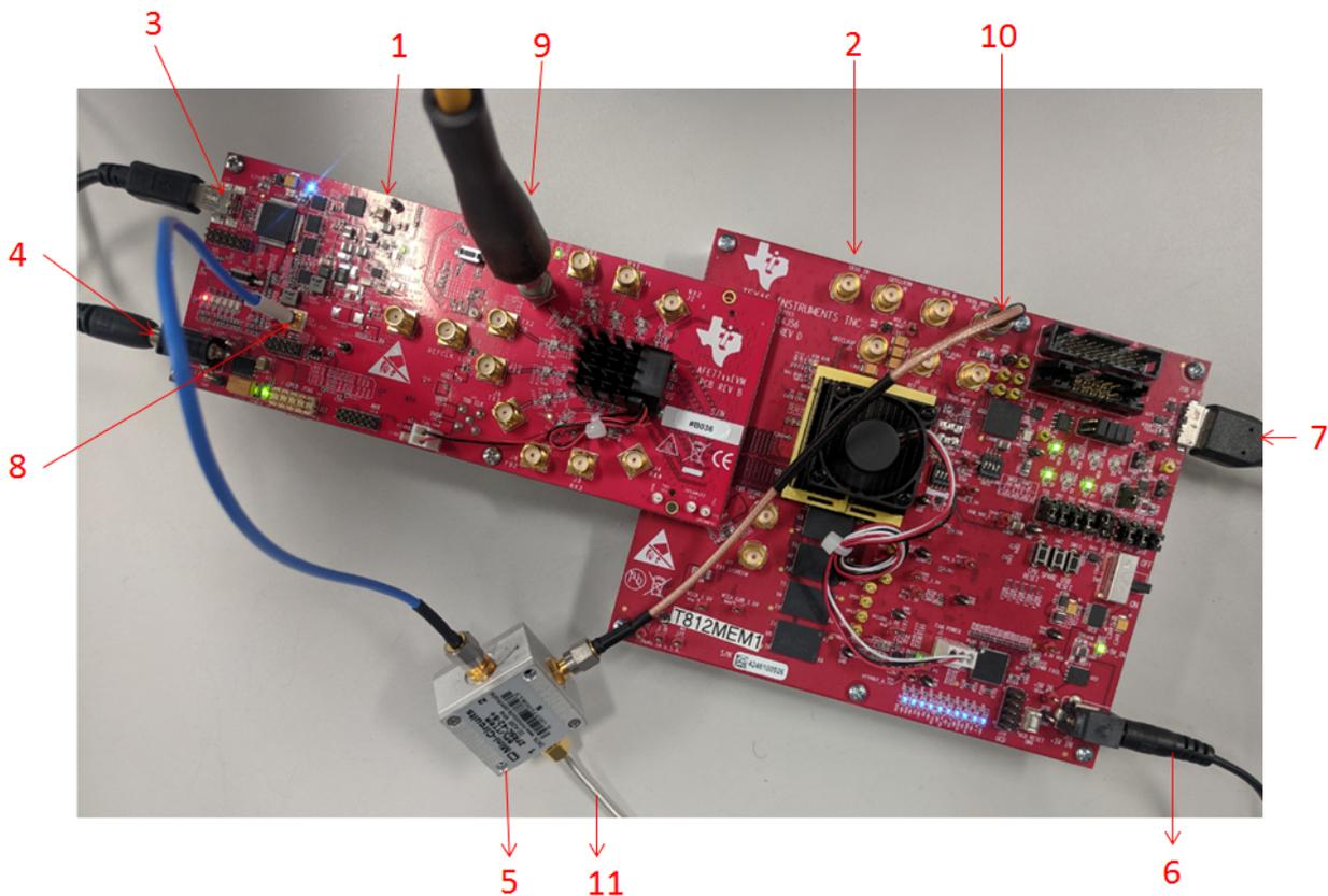
**Figure 3-1. Setup for TDD Mode Evaluation**
