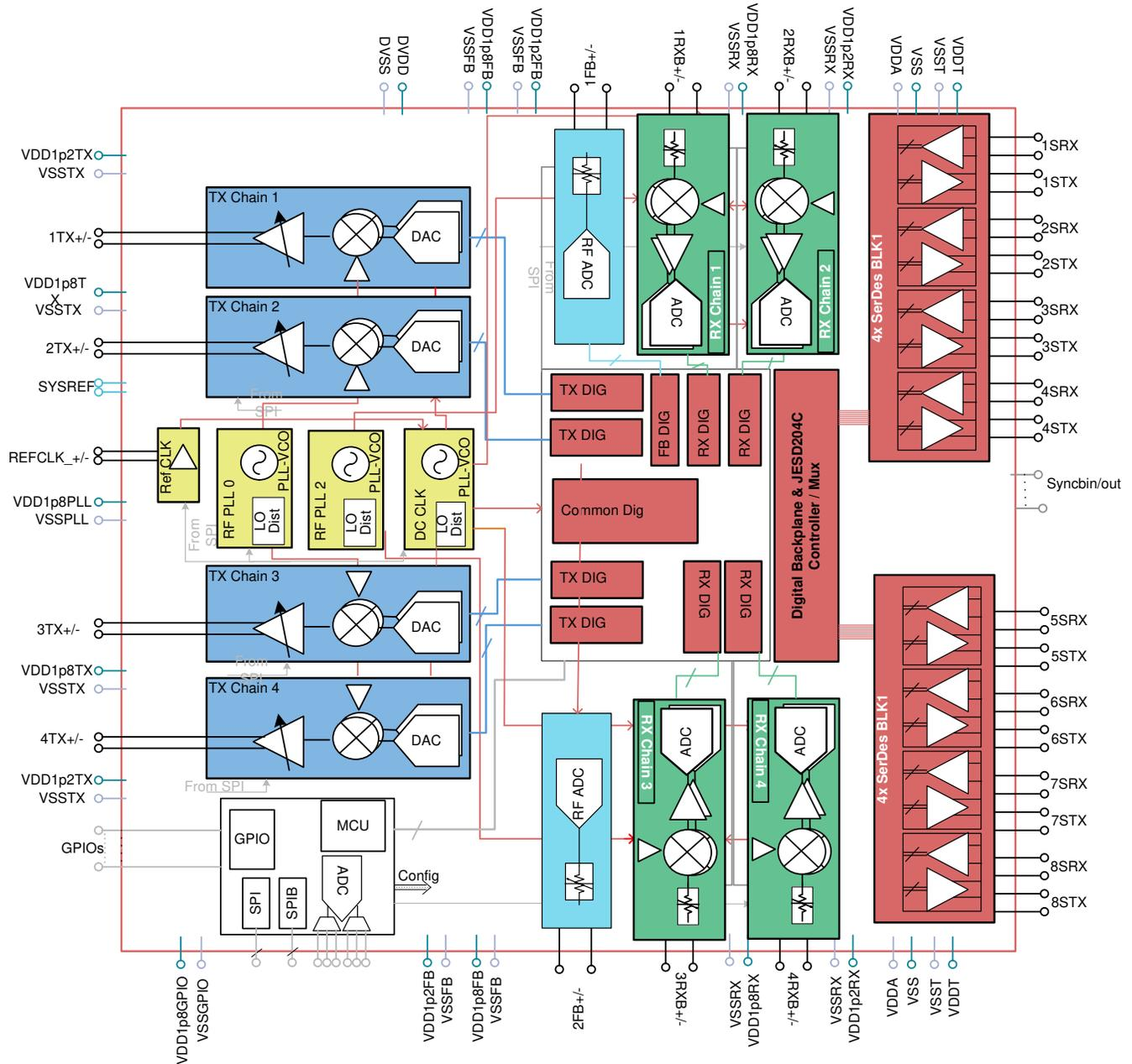
Figure 2-1. Block Diagram of the AFE77xx
