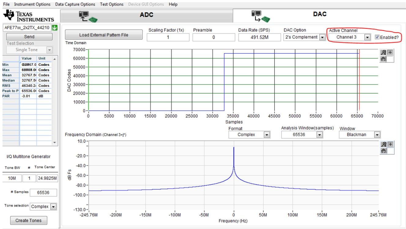
Figure 4-1. HSDCPRO DAC Tab Showing the TDD Test Pattern on Channel 3
