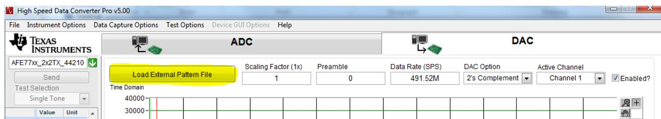
**Figure 3-2. Interface of HSDCPRO Showing Button to Load External Test Pattern File**
