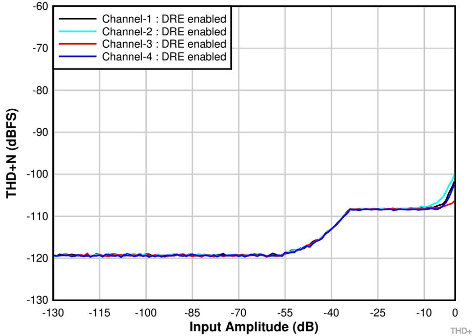
Figure 5-2. THD+N Performance Measurement with DRE Enabled
