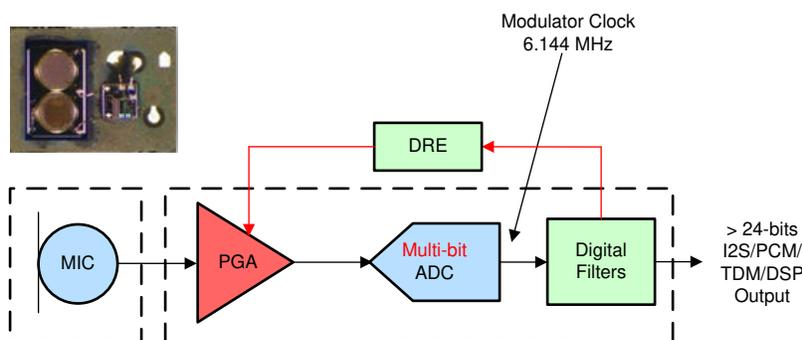
Figure 3-2. Analog Microphone with ADC for Multi-bit Output
