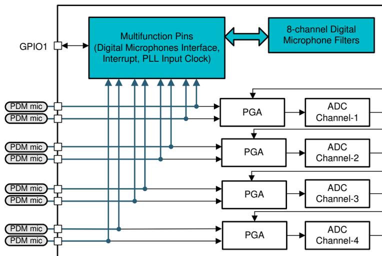
Figure 6-3. Digital PDM Microphones System Block Diagram
