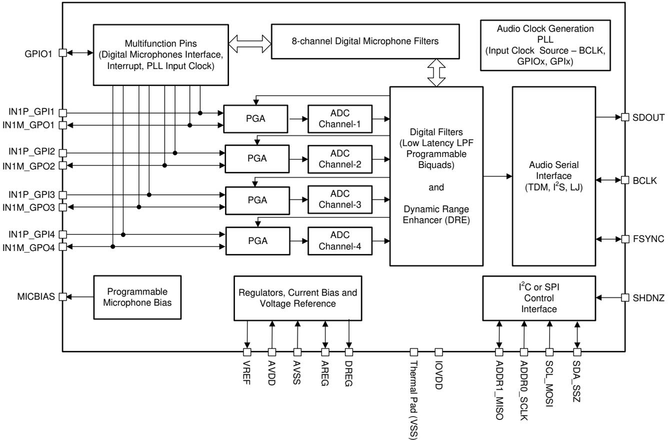
Figure 6-1. Internal Block Diagram of the TLV320ADC5140/PCM51x0-Q1
