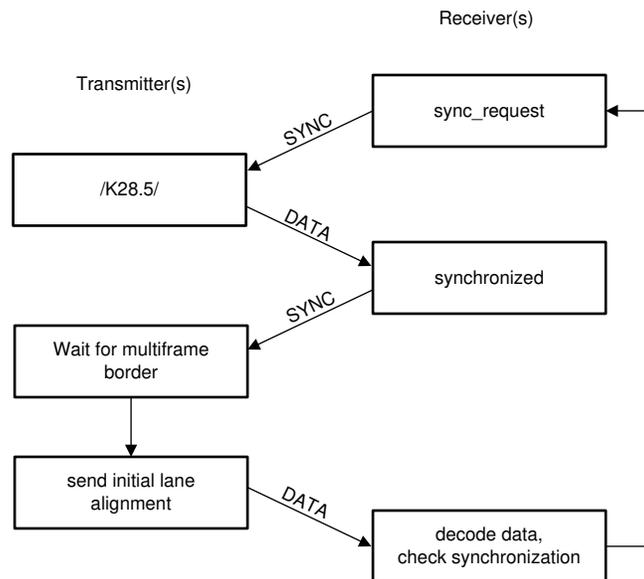
**Figure 6-1. Synchronization Process for Subclasses 1 and 2 <sup>2</sup>**
