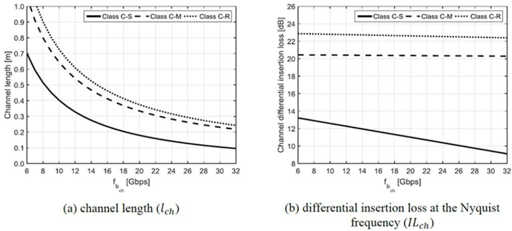
**Figure 5-1. Category C Channel Characteristics as a Function of a Channel Data Rate <sup>1</sup>**
