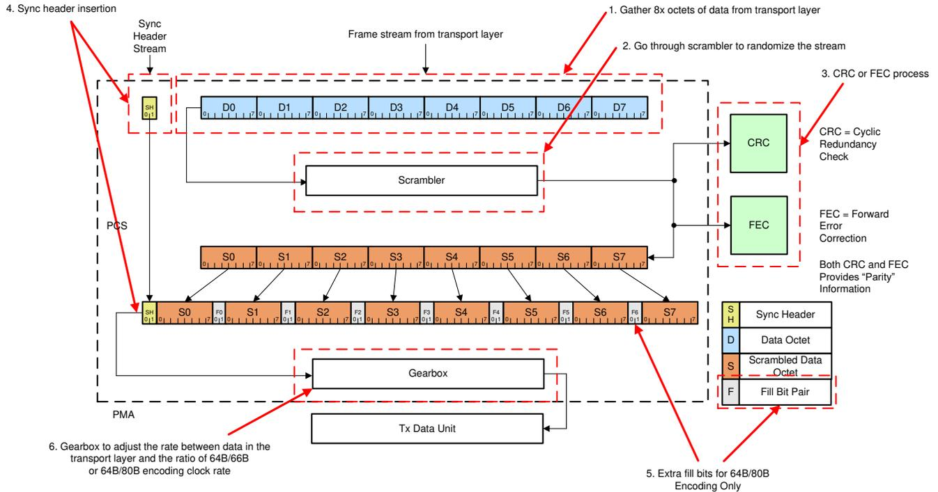
**Figure 6-2. 64B/66B and 64B/80B Encoding Process<sup>5</sup>**
