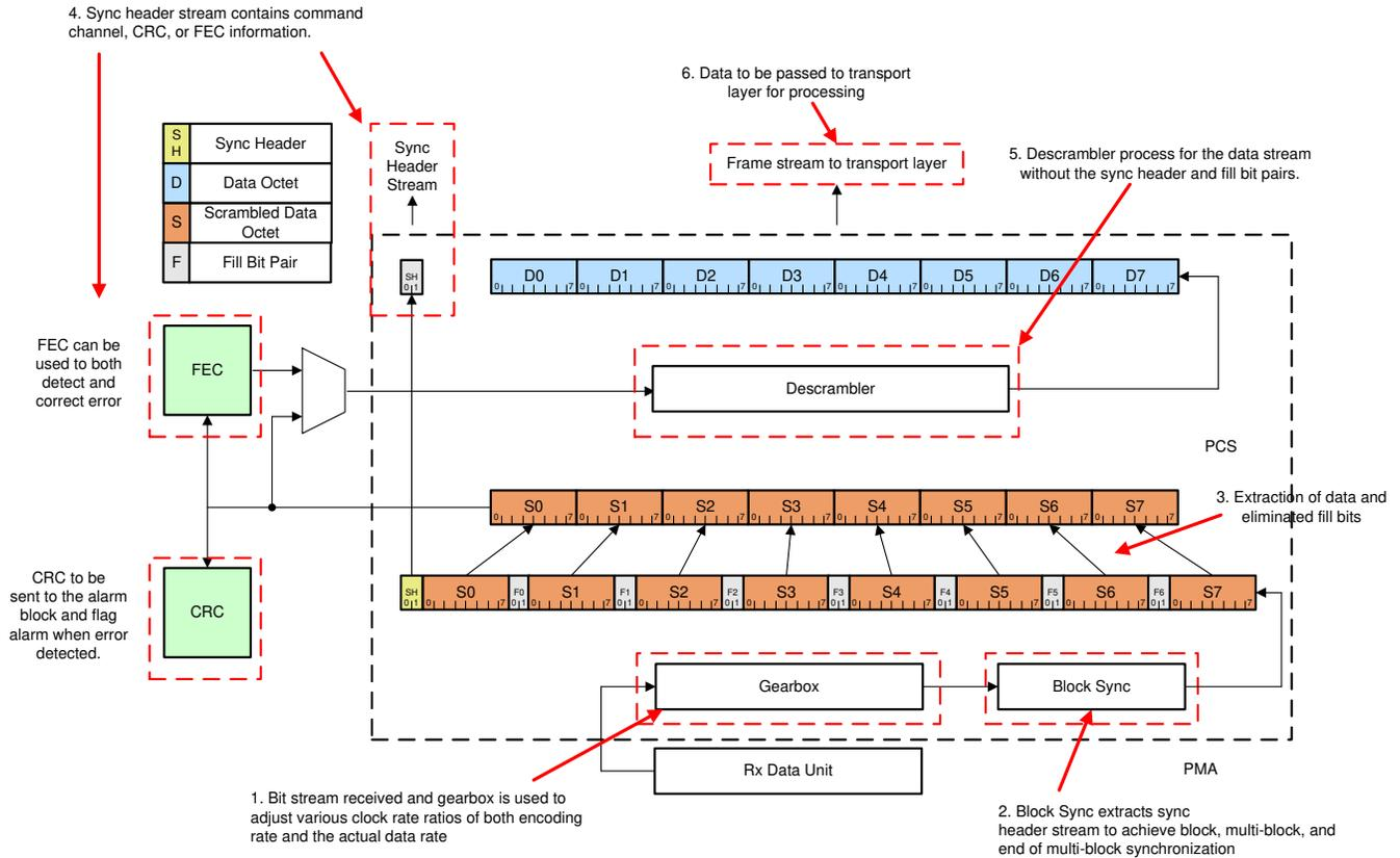
**Figure 6-3. 64B/66B and 64B/80B Decoding Process<sup>6</sup>**
