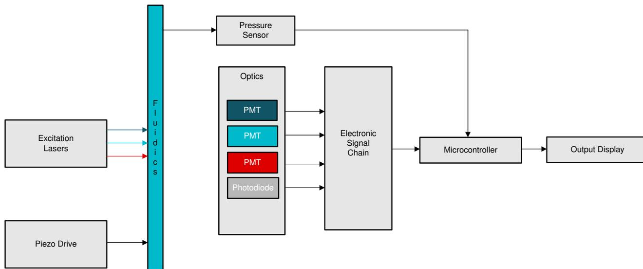
Figure 1-1. System Block Diagram of a flow Cytometer
