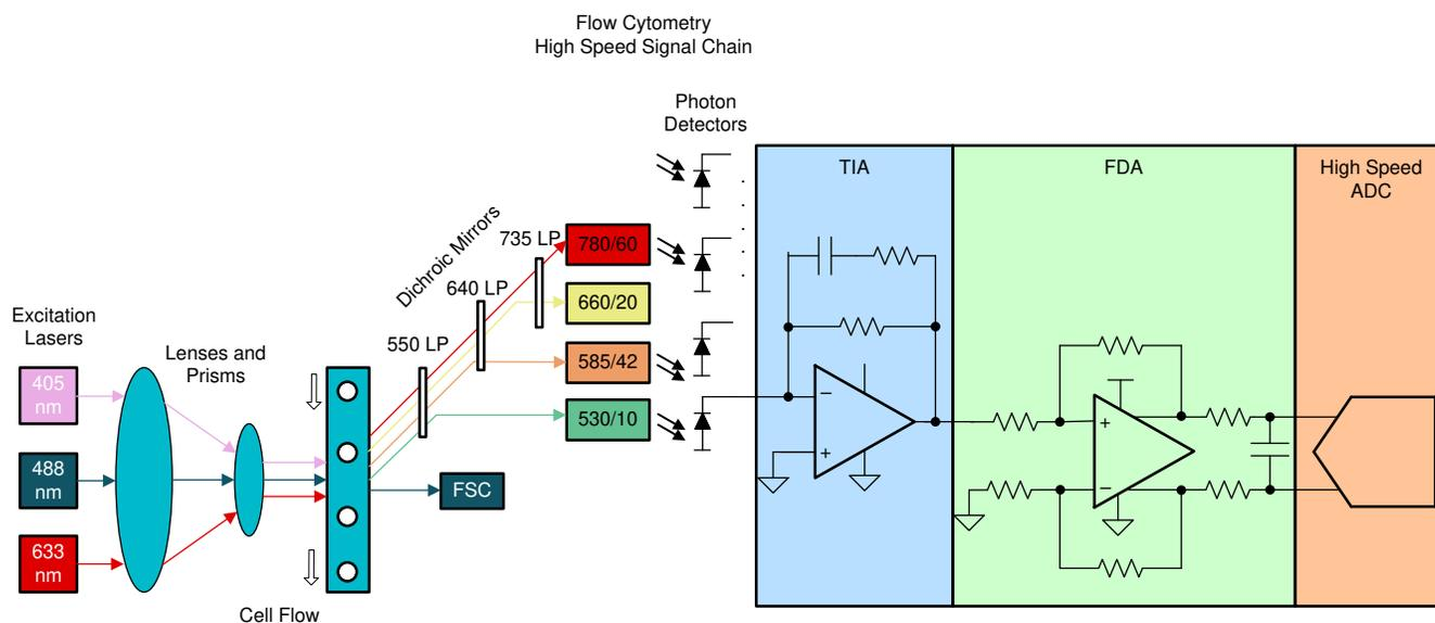
Figure 1-2. Analog Signal Chain of a Flow Cytometer
