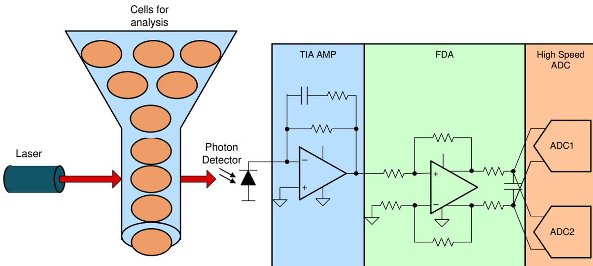
**Figure 3-3. Analog Signal Chain with a duplicate ADC channel**
