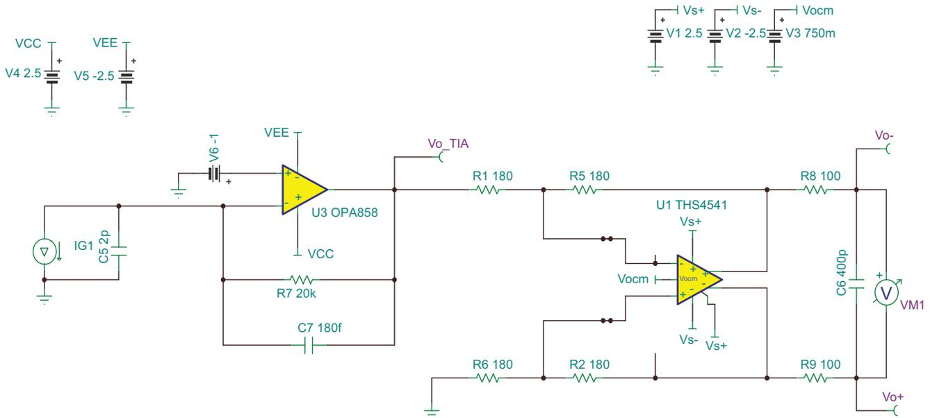
Figure 3-1. Transimpedance amplifier and Fully Differential Amplifier for photon detectors
