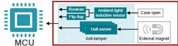
Figure 1-1. Smart Meter With Light Sensor Block Diagram
