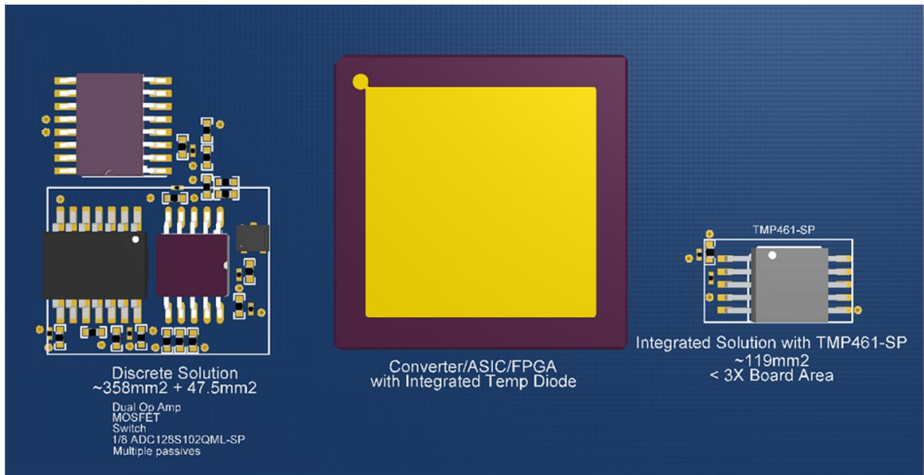
**Figure 3. Discrete Solution vs. TMP461-SP Layout**
