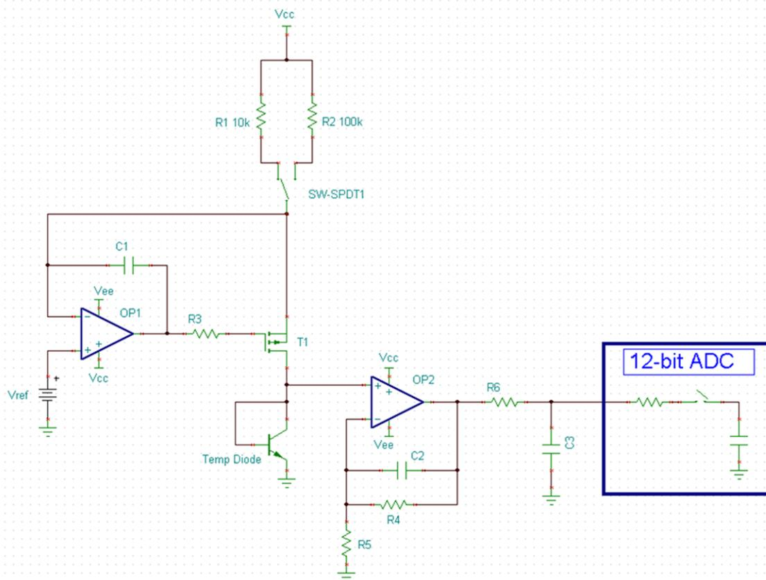
**Figure 1. Discrete Temperature Sensing Circuit**
