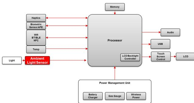
**Figure 1. Smart Watch Display Block Diagram**
