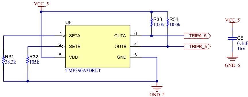
**Figure 1-8. Temperature Switch Schematic Using the TMP390**
