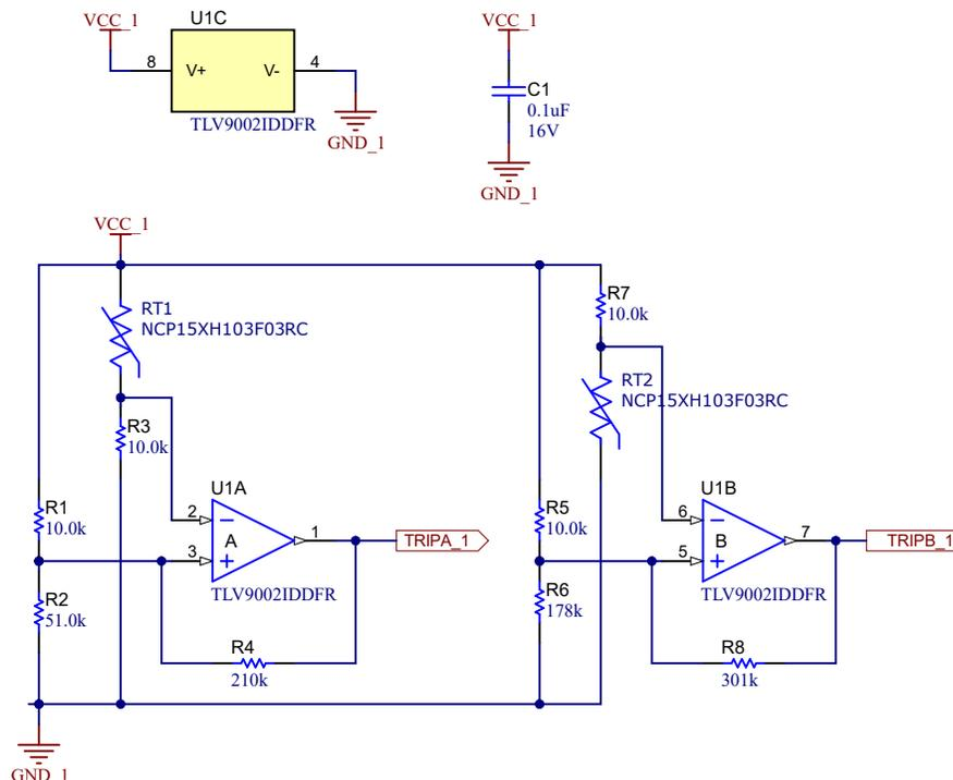
**Figure 1-2. Temperature Switch Schematic**
