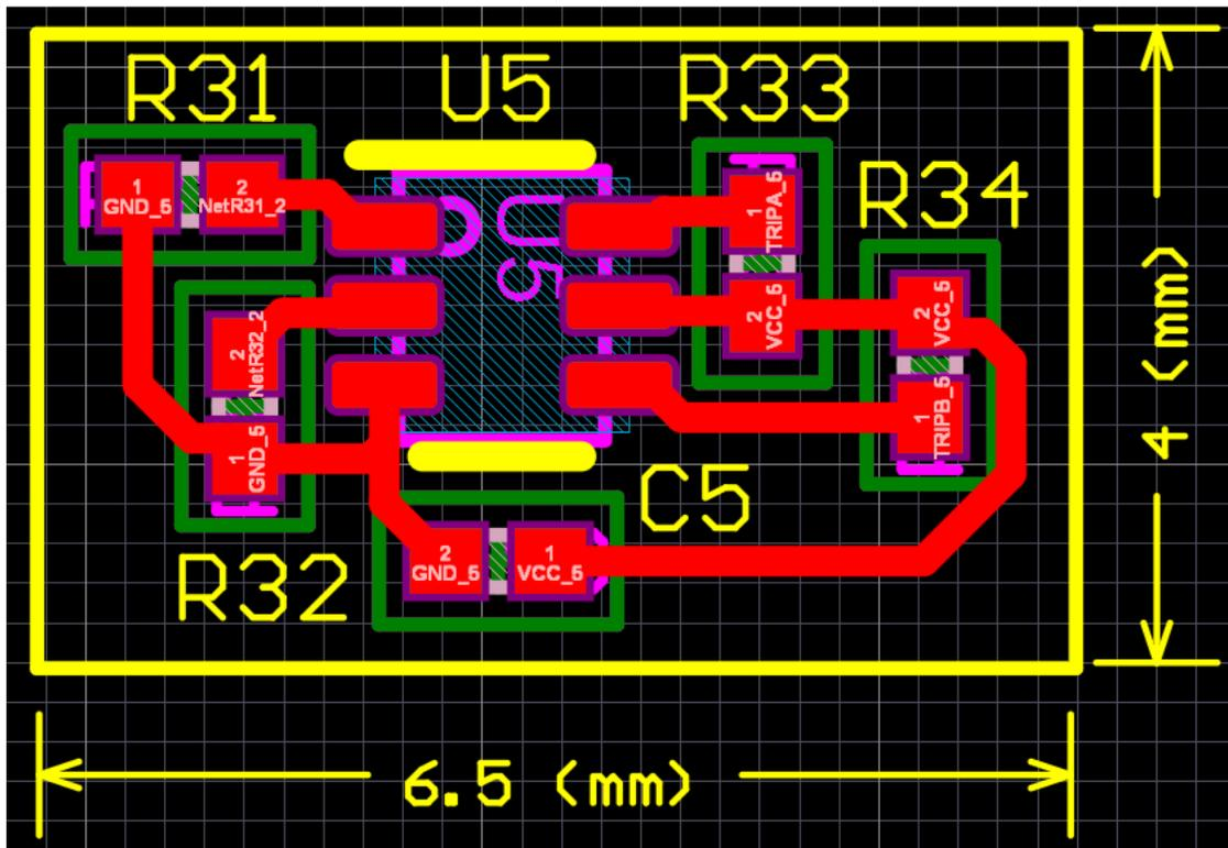
**Figure 1-9. Temperature Switch Layout Using the TMP390**
