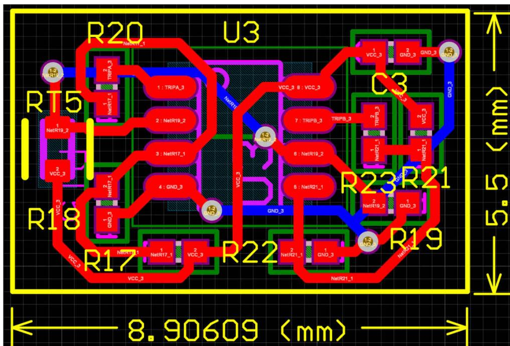
Figure 2-3. Temperature Switch Layout
