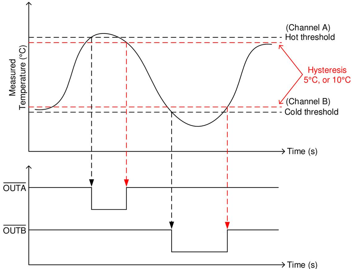
**Figure 1-1. Temperature Switch Output With Hot or Cold Thresholds and Hysteresis**
