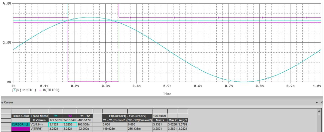
Figure 1-4. PSPICE Simulation Result of TRIPB\_1 Output
