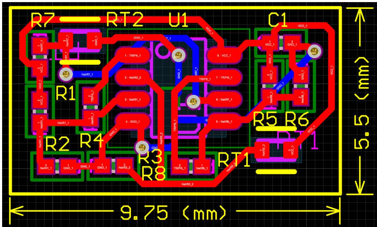
Figure 1-5. Temperature Switch Layout
