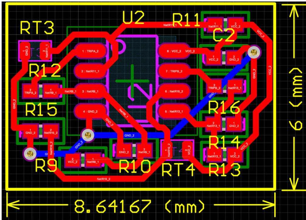
Figure 1-7. Temperature Switch Layout Using the TMP61
