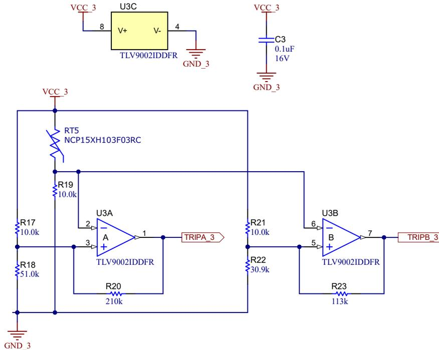
Figure 2-2. Temperature Switch Schematic
