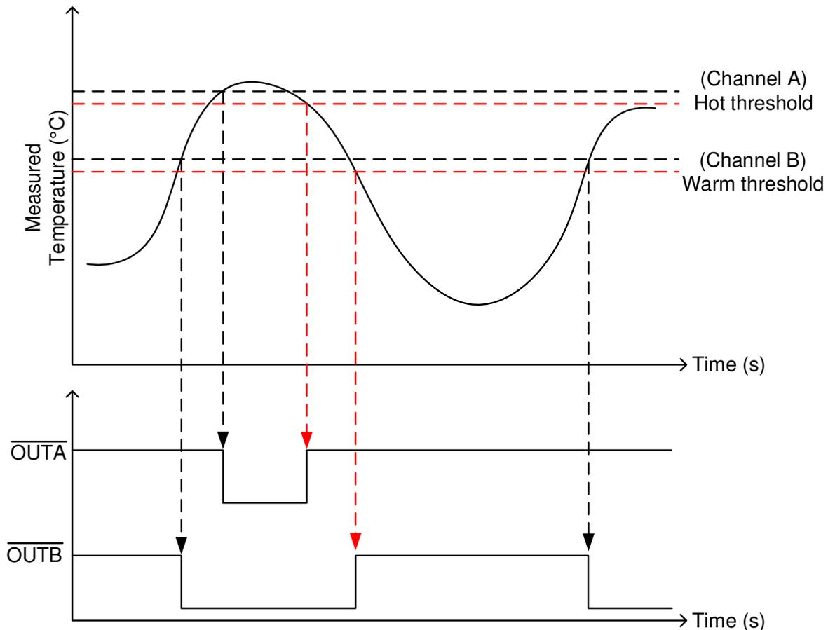
**Figure 2-1. Temperature Switch Output With Hot or Warm Thresholds and Hysteresis**
