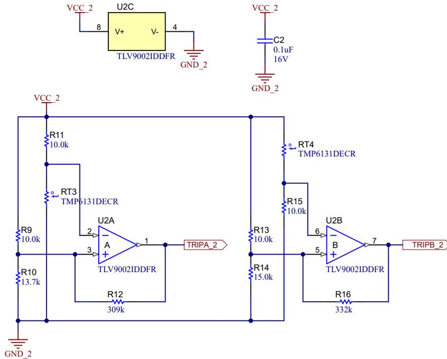
Figure 1-6. Temperature Switch Schematic Using the TMP61
