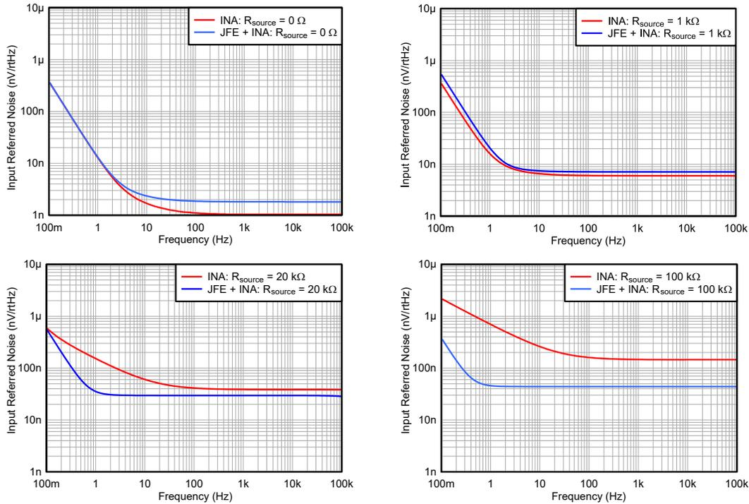
**Figure 3. Preamplifier Noise Comparison with Various Source Impedances**
