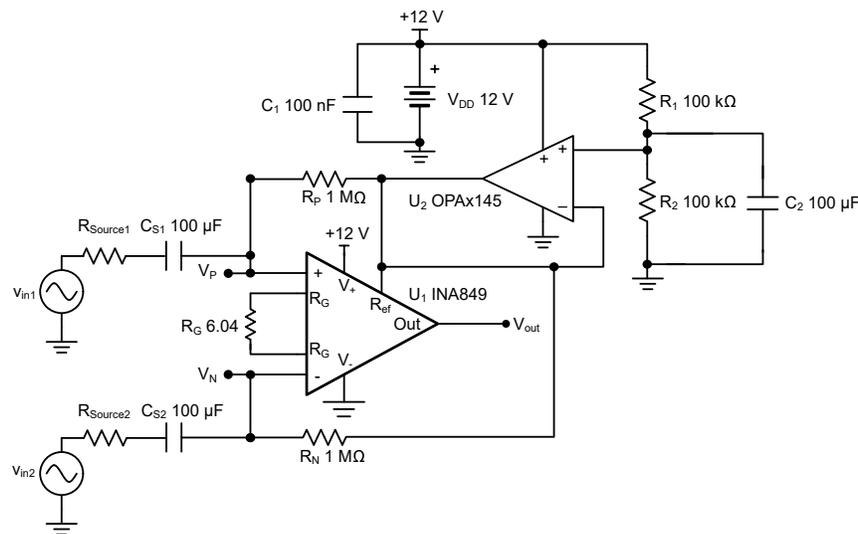
Figure 1. INA Preamplifier
