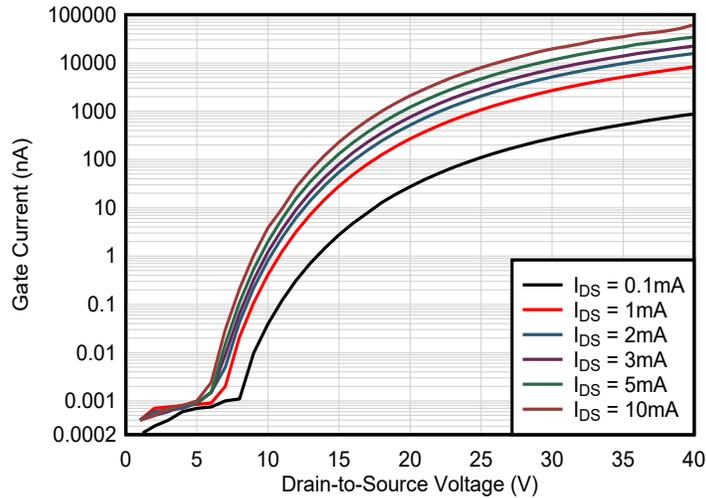
**Figure 5.  $I_G$  vs  $V_{DS}$**
