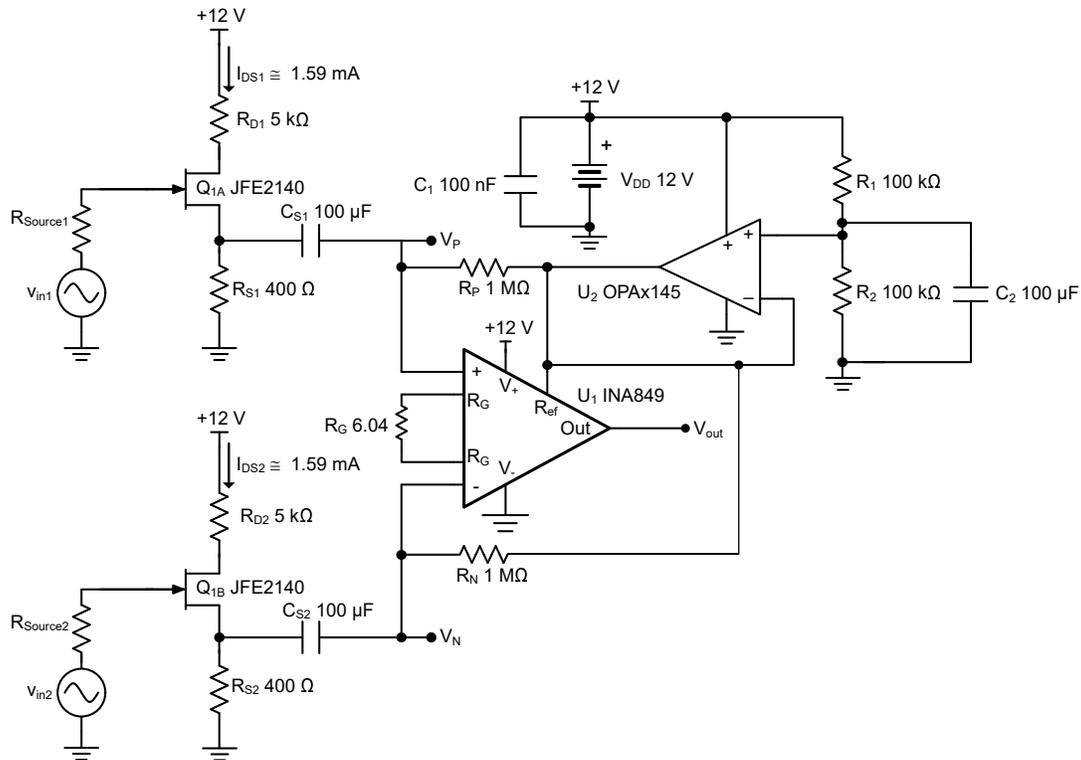
**Figure 2. Discrete JFET and INA Preamplifier**
