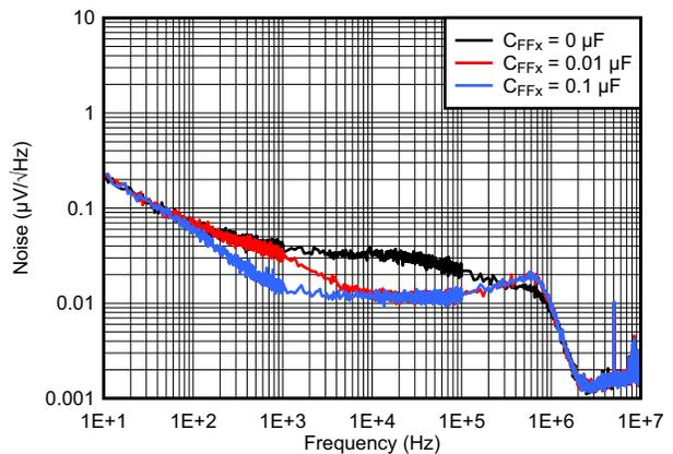
**Figure 2-7. Noise Versus Frequency and CFFx**
