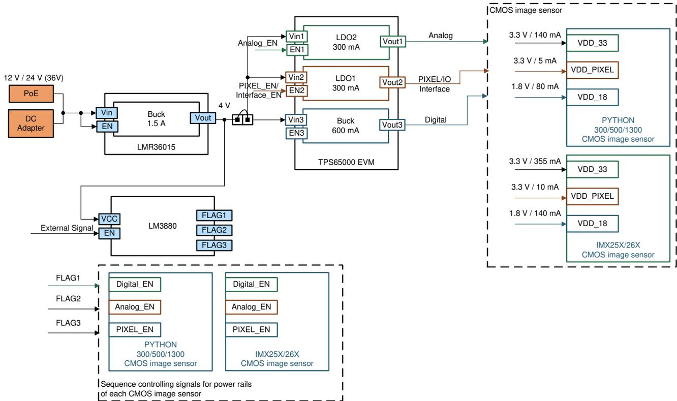
Figure 2-2. Block Diagram of PMIC TPS65000 Solution
