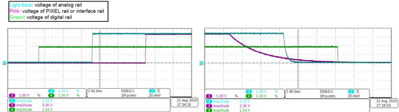
**Figure 4-1. Power Sequence of the Power Rails of PYTHON 300/500/1300 CMOS Image Sensors Using the 120-ms Delay Time LM3880**
