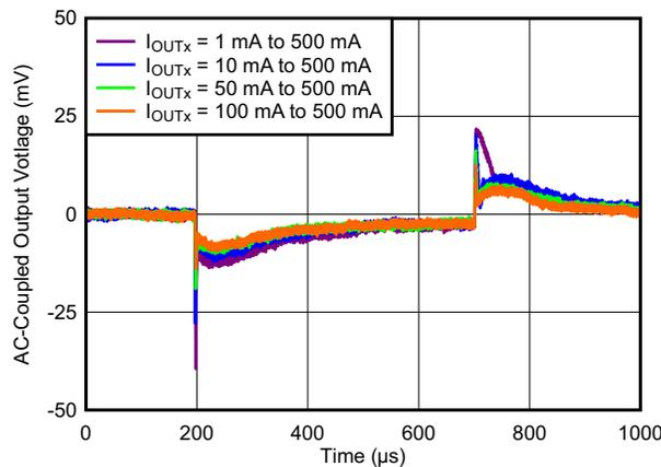
**Figure 2-8. Load Transient Response Versus Voutx**
