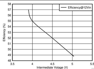
**Figure 4-3. The Relationship Between Efficiency of the Whole System and the Intermediate Voltage for Powering IMX25X/26X CMOS Image Sensors**
