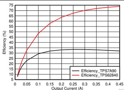
**Figure 3-2. Efficiency of the Digital Rail Supplied by TPS7A90 or TPS62840 in PYTHON 300/500/1300 CMOS Image Sensors**
