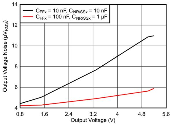
**Figure 2-6. Output Noise Versus Output Voltage**
