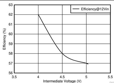
**Figure 4-2. The Relationship Between Efficiency of the Whole System and the Intermediate Voltage for Powering PYTHON 300/500/1300 CMOS Image Sensors**
