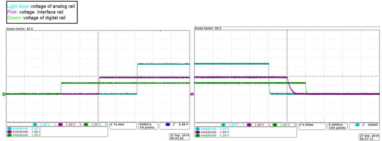
**Figure 3-5. Power Sequences of the Power Rails of IMX25X/26X CMOS Image Sensors**
