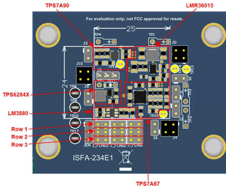
Figure 2-12. PCB Board of Discrete Solution
