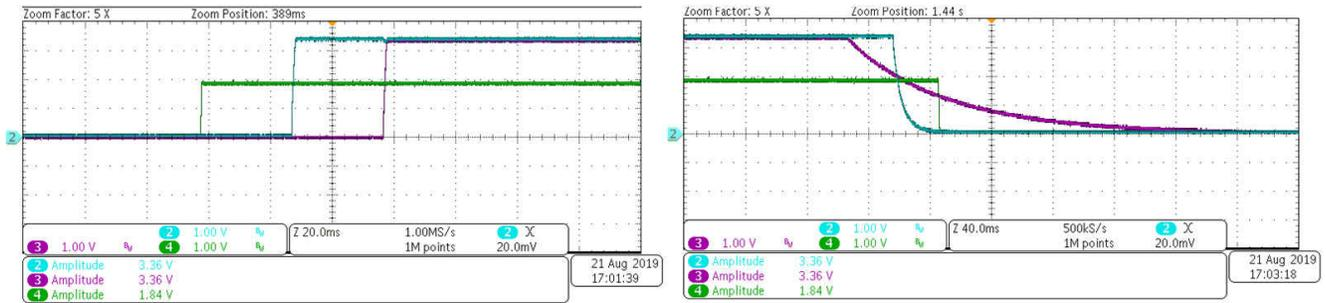
(a) Power Sequences of PYTHON 300/500/1300 CMOS image sensors' power rails
