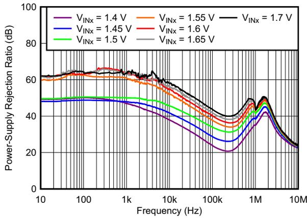
**Figure 2-4. Power Supply Rejection Ratio Versus Frequency and Input Voltage**
