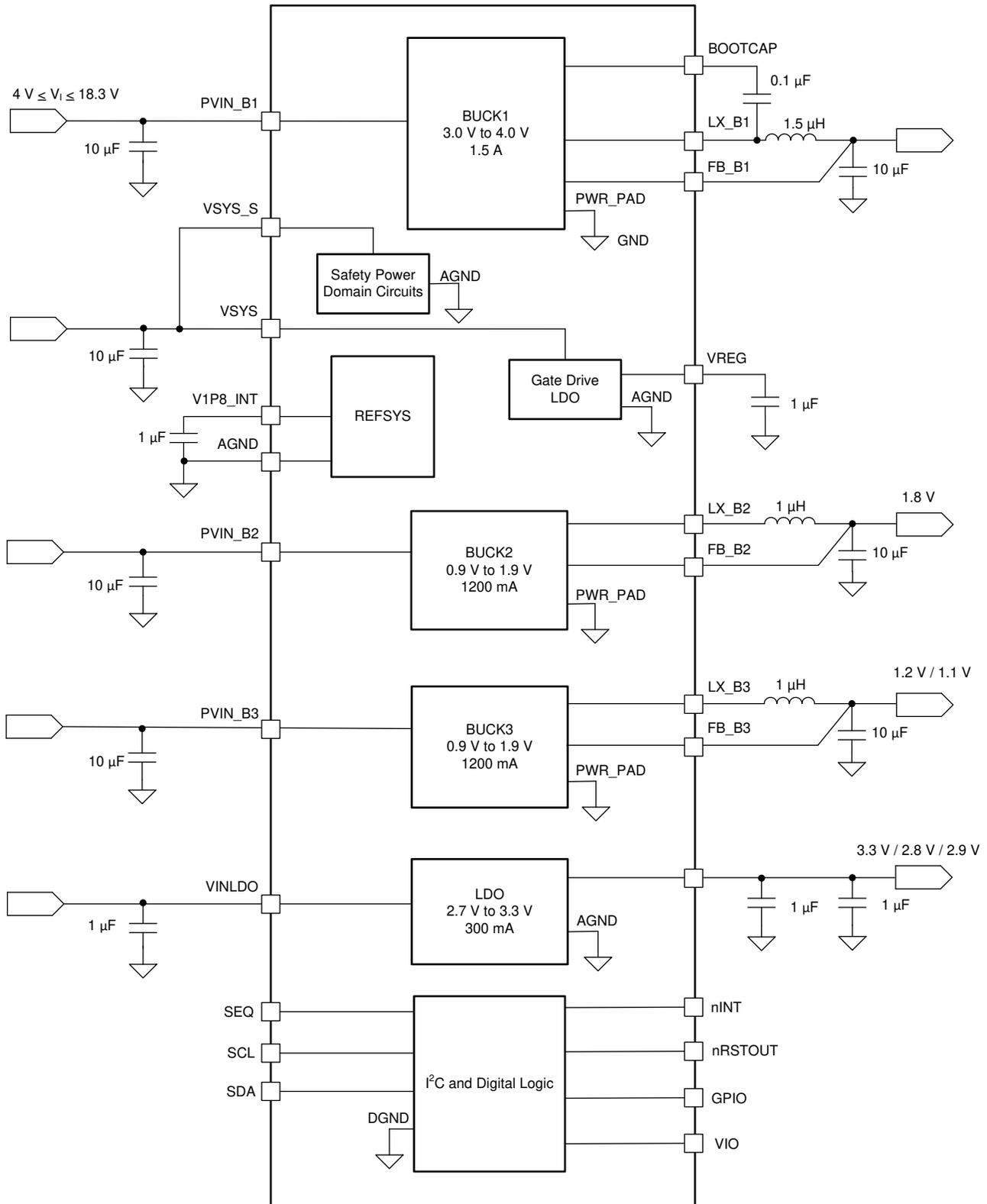
**Figure 2-14. Block Diagram of the TPS650330-Q1**
