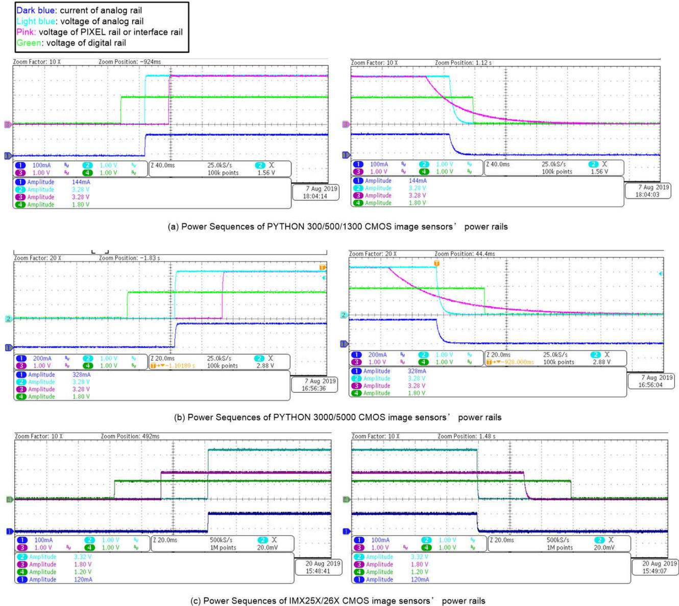
**Figure 3-1. Power Sequences of CMOS Image Sensor Power Rails**
