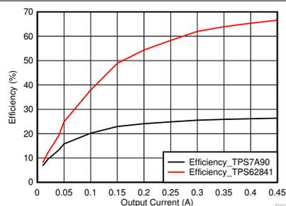
**Figure 3-3. Efficiency of the Digital Rail Supplied by TPS7A90 or TPS62841 in IMX25X/26X CMOS Image Sensors**
