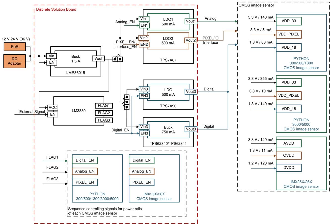
Figure 2-1. Block Diagram of Discrete Solution Board
