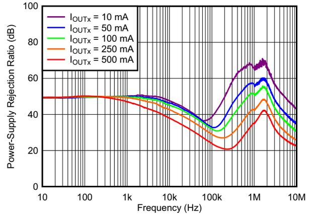
**Figure 2-5. Power Supply Rejection Ratio Versus Frequency and Output Current**
