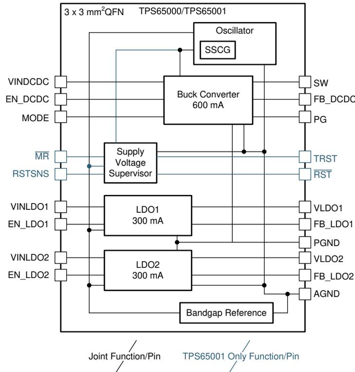
Figure 2-13. Block Diagram of the TPS65000
