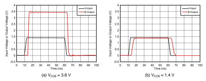
Figure 5. A-to-B Switching Waveforms with  $V_{CCA}$  (Input) = 1.4
