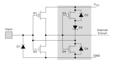
Figure 10. Bus-Hold Circuit
