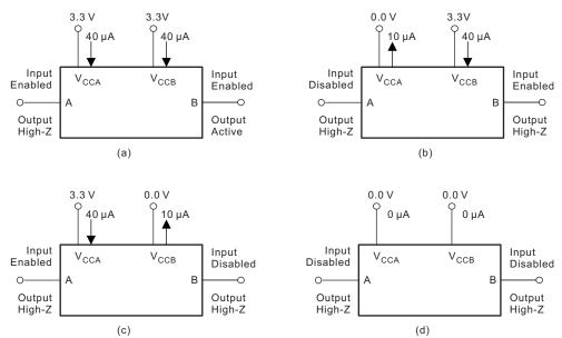
Figure 8. Graphical Depiction of I<sub>CC</sub> and I/O Port States for Partial-Power-Down Conditions (A-to-B Mode)
