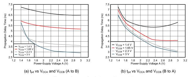
Figure 6. Propagation Delays vs  $V_{\text{CCA}}$  and  $V_{\text{CCB}}$
