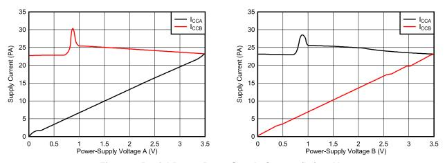
Figure 9. Partial-Power-Down Supply Current (Icc) vs Vcc
