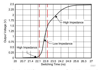
Figure 7. Typical AVCx164245 Output Switching Waveform
