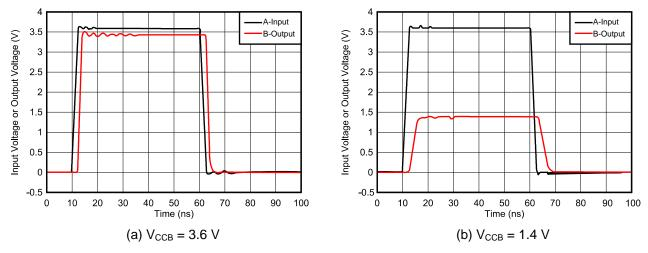
Figure 4. A-to-B Switching Waveforms With  $V_{CCA}$  (Input) = 3.6 V
