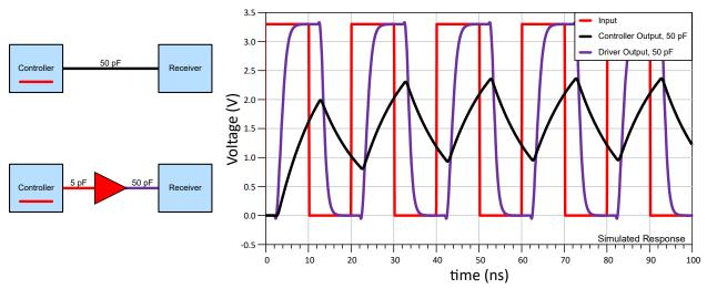
Left: block diagrams for signal redriving. Right: simulated input (red) and output signals with weak controller (black) and typical buffer driver from the LVC logic family (purple).
