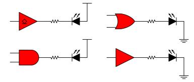
Figure 3-1. Using Logic to increase LED Drive Strength.
