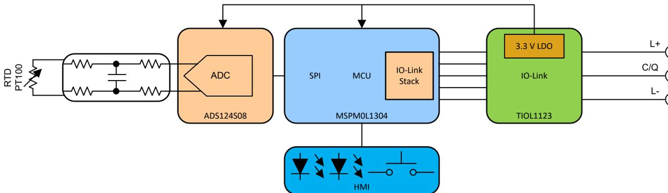
**Figure 4. Block Diagram of RTD Temperature Transmitter Based on MSPM0L1304**
