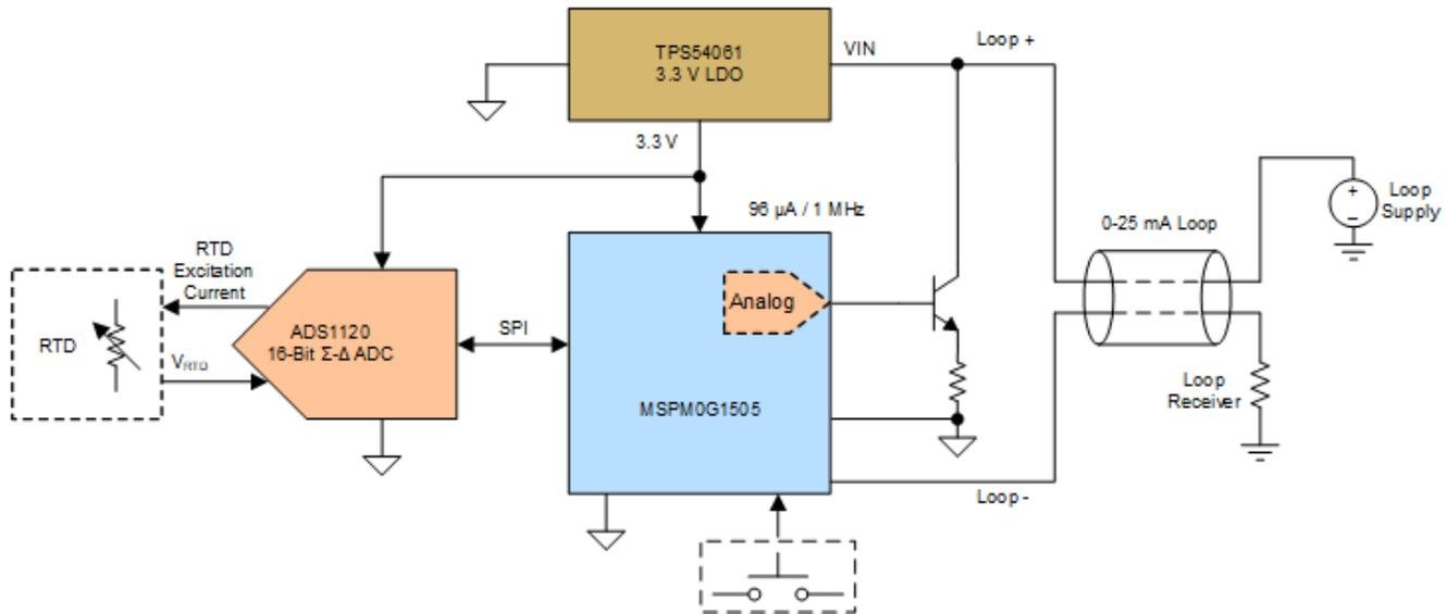
**Figure 2. Block Diagram of RTD Temperature Transmitter Based on MSPM0G1505**
