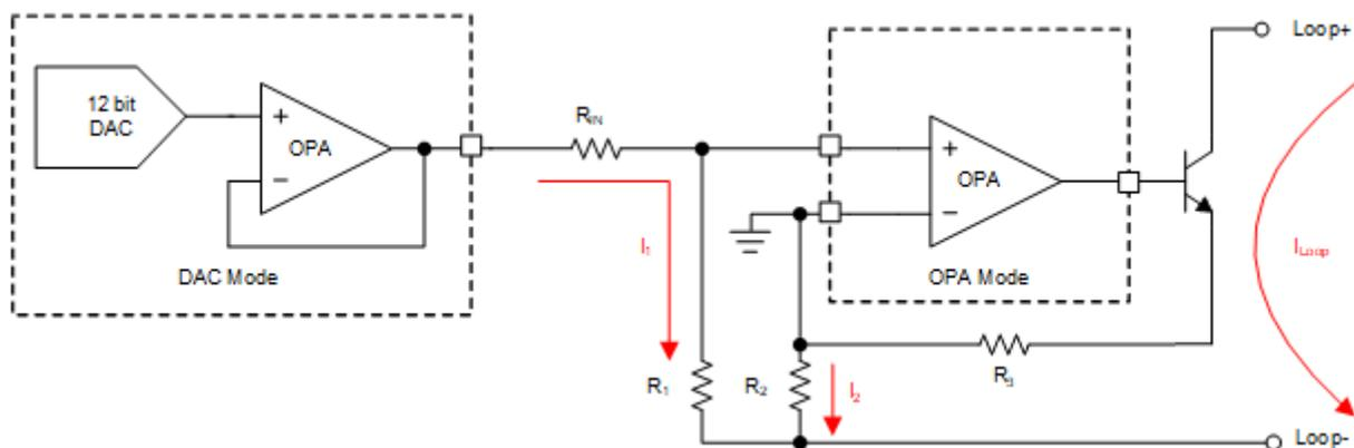
**Figure 3. Configuration and Connections of MSPM0G1505 Internal Analog**
