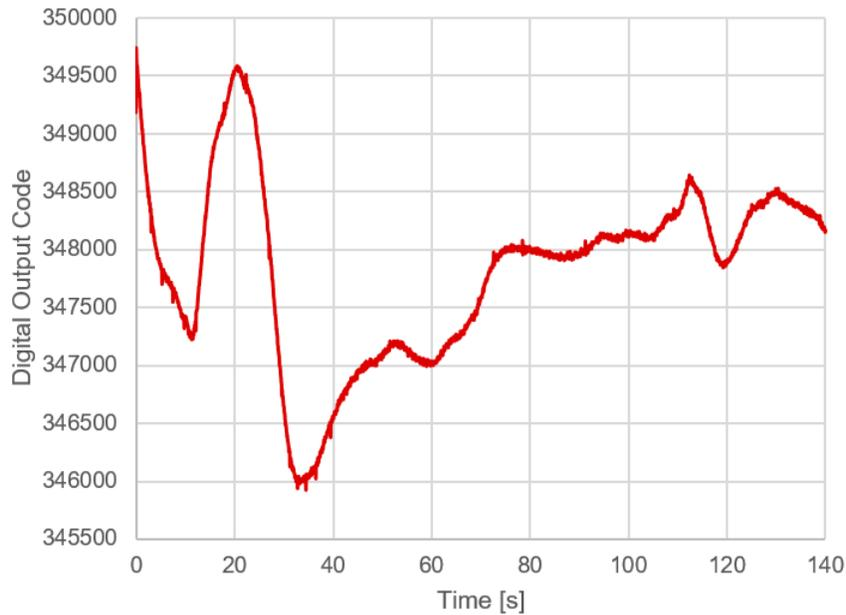
**Figure 3-3. PIR Sensor Signal Drift Over Time**
