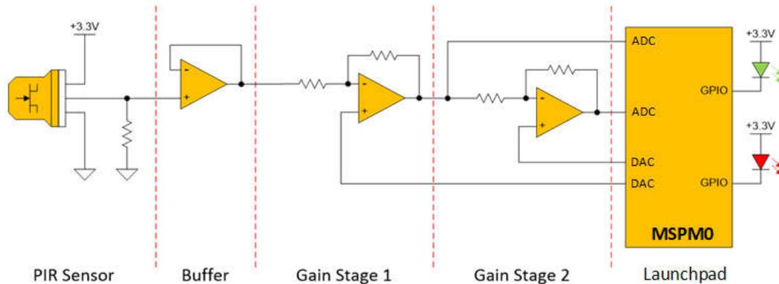
Figure 1-6. Capacitor Free Signal-Chain
