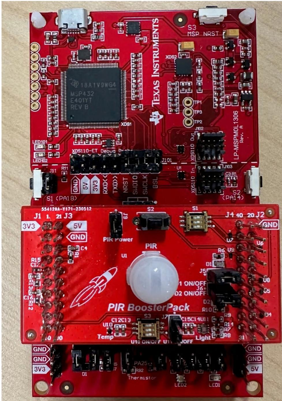
Figure 2-1. MSPM0 Launchpad and PIR Boosterpack
