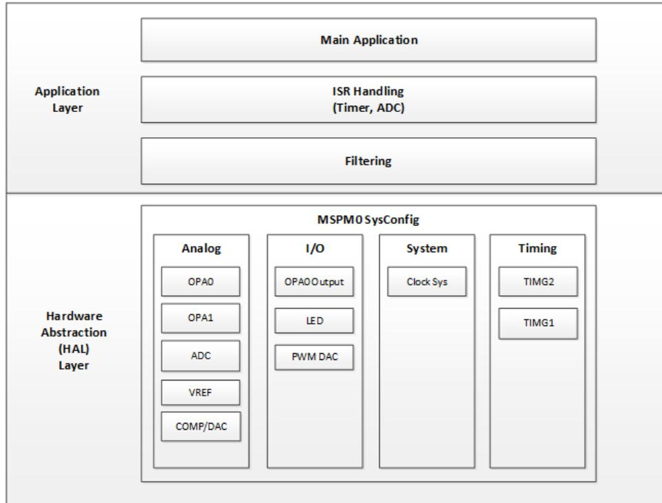
**Figure 3-1. Software Architecture**
