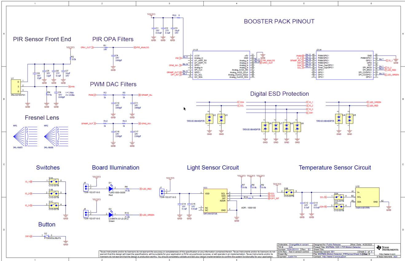
**Figure 2-2. M0L PIR Boosterpack Schematic**
