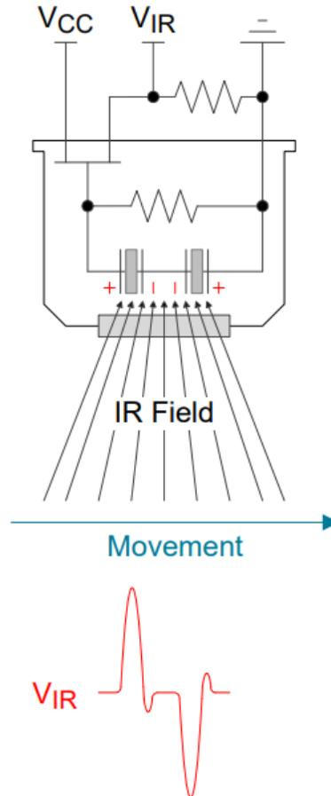
**Figure 1-2. PIR Motion Sensor Illustration**
