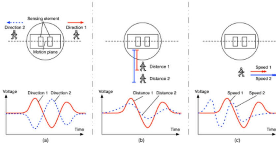
**Figure 1-3. PIR Sensor Output Signal**
