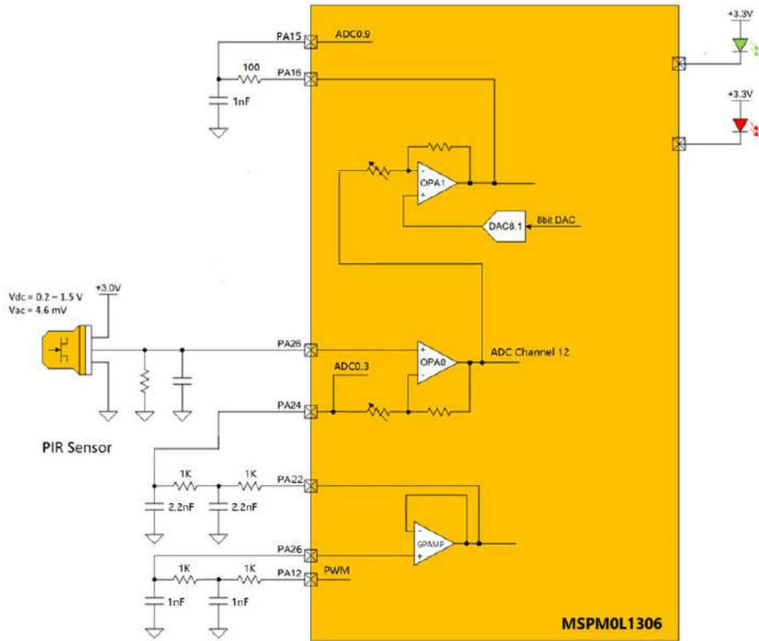
Figure 1-7. PIR Signal-Chain Integrated into MSPM0L1306
