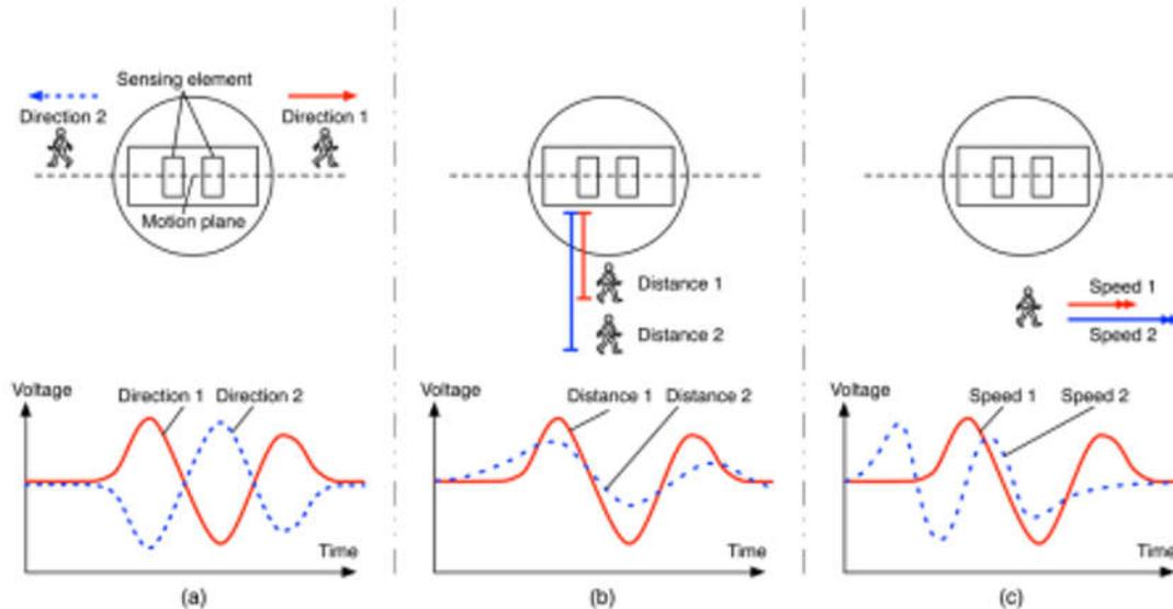
**Figure 1-3. PIR Sensor Output Signal**
