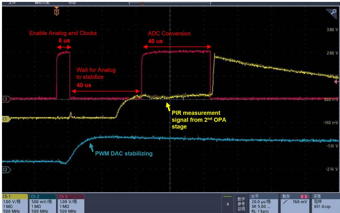
Figure 4-1. Power Profile of MSPM0L13xx PIR Demo Software
