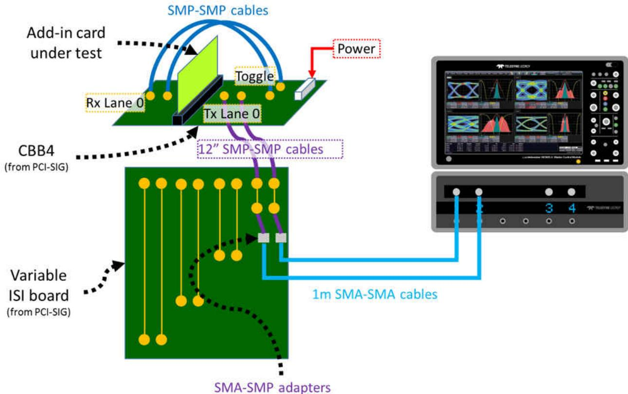
**Figure 2-2. PCI Express® 4.0 TX CBB, AIC Test Setup**
