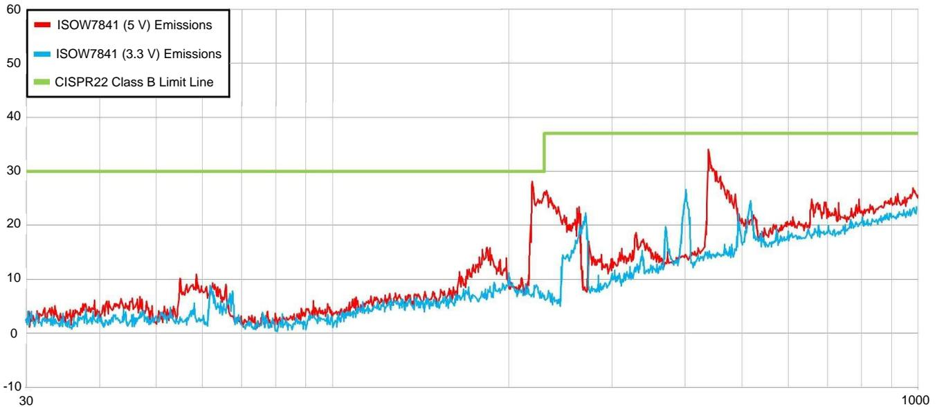
Figure 4. Radiated Emissions of ISOW7841 at 5-V Input vs at 3.3-V Input
