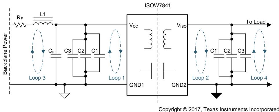
Figure 5. Supply Decoupling Capacitors and Input Ballasting Resistor
