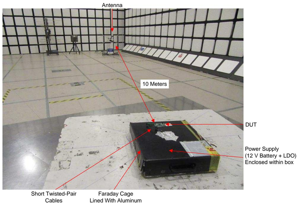
**Figure 14. ISOW7841 Emissions Measurement Setup (CISPR 22)**
