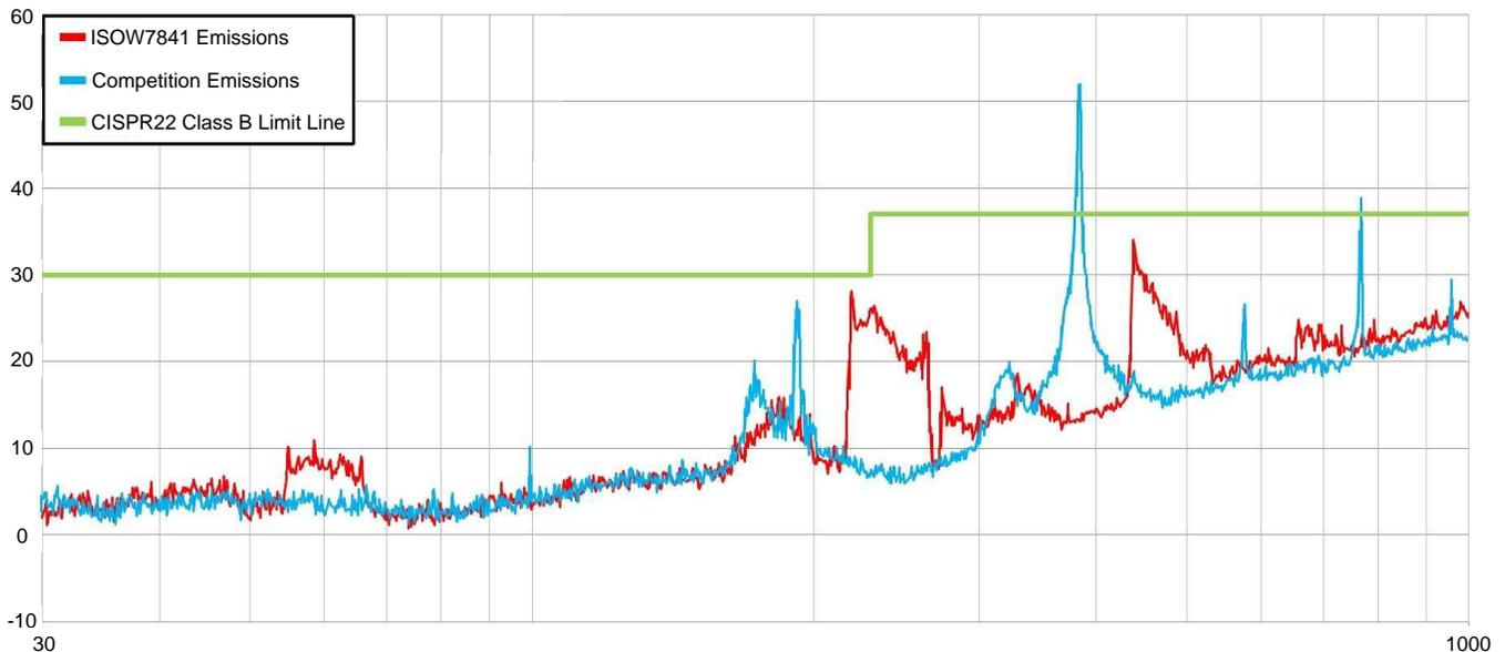
**Figure 3. Radiated Emissions of the ISOW7841 vs a Competitive Device at 5-V Input and 80-mA Load**
