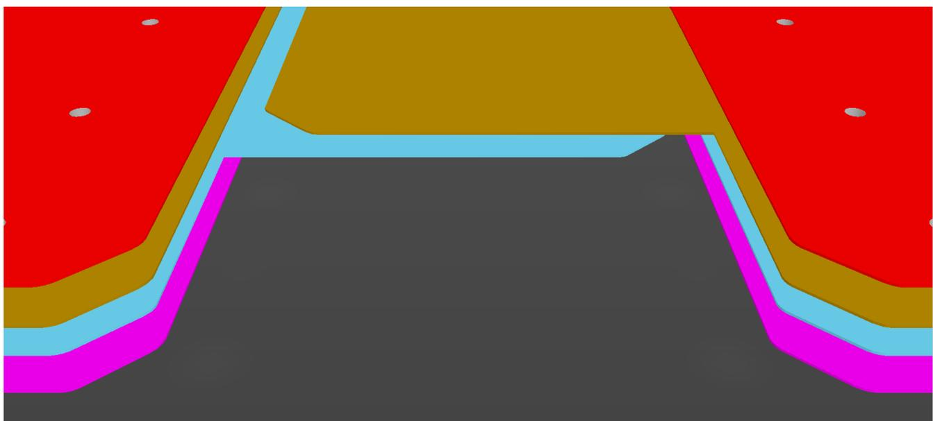
**Figure 11. Triangle Corners Implemented to Enhance High-Voltage Performance**
