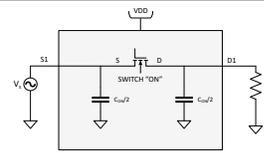
Figure 6-2. Source and Drain On Capacitance
