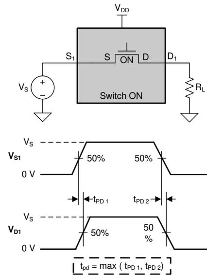
**Figure 7-5. Propagation Delay Through the Switch**
