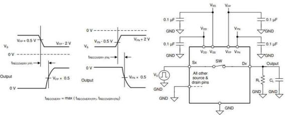
**Figure 7-10. Fault Recovery Time**
