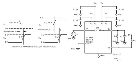
**Figure 7-11. Fault Flag Recovery Time**
