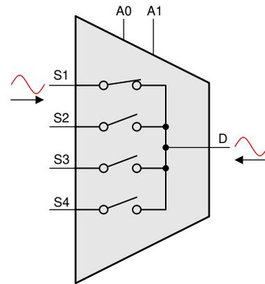
**Figure 3-5. Bidirectional Signal Path**
