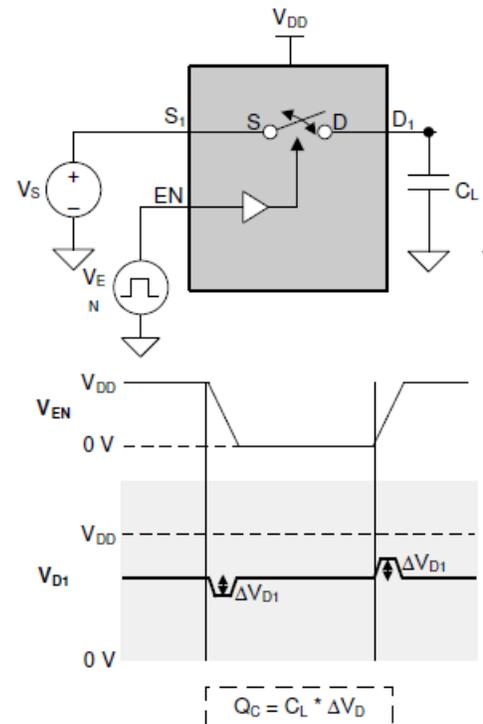
Figure 6-3. Charge Injection
