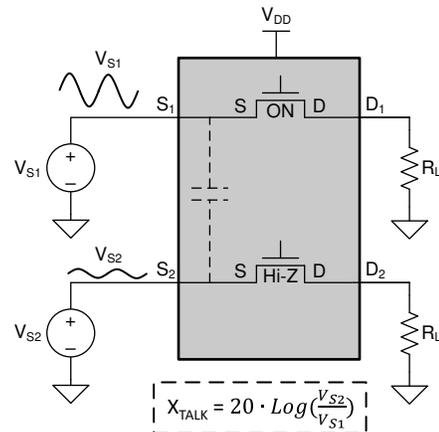
**Figure 6-5. Channel-to-Channel Crosstalk**
