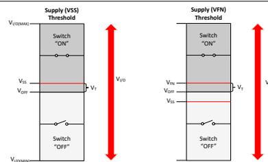
Figure 4-6. Undervoltage Protection
