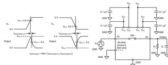
**Figure 7-7. Fault Response Time**
