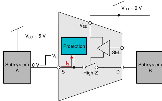
Figure 4-9. Powered-Off Protection
