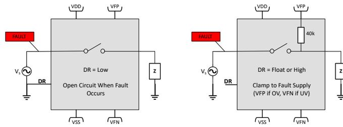
Figure 4-8. Drain Response Output
