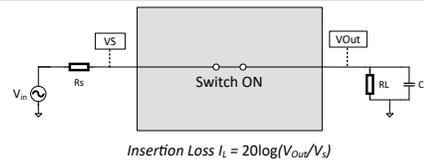
**Figure 6-7. Insertion Loss**
