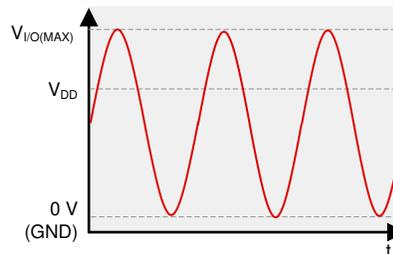
**Figure 3-4. I/O Voltage Beyond Supply**
