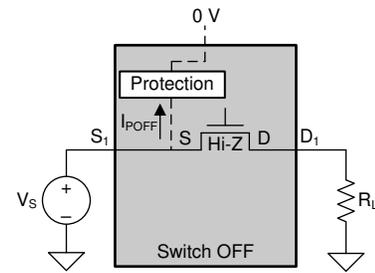
**Figure 5-5. Powered-Off I/O Pin Leakage Current**
