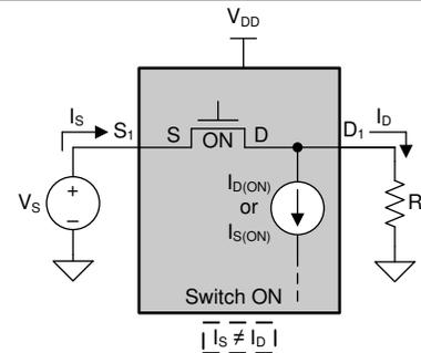
**Figure 5-6. ON Leakage Current**
