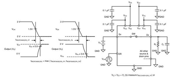
**Figure 7-9. Fault Drain Enable Time**
