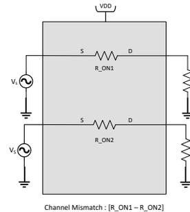
**Figure 5-3.  $\Delta R_{ON}$**
