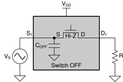
Figure 6-1. Source and Drain Off Capacitance
