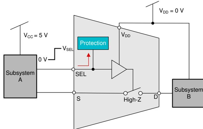
Figure 4-1. Fail-Safe Logic
