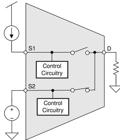
Figure 4-2. Injection Current Control
