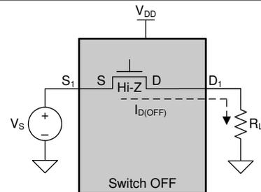
**Figure 5-4. OFF Leakage Current**
