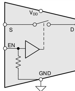
Figure 4-3. Integrated Pull-down Resistor on Logic Pin
