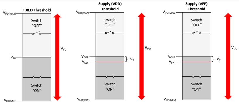
Figure 4-5. Overvoltage Protection
