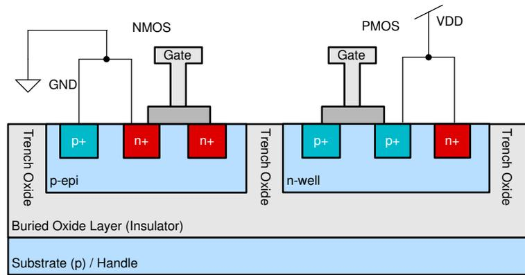
Figure 4-4. Latch-Up Immunity With SOI Process
