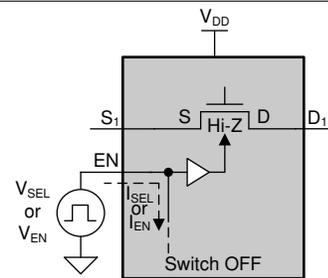
**Figure 5-7. Control Input Leakage**
