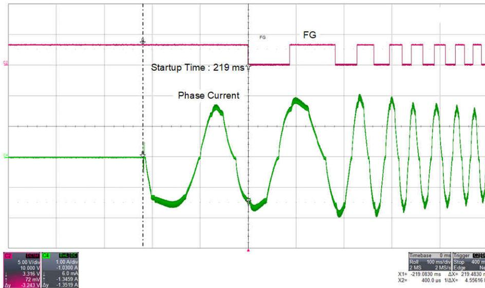
Figure 2-8. Time Taken to Enter Closed Loop in IPD
