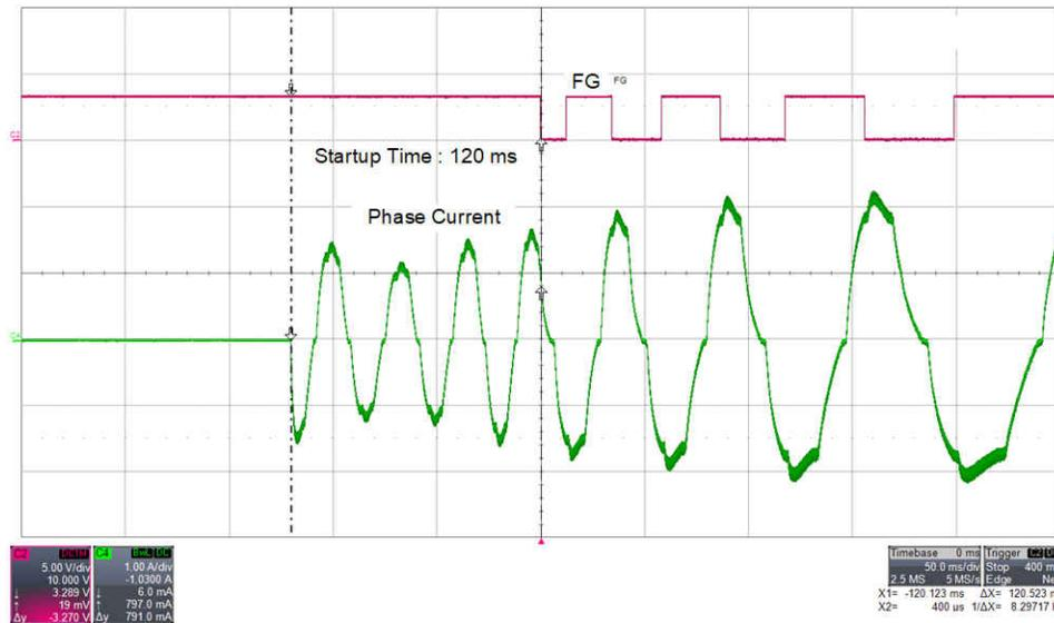
**Figure 2-10. Time Taken to Enter Closed Loop in Slow First Cycle**
