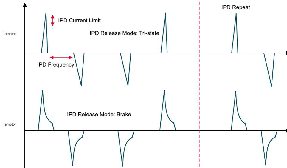
**Figure 2-4. IPD Current Pulses in Tri-State and Brake Mode**
