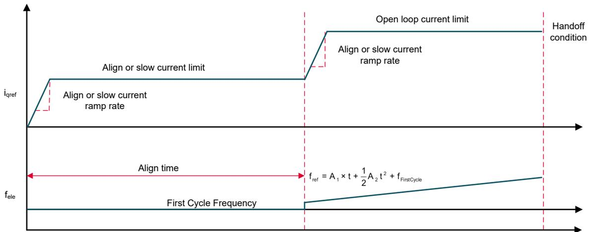
**Figure 2-1. Q-Axis Current and Motor Electrical Frequency During Align**
