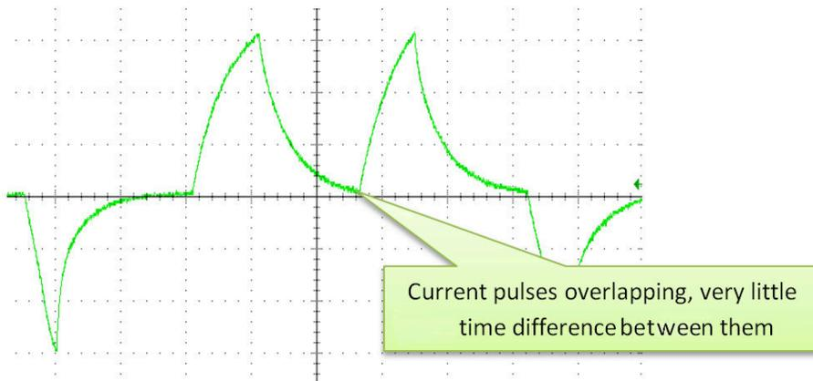
**Figure 2-5. Overlapping IPD Current Pulses**
