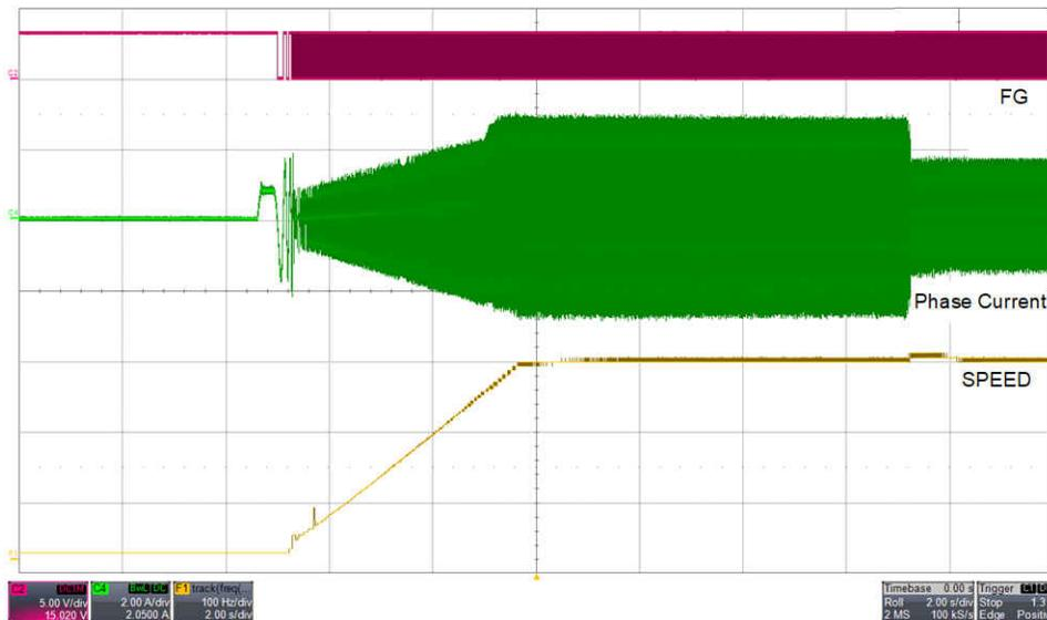
Figure 2-13. FG, Phase Current and Motor Electrical Speed in Hz When the Phase Current Drops From 3A to 1.5A
