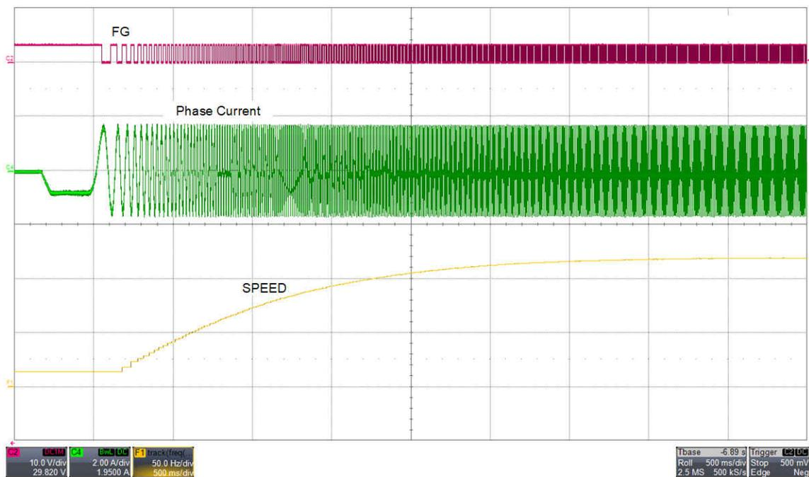
Figure 2-11. FG, Phase Current and Motor Electrical Speed in Hz With Auto Tuned Kp and Ki
