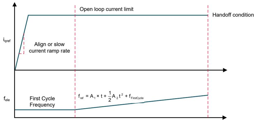
**Figure 2-9. Q-Axis Current and Motor Electrical Frequency During Slow First cycle**
