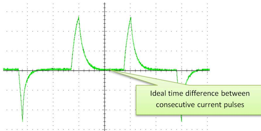
**Figure 2-6. IPD Current Pulses Showing Ideal IPD Clock Frequency**
