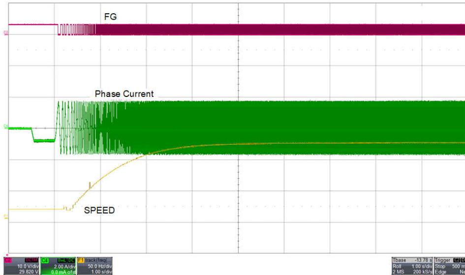
Figure 2-12. FG, Phase Current and Motor Electrical Speed in Hz With Manually Tuned Kp and Ki
