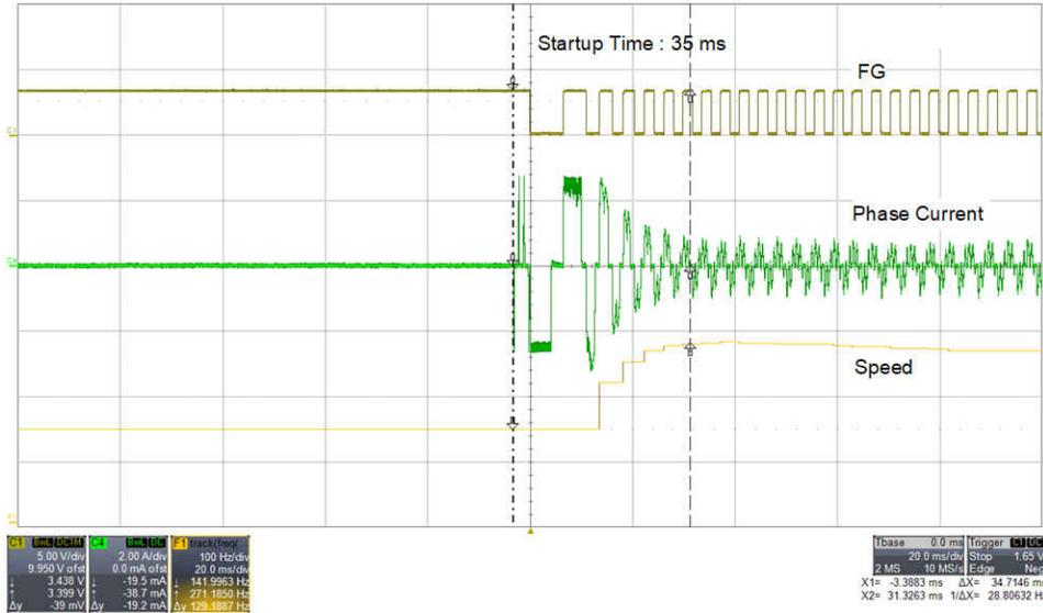
**Figure 2-2. Startup Time Using IPD as Motor Startup Method**
