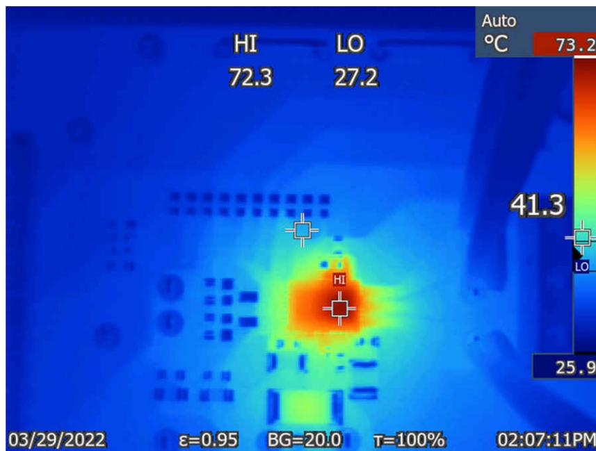
**Figure 2-5. Thermal Image of MCT8316A – Higher Case Temperature**
