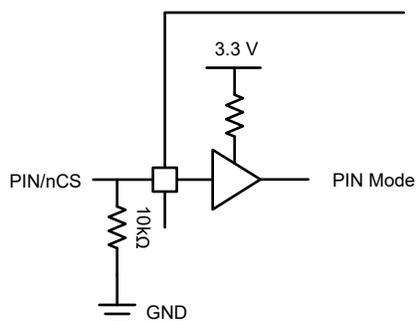
**Figure 1-1. PIN/nCS Configuration for Pin Control**
