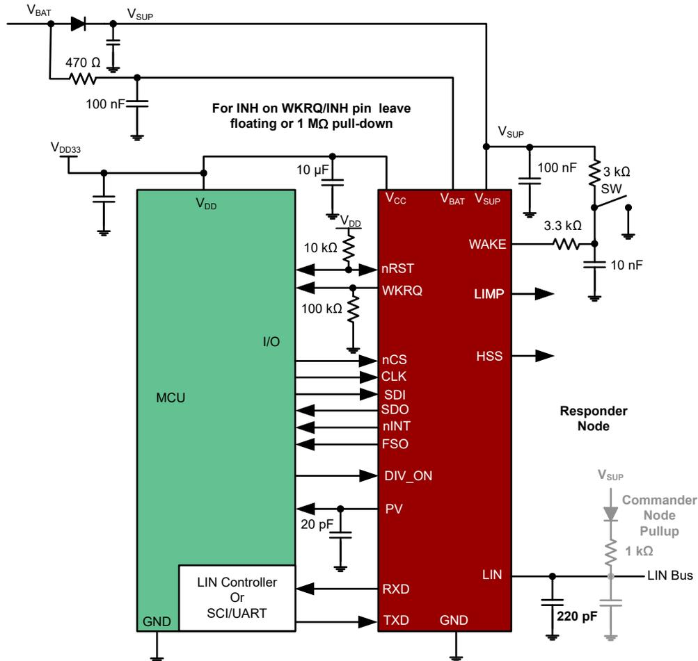
Figure 3-1. Typical Application of TLIN1431-Q1 in SPI Control
