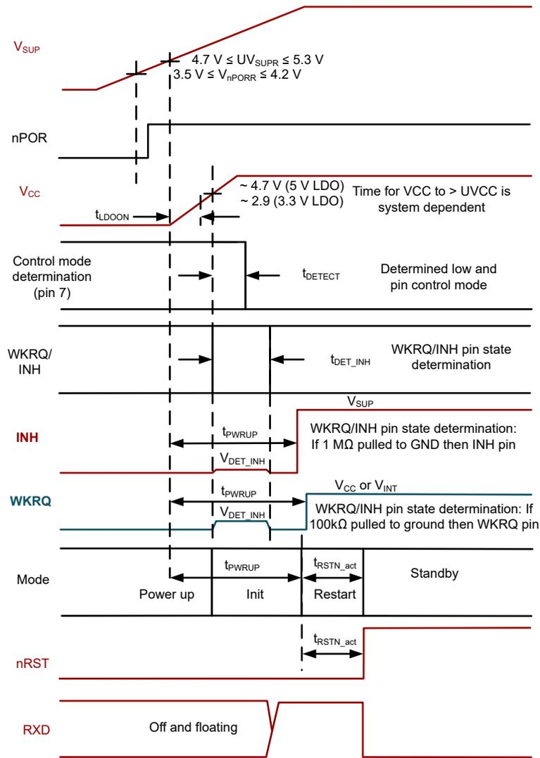
When  $t_{LDOON}$  times out the device checks the status of VCC to determine if a short or over-voltage is present. VCC may or may not have reach regulation
