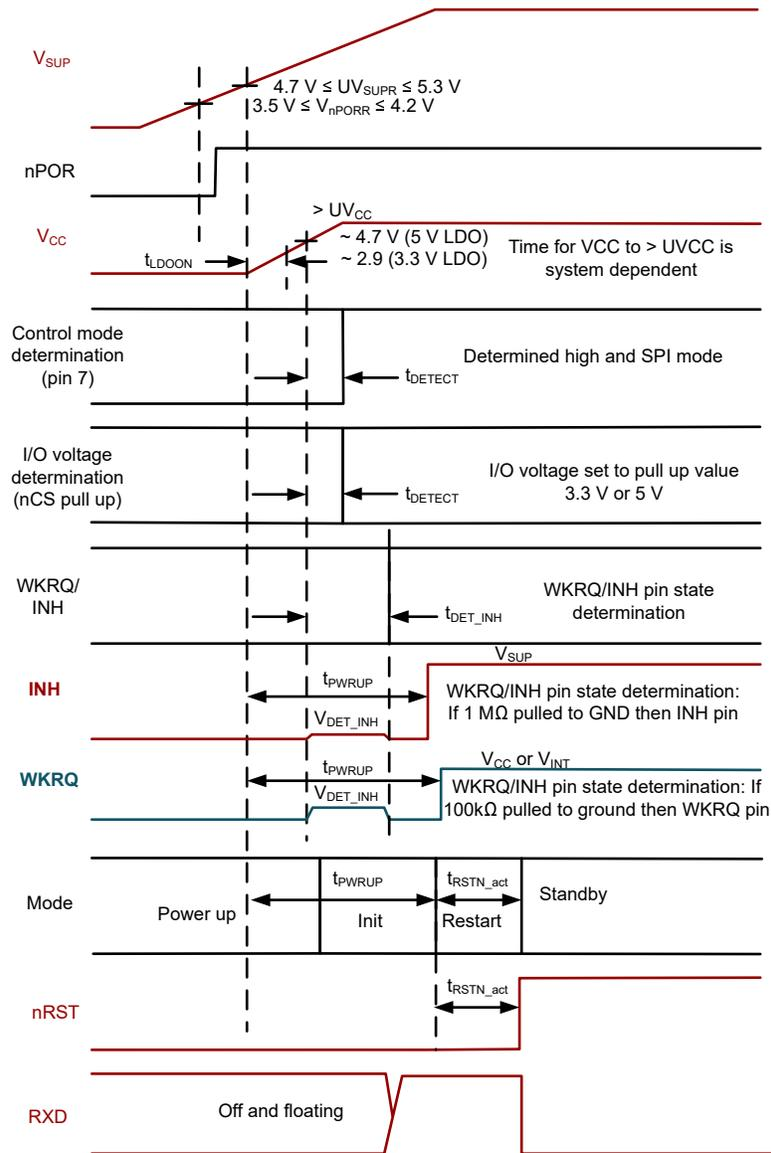
When  $t_{LDOON}$  times out the device checks the status of  $V_{CC}$  to determine if a short or over-voltage is present.  $V_{CC}$  may or may not have reach regulation
