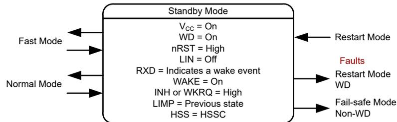
**Figure 2-4. Standby Mode in Pin Control**
