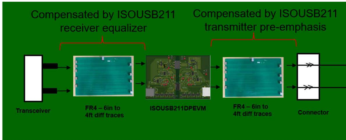
Figure 6-1. Using RXEQ and RX PE for Trace Loss Compensation
