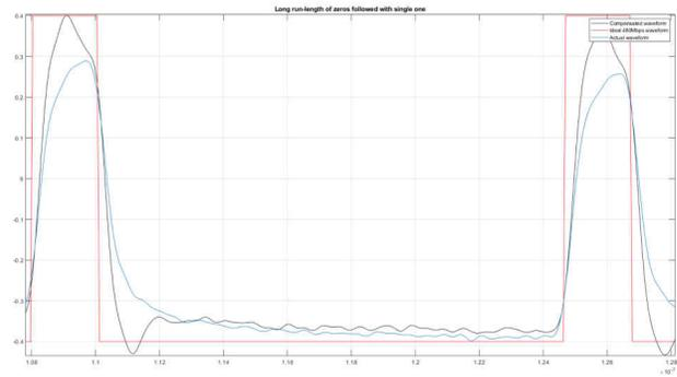
**Figure 2-2. Compensated, Actual, and Ideal Waveforms with Long-Run Length**
