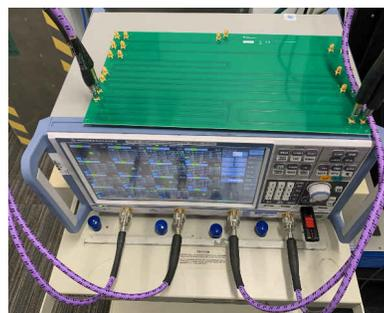
**Figure 1-3. FR4 board with SMA connectors**
