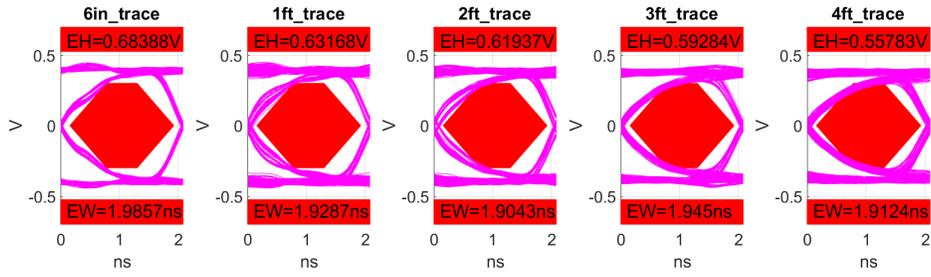
Figure 1-7. Eye-diagrams for 6 inch to 4 feet Traces
