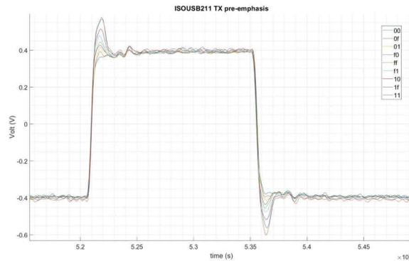
**Figure 2-3. ISOUSB211 Transmitter Pre-emphasis Measurements**
