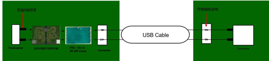
Figure 5-1. Far-end Eye Measurement Setup
