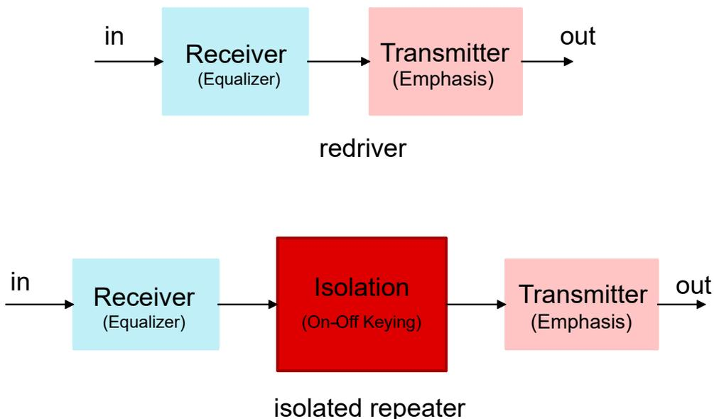
**Figure 1-1. Isolated Repeater vs. Redriver**
