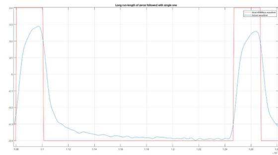
**Figure 1-6. Ideal and Actual USB 2.0 Waveforms with Long Run-length**
