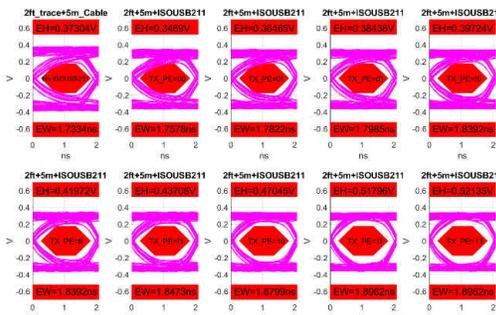
Figure 5-4. FE TX\_PE 2-feet + 5 m
