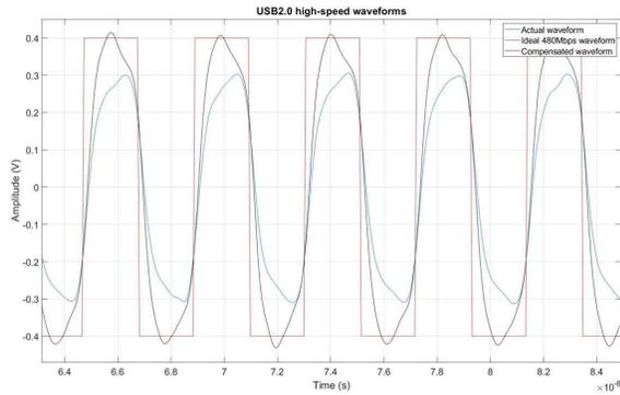
**Figure 2-1. Compensated, Actual, and Ideal Waveforms**
