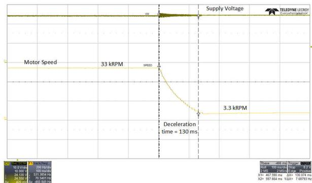
**Figure 6. Fast Deceleration with a CPAP Motor using MCT8329A**
