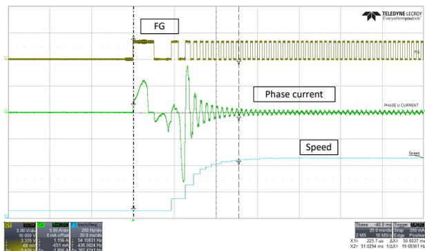
**Figure 7. Fast Acceleration with a Fuel Pump Motor using MCT8329A**
