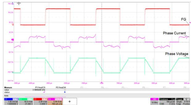
Figure 1. Motor Speed More Than 3 kHz with MCT8329A
