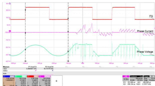
Figure 2. On-The-Fly Catch at 3 kHz Initial Speed using MCT8329A
