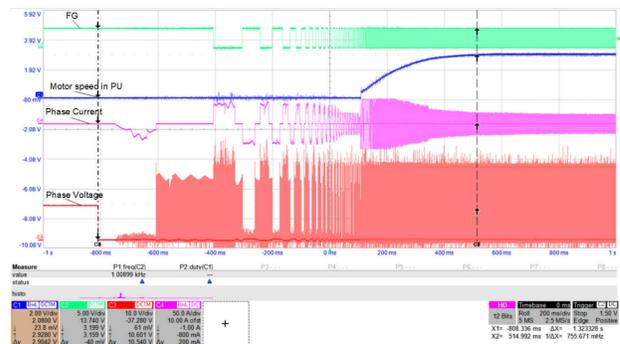
**Figure 8. Fast Acceleration with a Vacuum Cleaner Motor using MCT8329A**
