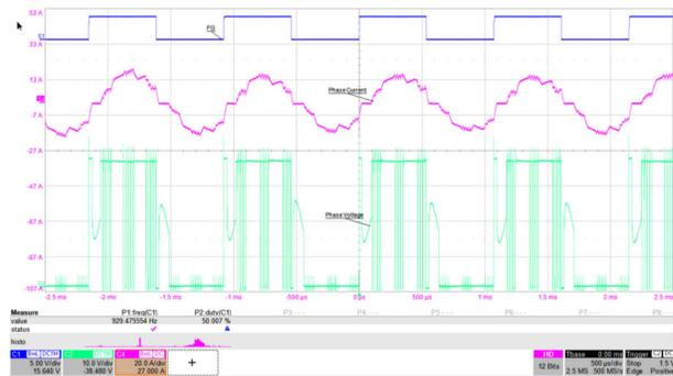
**Figure 5. High Speed Operation of a Vacuum Cleaner Motor with 150° Modulation**
