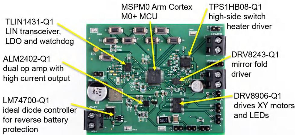
**Figure 2. Example Implementation of Side Mirror Module Design**
