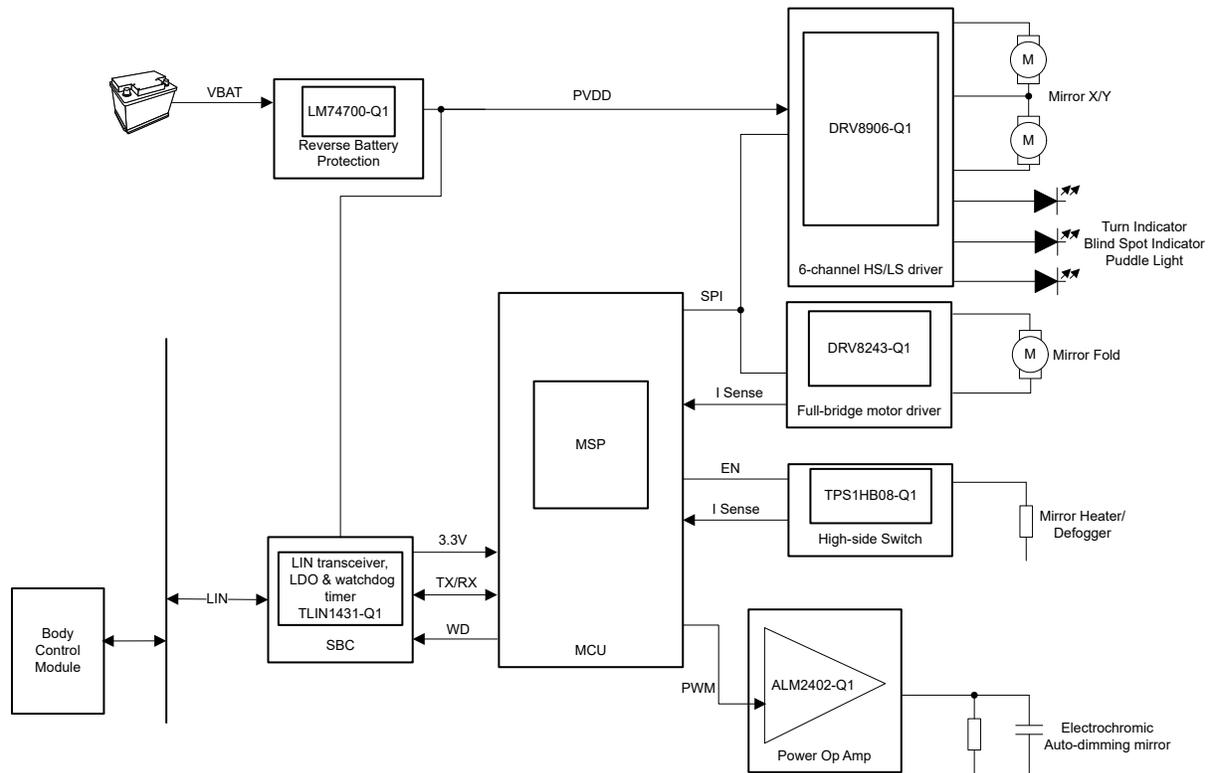
**Figure 1. Block Diagram of Typical Side Mirror**
