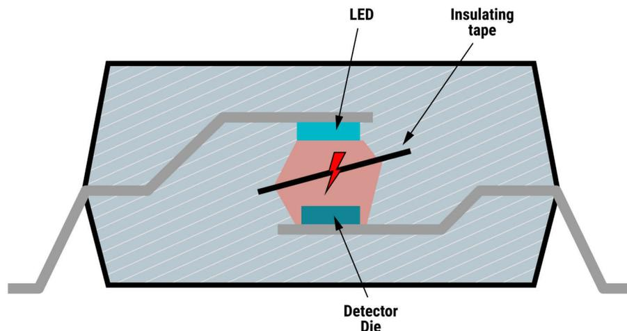
**Figure 1-1. Cross-Section of an Opto-Coupler**
