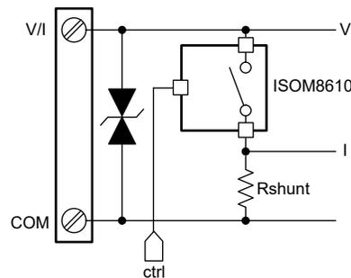
Figure 2-4. ISOM8610 for Switching Burden Resistor in Universal Analog Input Module
