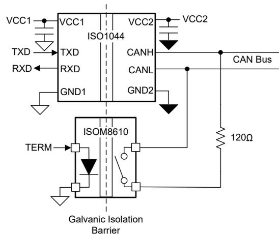
Figure 2-1. ISOM8610 for Software Controllable Switchable Termination on CAN Bus
