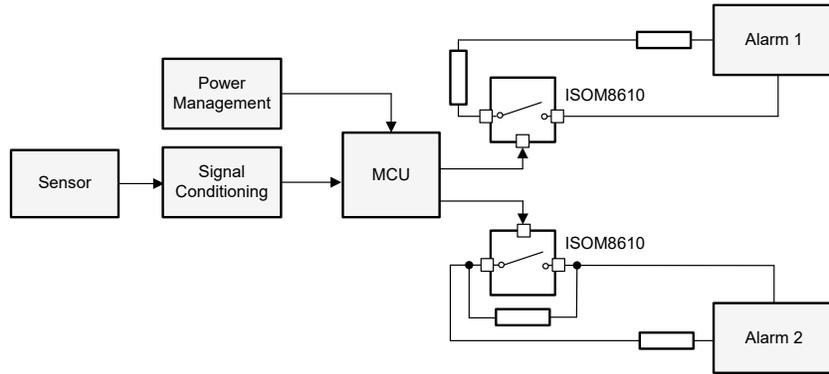
**Figure 2-5. ISOM8610 for Switch Outputs in Intrusion Detection Systems**
