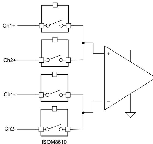
Figure 2-3. ISOM8610 for Channel to Channel Isolated Analog Voltage Input Module
