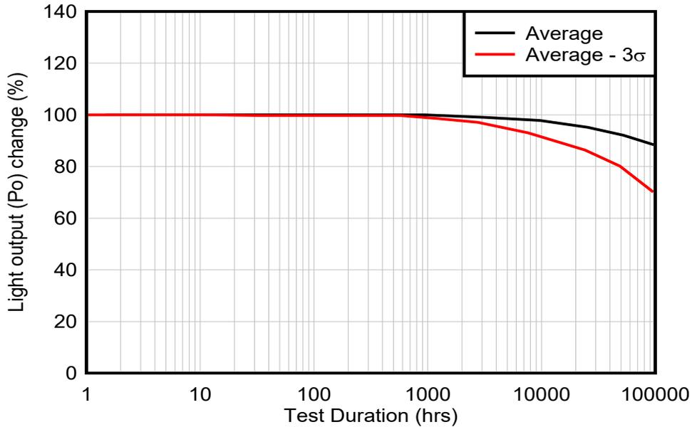
**Figure 1-2. LED Deration Over Lifetime Usage (Representational)**
