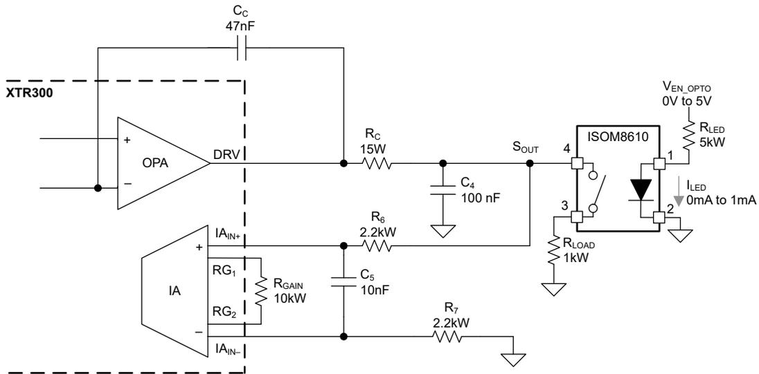
Figure 2-2. ISOM8610 for Analog Voltage/Current Driver Output Isolation
