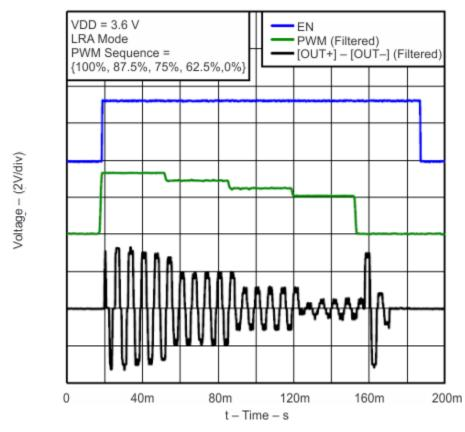
Figure 1-1. LRA Auto-Resonance Detection
