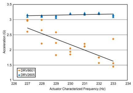
Figure 3-2. Acceleration Performance of the DRV2605 versus DRV8601
