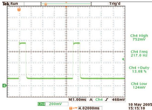
**Figure 2. GSM Load Profile Across a 0.5-Ω Resistor**
