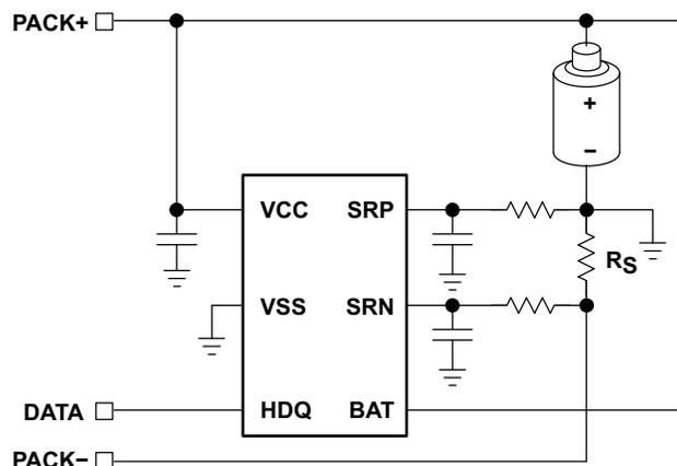
**Figure 1. Simplified Gas Gauge Circuit**
