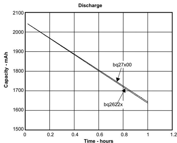
**Figure 3. Capacity Measurement During Discharge**
