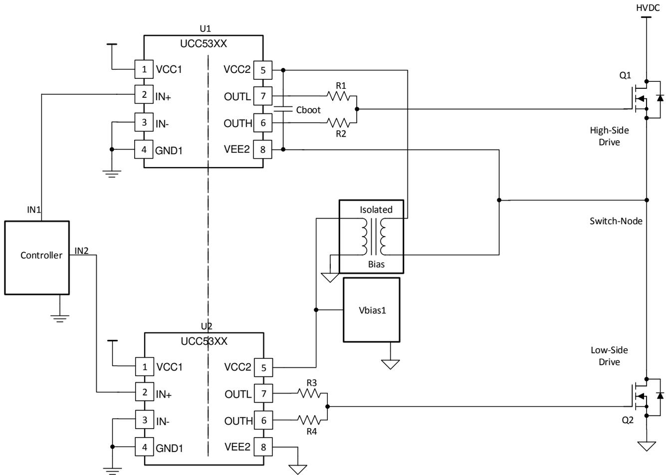
**Figure 2-5. Isolated Drivers Using Isolated Bias Supply**
