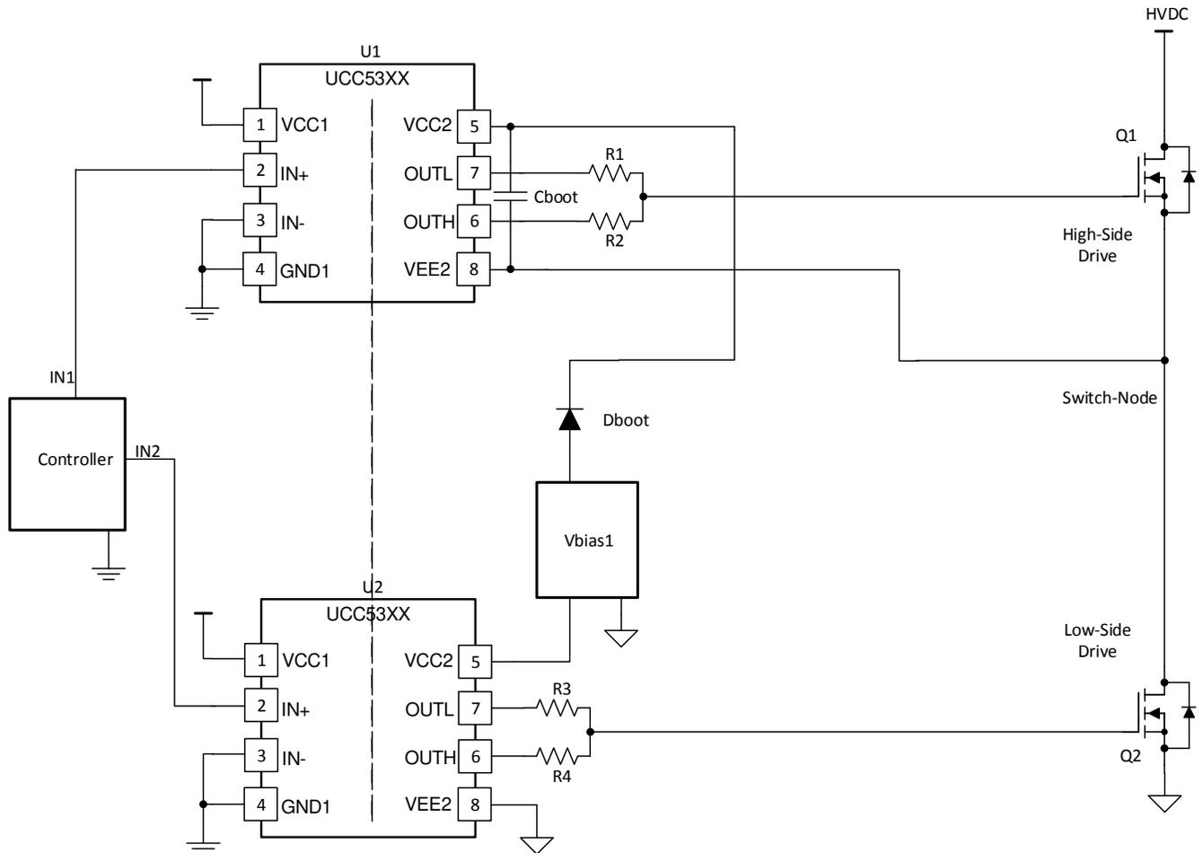
Figure 2-4. Isolated Drivers Using High-Side Bootstrap Circuit
