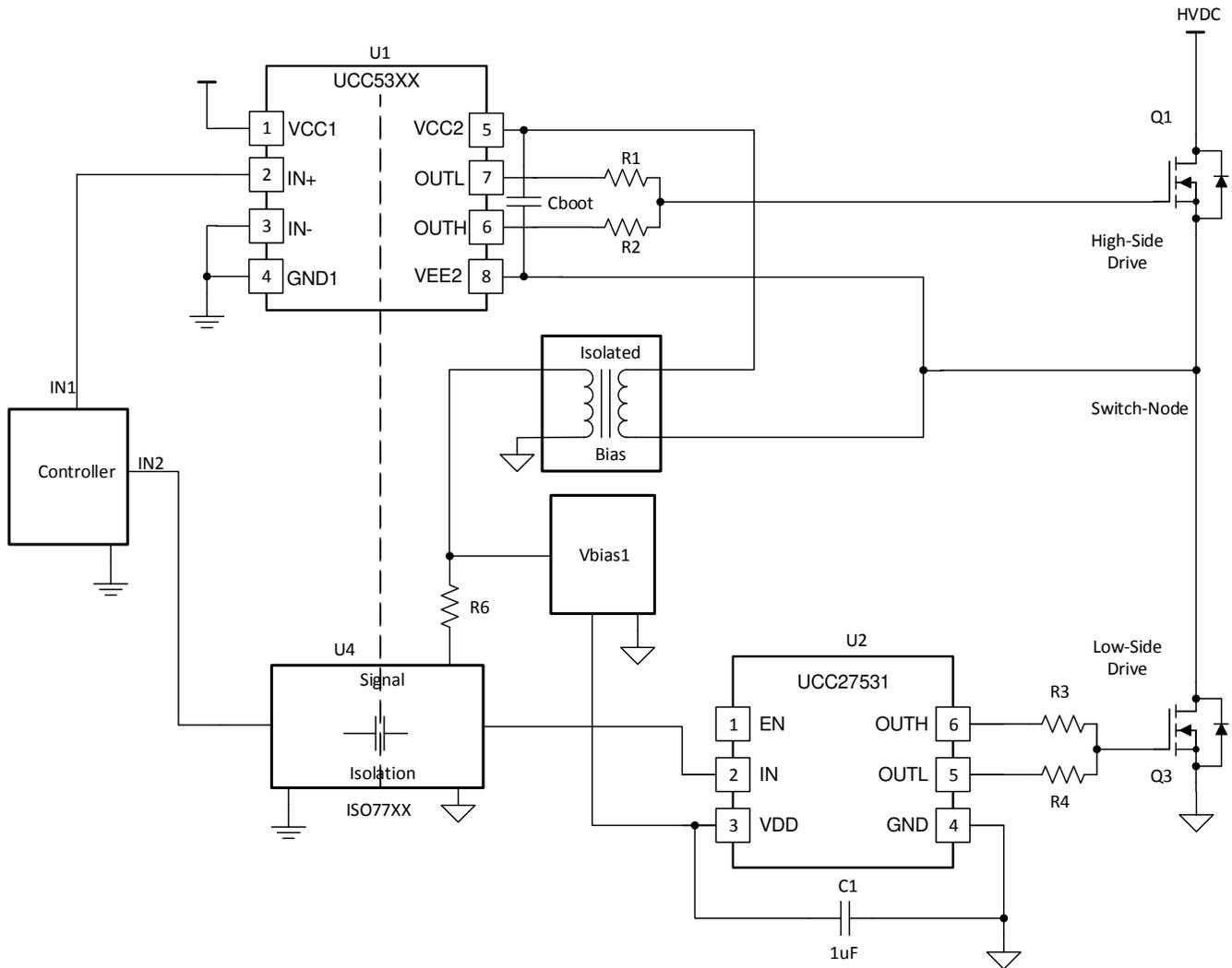
**Figure 2-3. High-Side Isolated Driver and Bias Supply**
