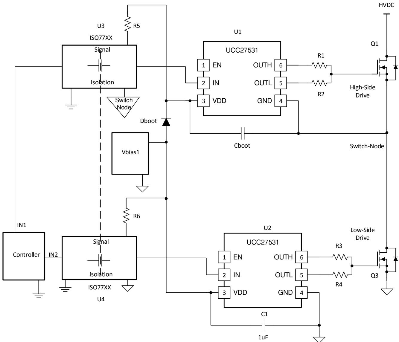
**Figure 2-2. High-Side Bootstrap Circuit Using Capacitor-Based Signal Isolation**
