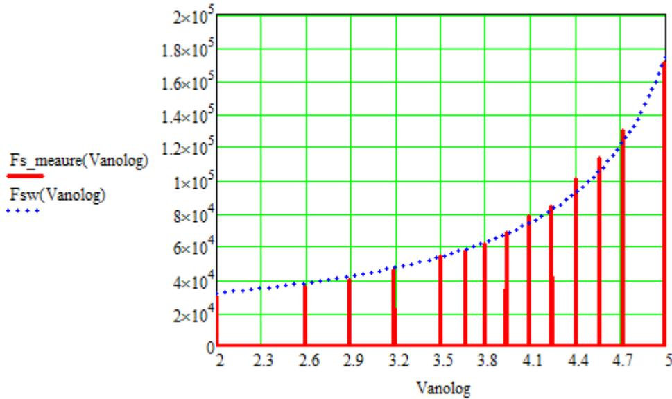
**Figure 15. Operation Frequency Curve—Comparison Between Measurement and Calculation**
