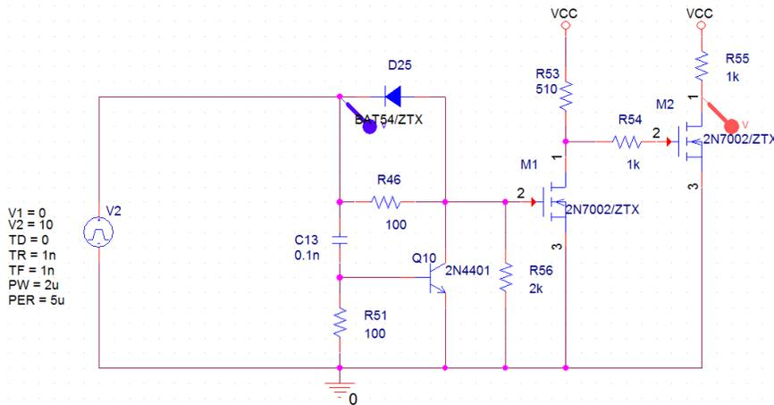
**Figure 12. Circuit to Improve Analog Dimming Performance**
