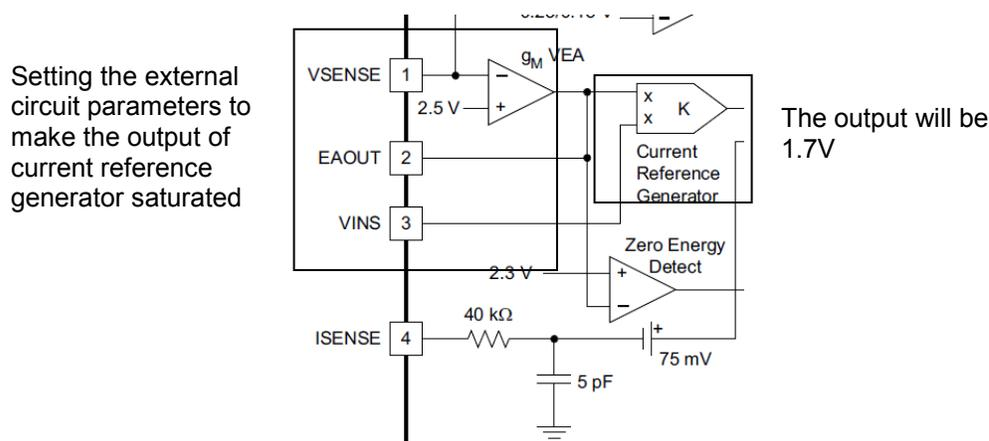
Figure 2. Internal 1.7-V Creating Function for the UCC28810/11 Device
