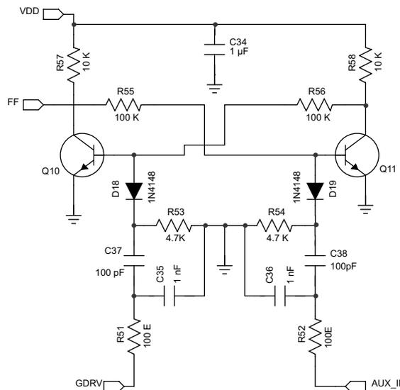
(Circuit used in only-primary-side output current regulation scheme.)
