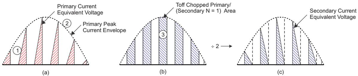
Figure 9. Primary-Side Output Current Regulation Logic
