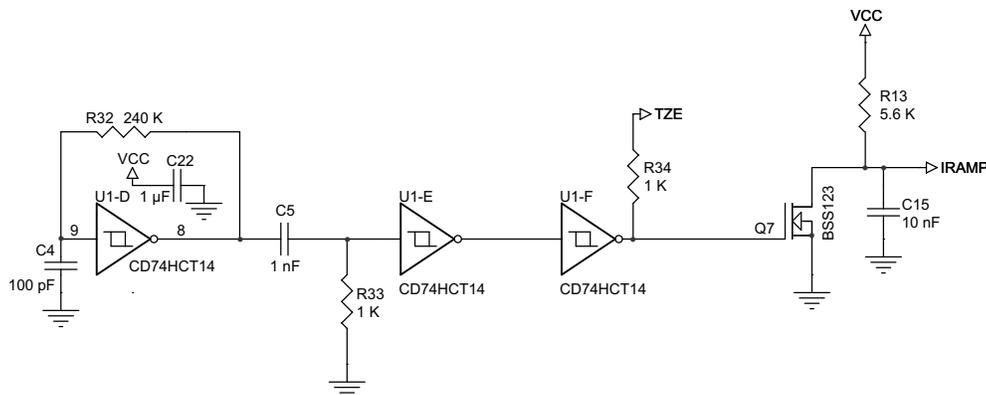
Figure 6. Switching Oscillator
