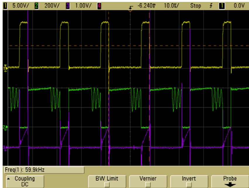
Ch1: Primary-Side FET Gate Drive, Ch2: Primary-Side FET Drain Waveform,
