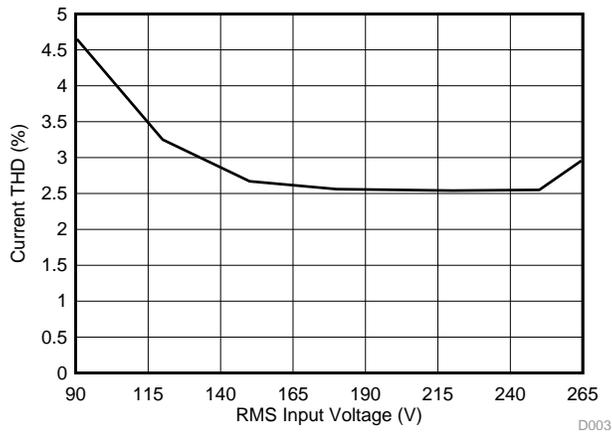
Figure 15. Variation of Current THD with Input Voltage
