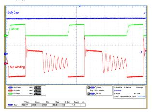
Figure 3. Waveforms Needed to Distinguish Input UVLO Issue
