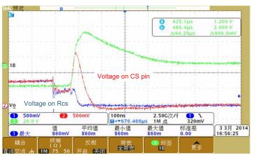
Figure 6. OCP Caused by the Noise
