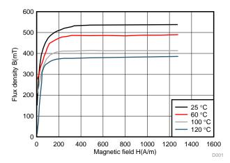
Figure 8. B-H Temperature Characteristics of the TDK PC95
