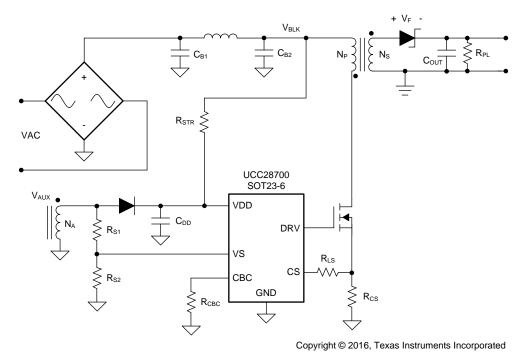
Figure 1. Simplified Typical TI PSR Flyback Application
