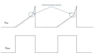
Figure 7. OCP Protection Caused by Transformer Saturation
