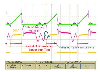
Figure 11. Long LC Resonant Period Causes Missing Valley Switching
