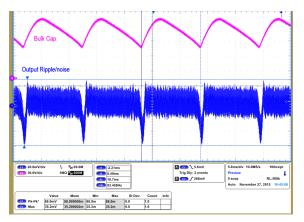
Figure 9. Line Frequency Ripple in Output Voltage
