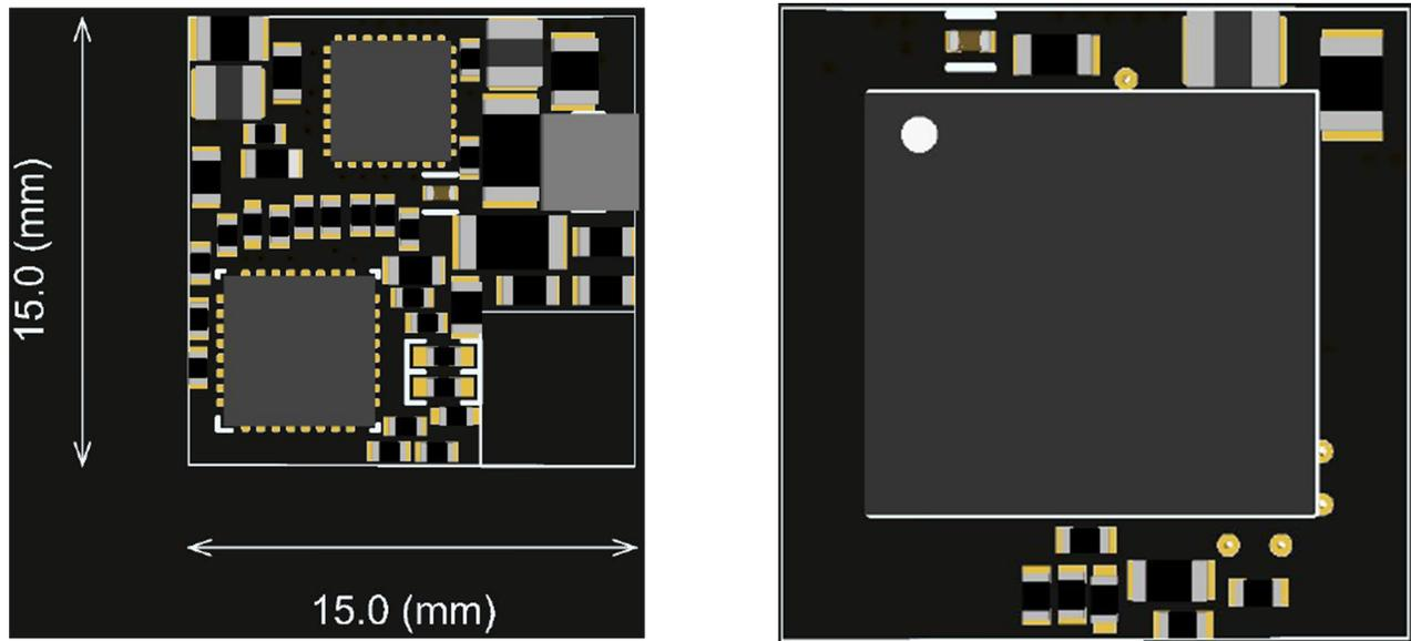
Figure 7. Layout Example – Double Sided
