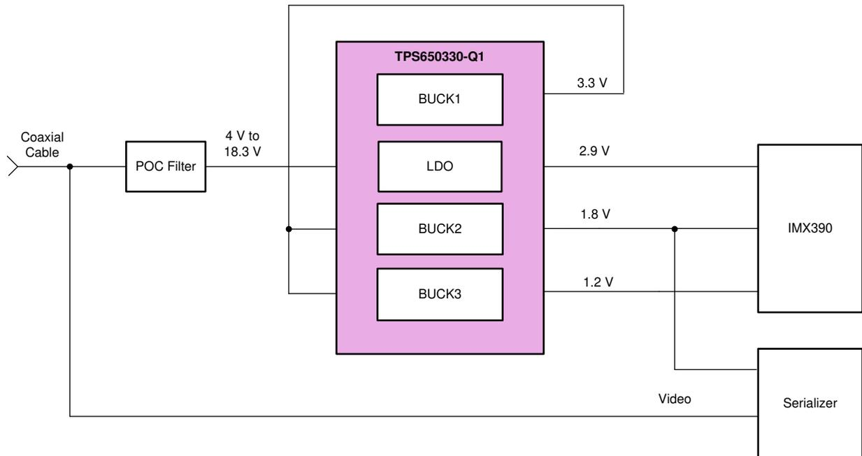
**Figure 1. Sony® IMX390™ Powered by the TPS650330-Q1 Power Management IC (Texas Instruments Reference Design [TIDA-020003](#))**
