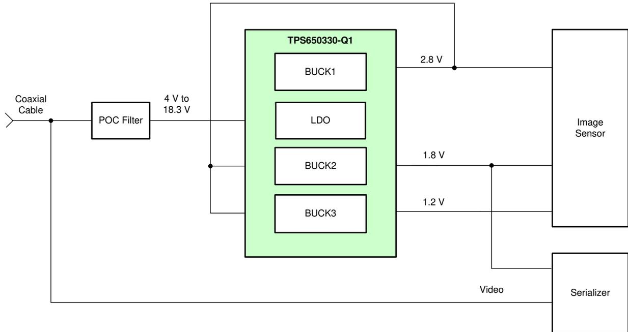
**Figure 9. Using a DCDC Converter to Power the Analog Rail.**
