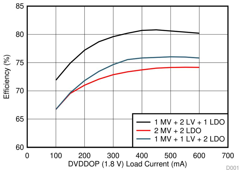
**Figure 4. Overall System Level Efficiency Comparison Graph <sup>(9)</sup>**
