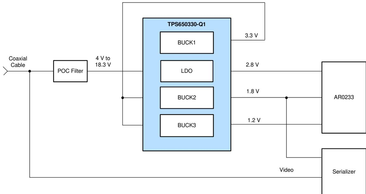
**Figure 2. Aptina® AR0233™ Powered by the TPS650330-Q1 Power Management IC (Texas Instruments Reference Design [TIDA-050035](#))**
