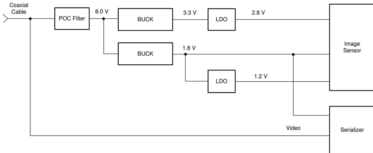
**Figure 5. 2 MV + 2 LDO Configuration**
