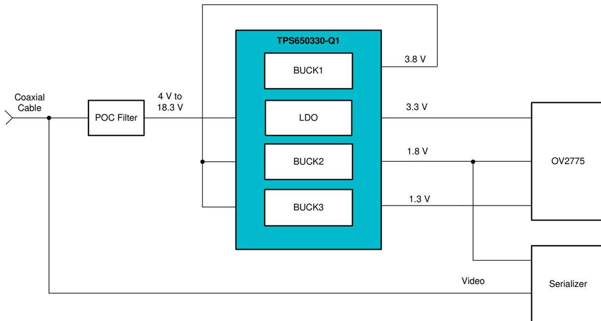
**Figure 3. Omnivision® OV2775™ Powered by the TPS650330-Q1 Power Management IC**
