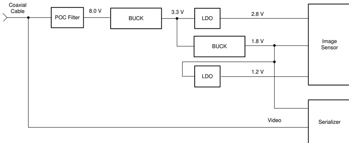
**Figure 6. 1 MV + 1 LV + 2 LDO Configuration**
