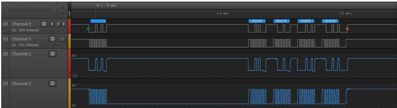
**Figure A-6. Current Write From the Gauge to the Charger in Broadcast Mode**
