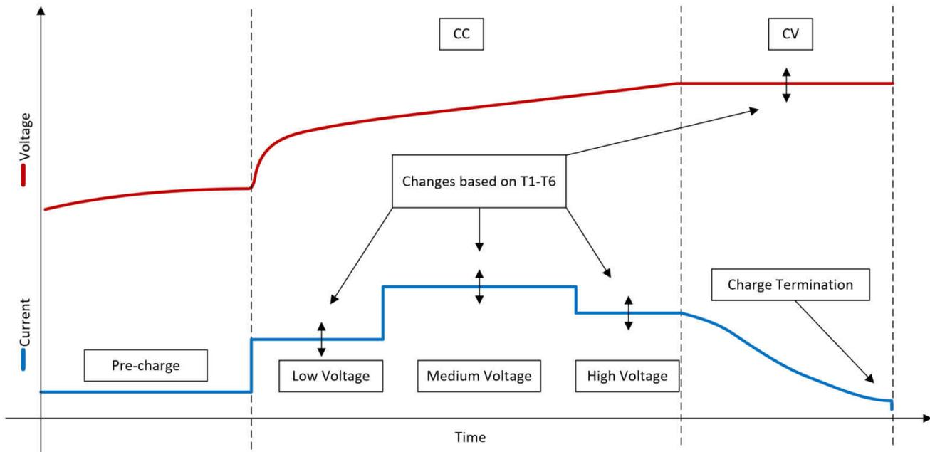
**Figure 2-1. Charging Profile Using Advanced Charging Algorithm**
