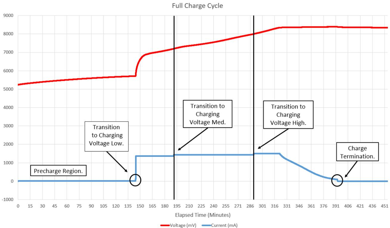
**Figure 4-2. Full Charge Cycle Using SMBus SBS**
