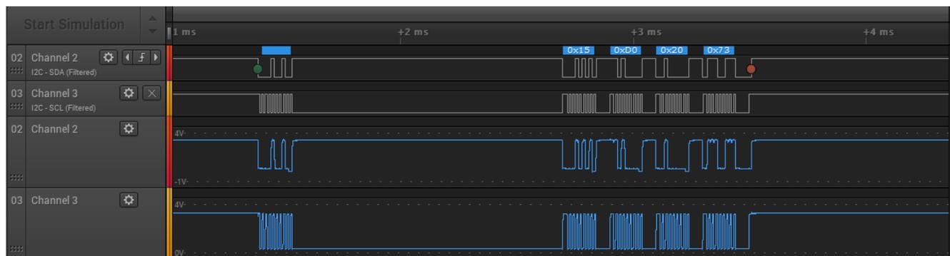
Figure A-5. Voltage Write From Gauge to the Charger in Broadcast Mode
