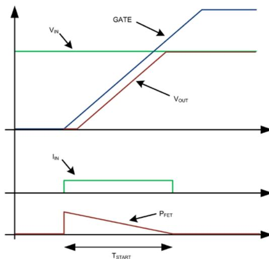
**Figure 7. Start Up With Output  $dv/dt$  Control**
