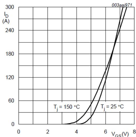
**Figure 12. Transfer Characteristics (PSMN4R8-100BSE)<sup>4</sup>**
