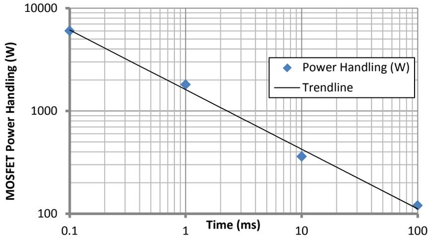
Figure 10. SOA vs Time for  $V_{DS} = 60\text{ V}$  (PSMN4R8-100BSE)<sup>4</sup>
