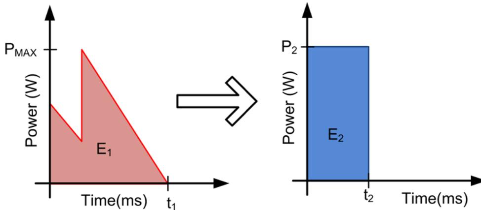
Figure 11. Approximating FET stress for Non-square pulses
