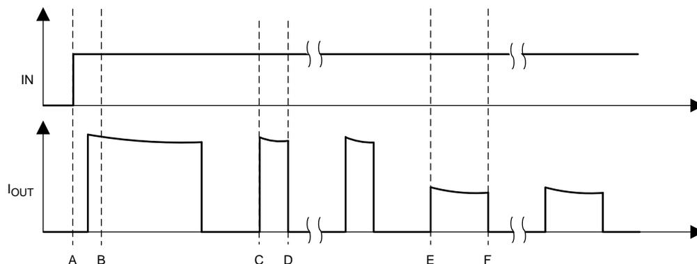
**Figure 4. Timing Diagram of Hot Repetitive Short Circuit**
