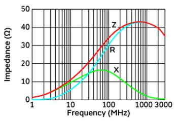
Figure 13. Impedance VS. Frequency Characteristics (BLM21PG300SN1)
