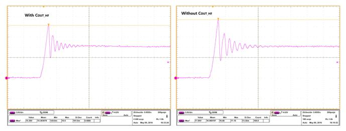
Figure 5. SW Voltage Spike With and Without  $C_{OUT\_HF}$
