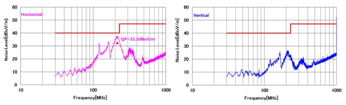
Figure 15. Radiated EMI Result ( $V_{IN}$  = 3.3V, VO = 9 V /  $I_{O}$  = 2A)
