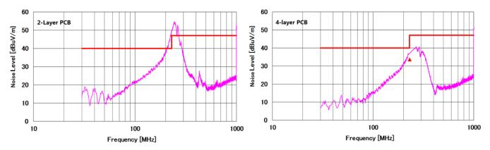
Figure 7. Radiated EMI Result of a 2-Layer PCB and a 4-Layer PCB
