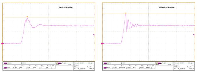
Figure 9. SW Voltage Comparison With and Without RC Snubber
