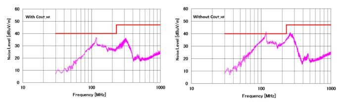
Figure 6. Radiated EMI Result With and Without Cout HF
