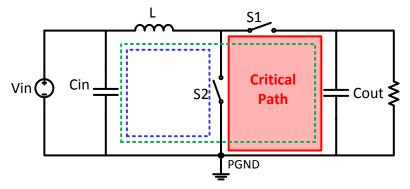
Figure 1. Critical Current Path of Boost Converter
