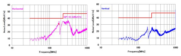
Figure 16. Radiated EMI Result ( $V_{IN}$  = 3.3V, VO = 12V /  $I_o$  = 1.5 A)
