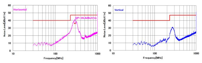
Figure 14. Radiated EMI Result (V<sub>IN</sub> = 3.3 V, VO = 5V / I<sub>o</sub> = 3A)
