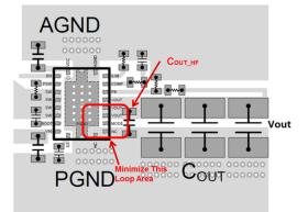
Figure 3. TPS61088 Critical Path Layout Example
