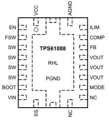
Figure 2. TPS61088 Pin Configuration
