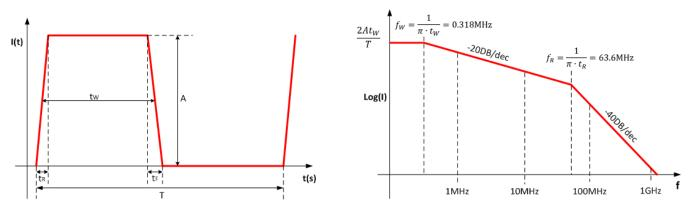
Figure 10. Harmonic Content of a Pulsed Current Waveform
