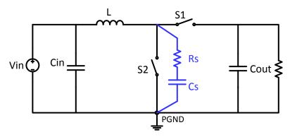
Figure 8. Placement of RC Snubber
