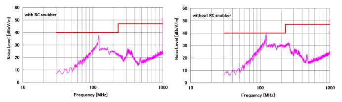
Figure 11. Radiated EMI Result With and Without RC Snubber
