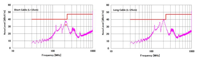
Figure 12. Radiated EMI Result with Different Input Cable Length
