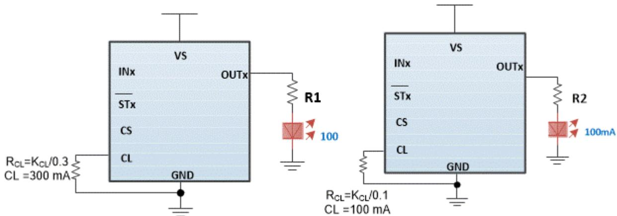
**Figure 5-4. Driving LED in Constant Output Voltage and Constant Current Mode**
