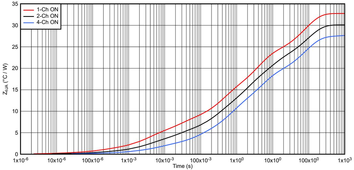
Figure 6-7. TPS4H160-Q1 Transient Thermal Impedance  $Z_{\Theta JA}$
