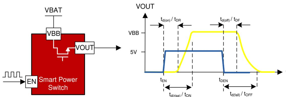
**Figure 2-4. Smart High Side Switching Waveform**
