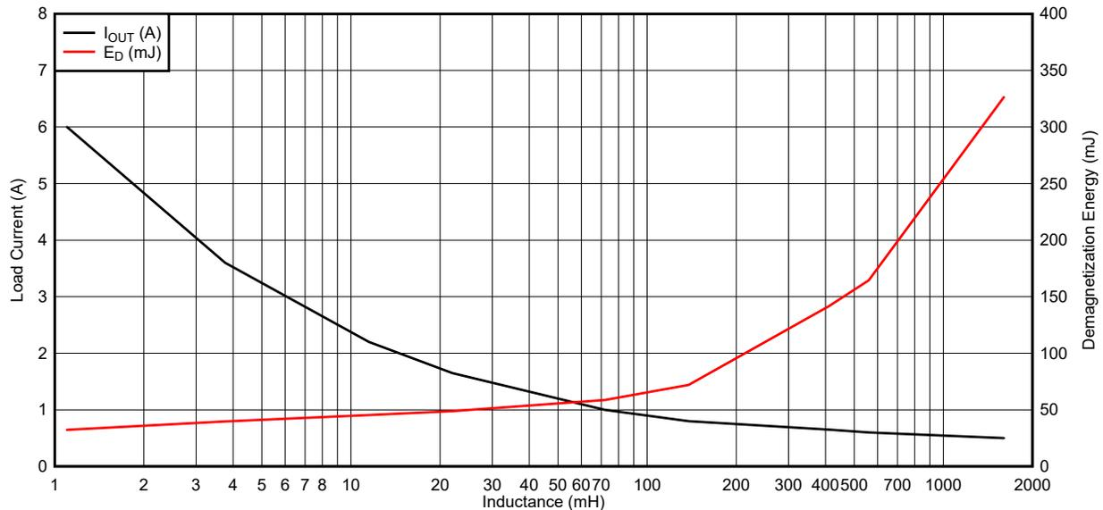
Figure 4-5. TPS4H160-Q1 Demagnetization Capability
