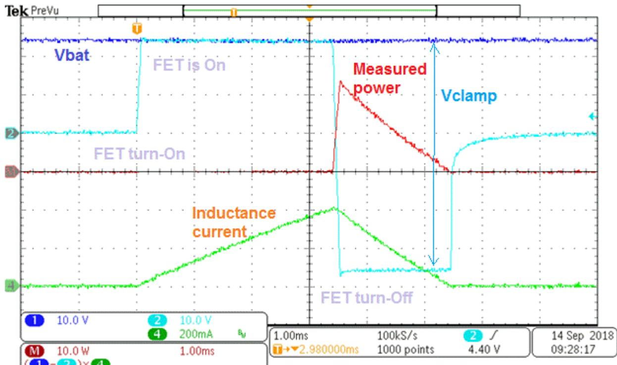
Figure 4-4. Demagnetization Energy During Inductive Turn-Off
