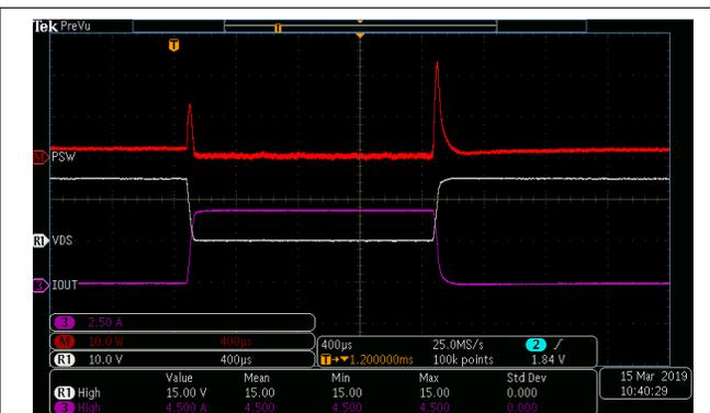
Figure 2-7. Measured Switching Losses Waveform
