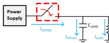
**Figure 3-3. Capacitive Load Charging Diagram**
