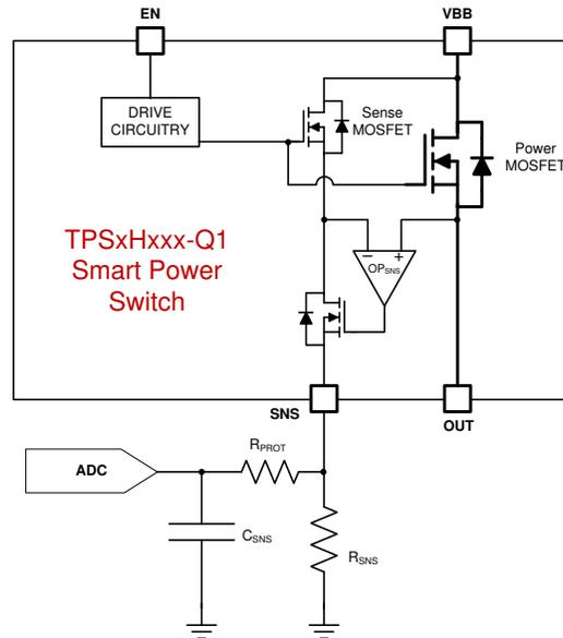
Figure 2-3. TPSxHxxx Current Sense Circuit
