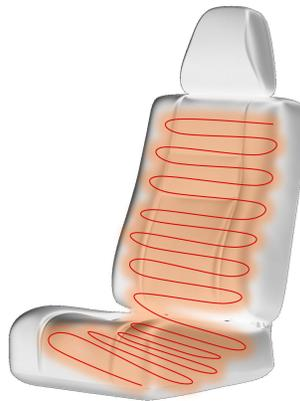
**Figure 2-1. Seat Heater Resistive Load Application**
