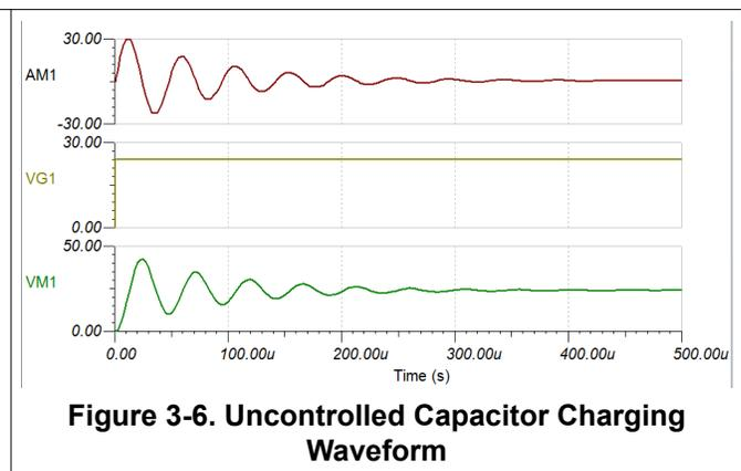
Figure 3-6 shows that an uncontrolled  $dV/dT$  leads to an inrush current that reaches nearly 30A with severe ringing. Without current limiting this is the quickest way to charge the capacitor, however for many systems this sort of inrush current is not acceptable and cannot be supported by the input power rail.
