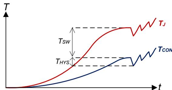
**Figure 3-17. Thermal Cycling due to relative thermal shutdown mechanism**
