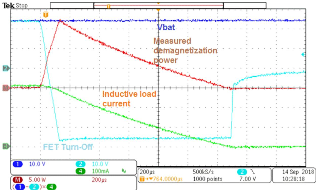
Figure 4-6. Load 1 Measured Demagnetization Energy
