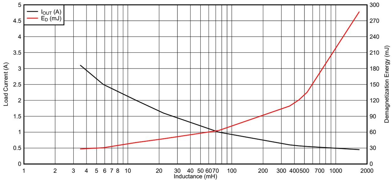
Figure 6-16. TPS1H200-Q1 Demagnetization Energy Capability
