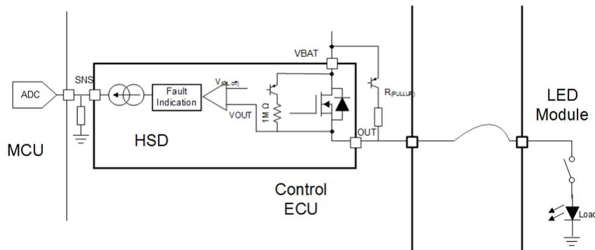
Figure 5-3. Open Load Detection Schematic
