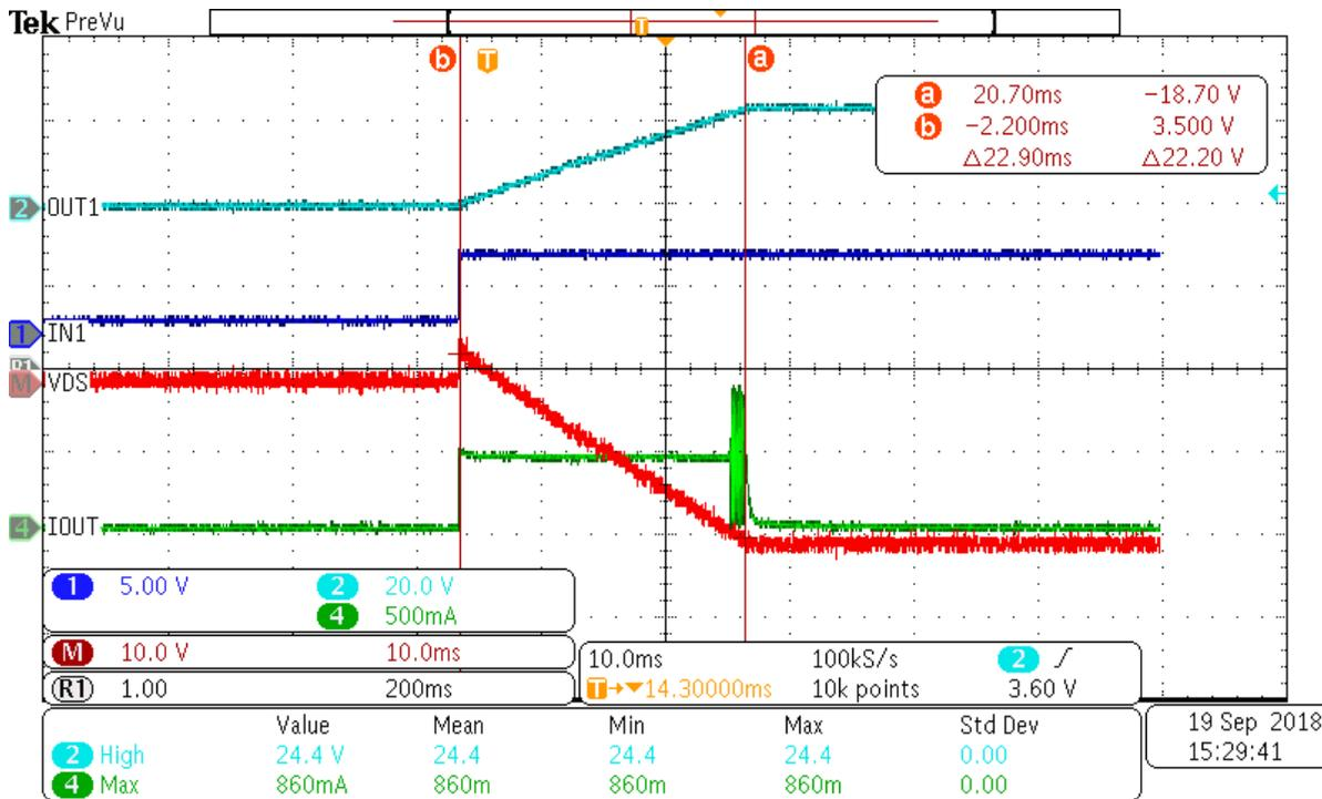
**Figure 3-11.  $V_{DS}$  While Charging Capacitance**
