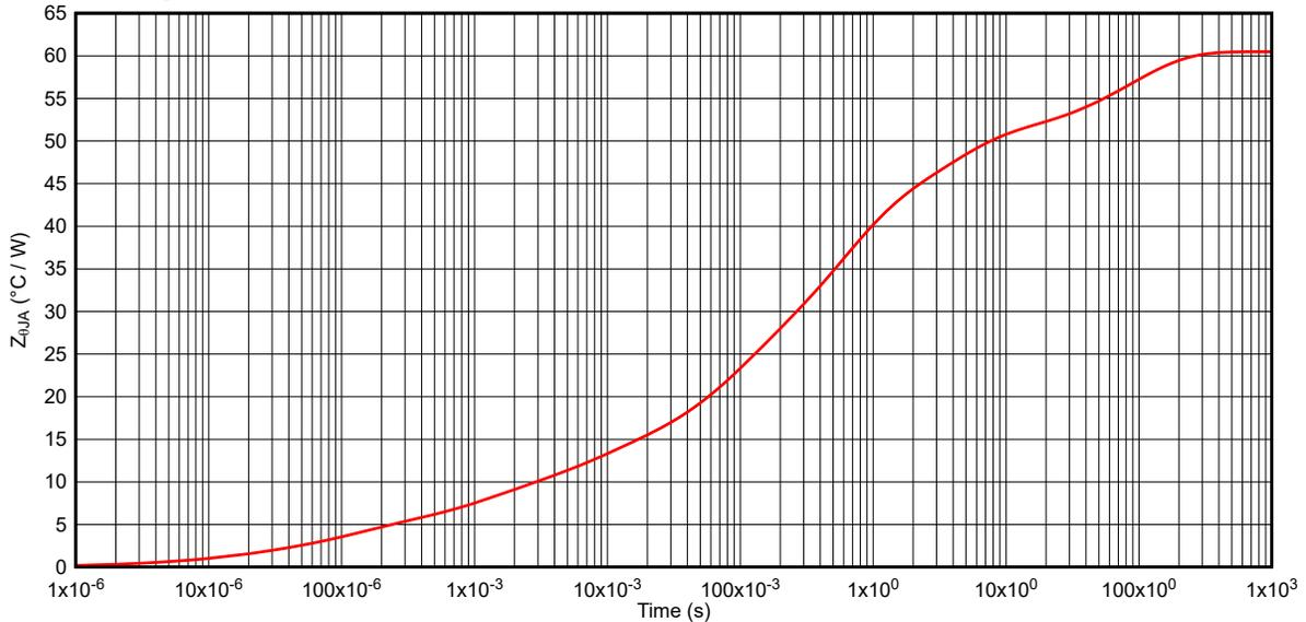
Figure 6-1. TPS1H000-Q1 Transient Thermal Impedance  $Z_{\Theta JA}$
