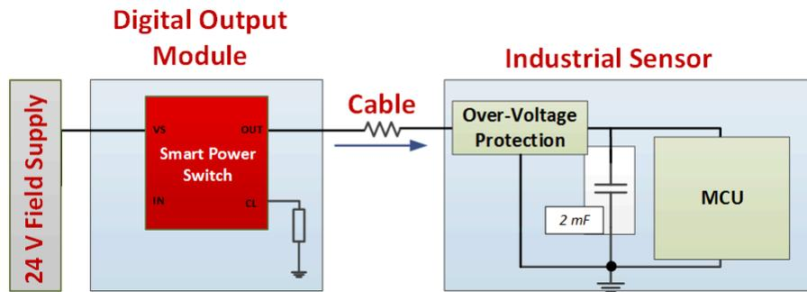
**Figure 3-2. Industrial Capacitive Load Driving Example**
