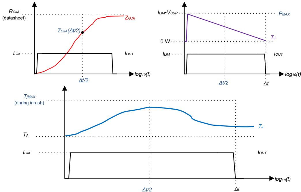
**Figure 3-15.  $R_{\theta JA}$  and Junction Temperature During an Inrush Period**
