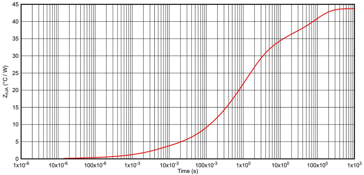
**Figure 6-4. TPS1H100-Q1 Transient Thermal Impedance  $Z_{\Theta JA}$**
