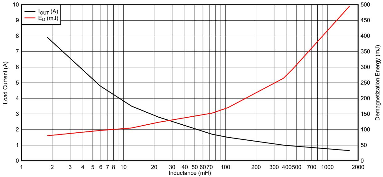
Figure 6-17. TPS1HA08-Q1 Demagnetization Energy Capability
