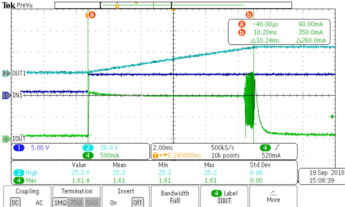
Now the capacitor charges fully without allowing the output current to exceed 1A and without adding significant DC series resistance to the system. Due to the FET heating up during this charging period some ringing occurs at the end because of the high temperature transition between the internal MOSFET modes of operation, however this poses no risk to the system due to the short transient length. The TPS2H160-Q1 has an on-
