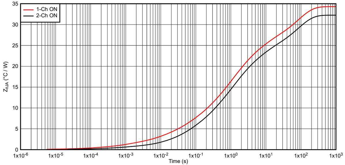
Figure 6-13. TPS2HB16-Q1 Transient Thermal Impedance  $Z_{\theta JA}$
