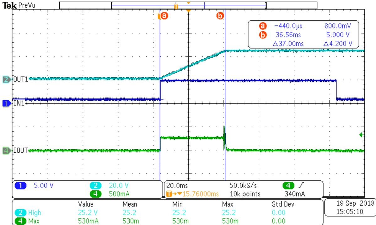
Figure 3-10. TPS2H160-Q1 Current Limiting at 500 mA
