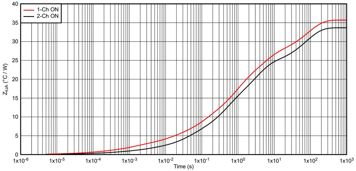
Figure 6-11. TPS2HB35-Q1 Transient Thermal Impedance  $Z_{\theta JA}$
