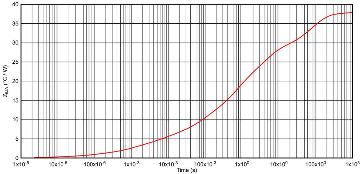
Figure 6-8. TPS1HB50-Q1 Transient Thermal Impedance  $Z_{\Theta JA}$
