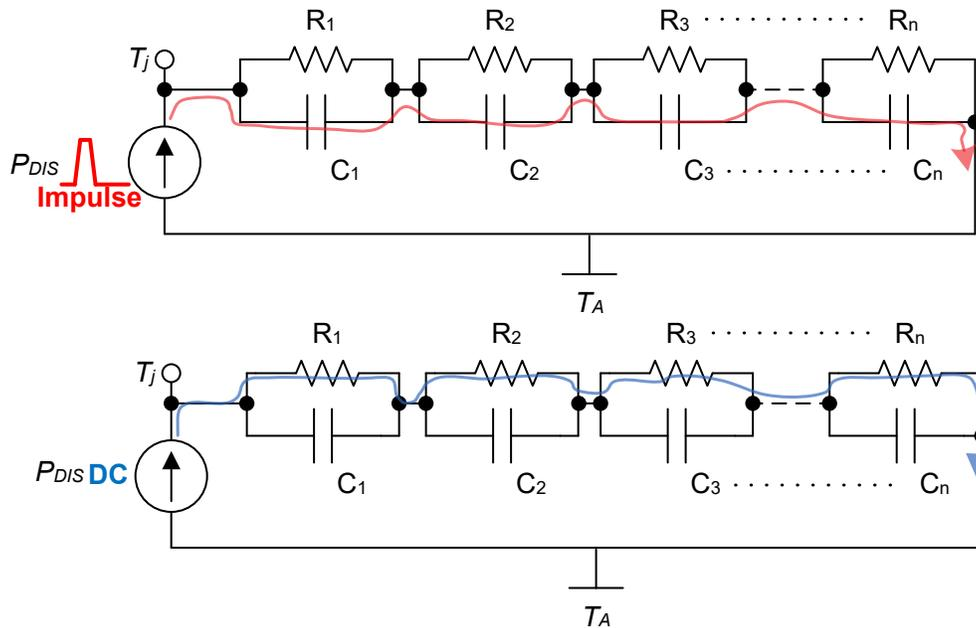
**Figure 3-14. Effect of Thermal Time Constant on  $R_{\theta JA}$  and Junction Temperature**
