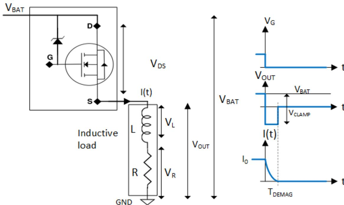
**Figure 4-3. Inductive Load Turn-Off Phase**
