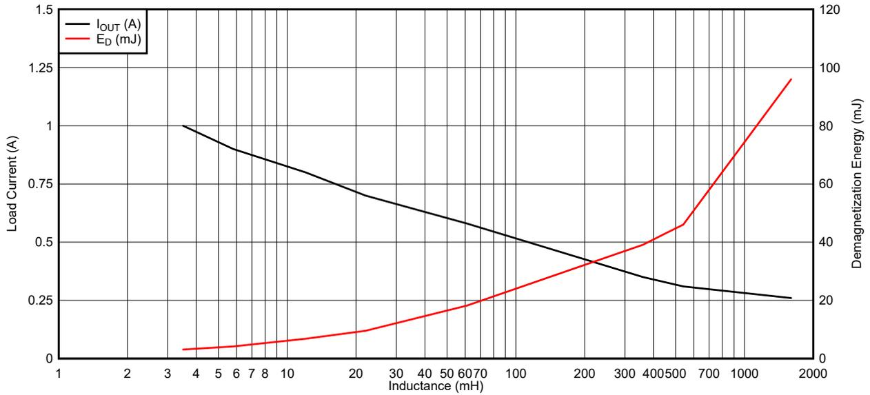
**Figure 6-19. TPS4H000-Q1 Demagnetization Energy Capability**
