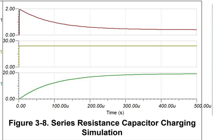
The addition of a 12Ω current limiting resistor limits the peak current to less than 2A, but is not a viable solution due to the power dissipation and voltage drop over the additional 12-Ω resistance. With a 500mA DC load this adds 3W of additional power dissipation and a 6V drop over the resistor. This heat dissipation and voltage drop are not acceptable in the majority of applications.
