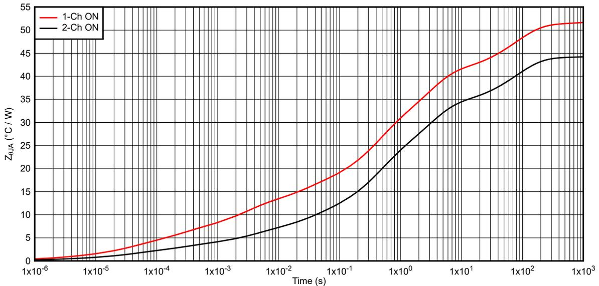
Figure 6-2. TPS2H000-Q1 Transient Thermal Impedance  $Z_{\Theta JA}$
