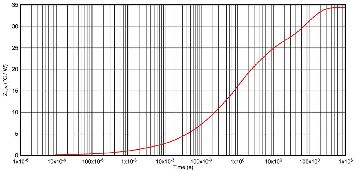
Figure 6-12. TPS1HB16-Q1 Transient Thermal Impedance  $Z_{\theta JA}$
