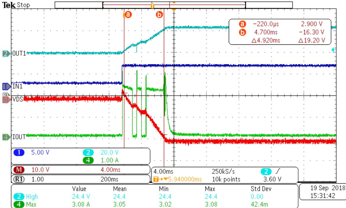
Figure 3-18. TPS2H160-Q1 Thermal Shutdown While Driving Capacitance
