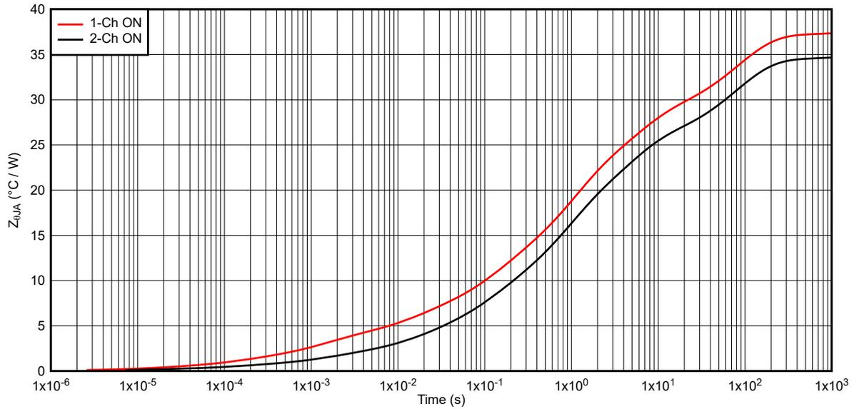
Figure 6-9. TPS2HB50-Q1 Transient Thermal Impedance  $Z_{\theta JA}$
