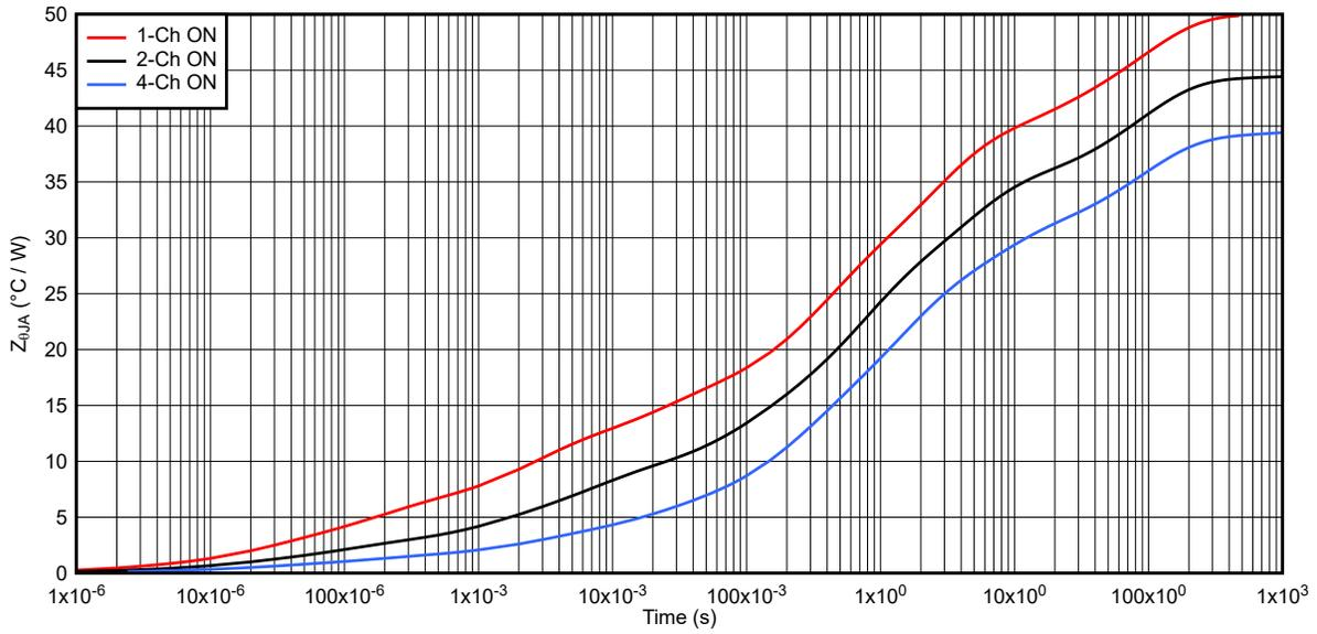
**Figure 6-3. TPS4H000-Q1 Transient Thermal Impedance  $Z_{\Theta JA}$**
