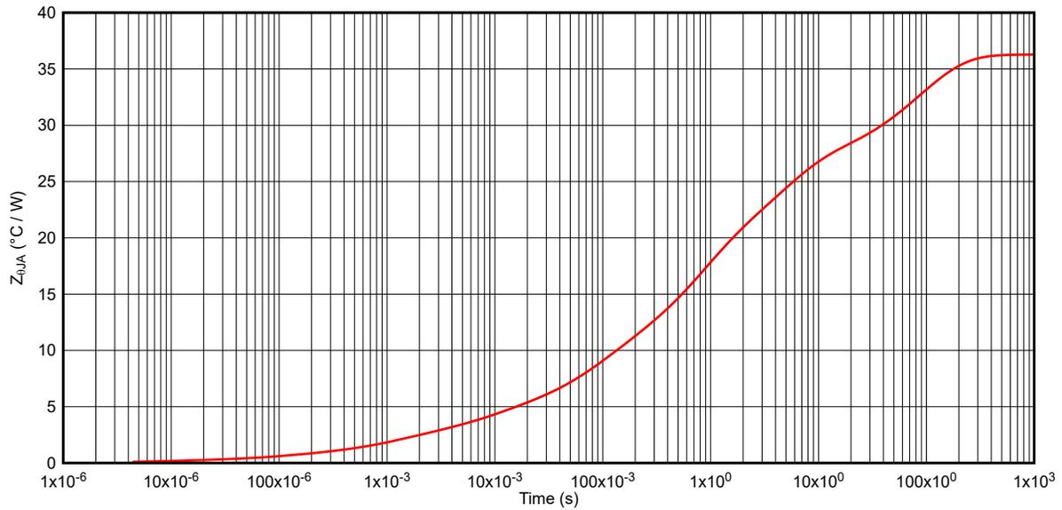
Figure 6-10. TPS1HB35-Q1 Transient Thermal Impedance  $Z_{\theta JA}$
