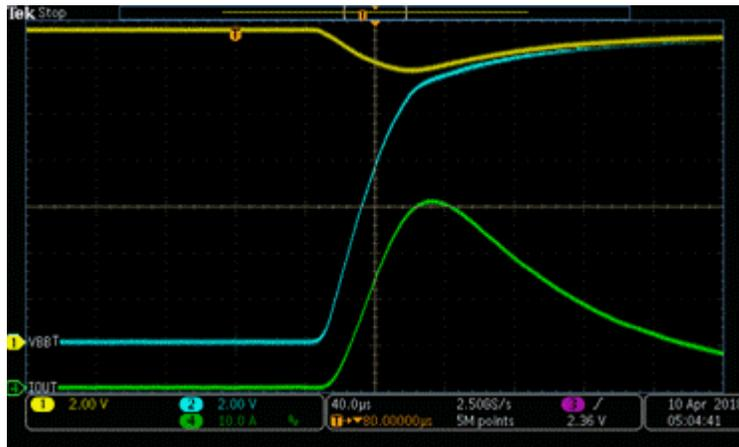
Figure 3-4. Inrush Supply Droop Example
