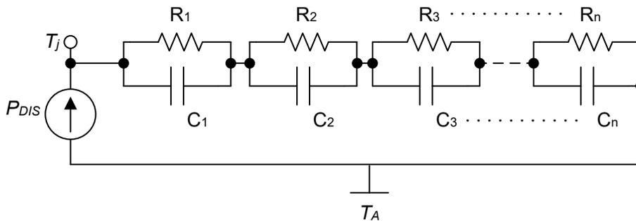
**Figure 3-13. Foster Network Model of Device Thermal Impedance**
