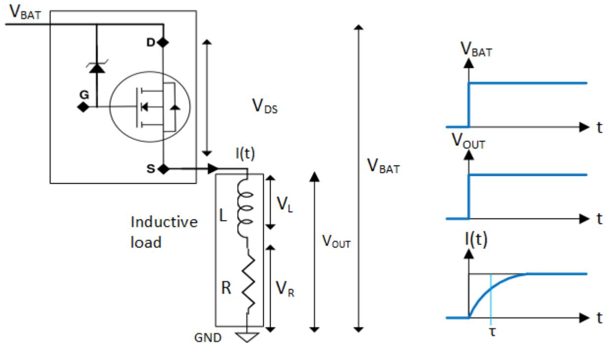
Figure 4-2. Inductive Load Turn-On Phase
