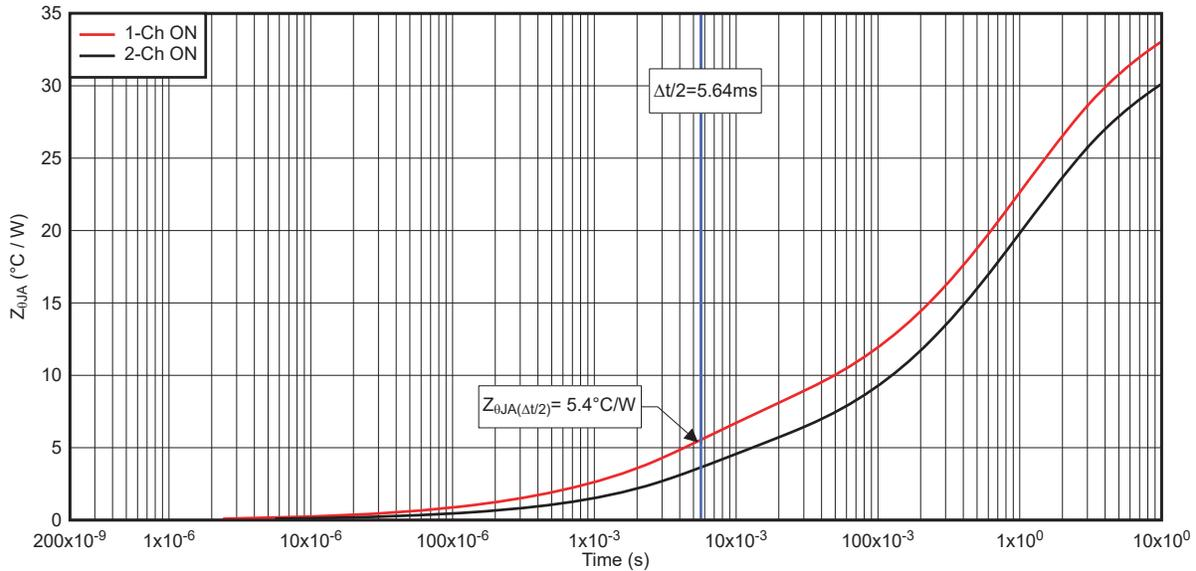
**Figure 3-16. Estimating  $Z_{\Theta JA(\Delta t/2)}$  from TPS2H160-Q1 Transient Thermal Impedance Curve**
