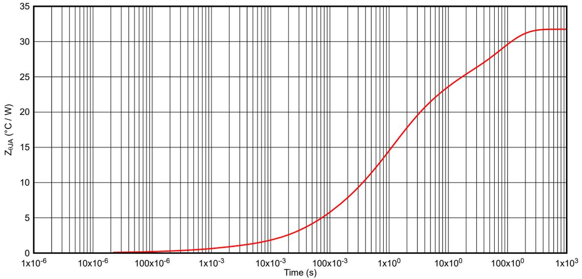
Figure 6-15. TPS1HB08-Q1 Transient Thermal Impedance  $Z_{\theta JA}$
