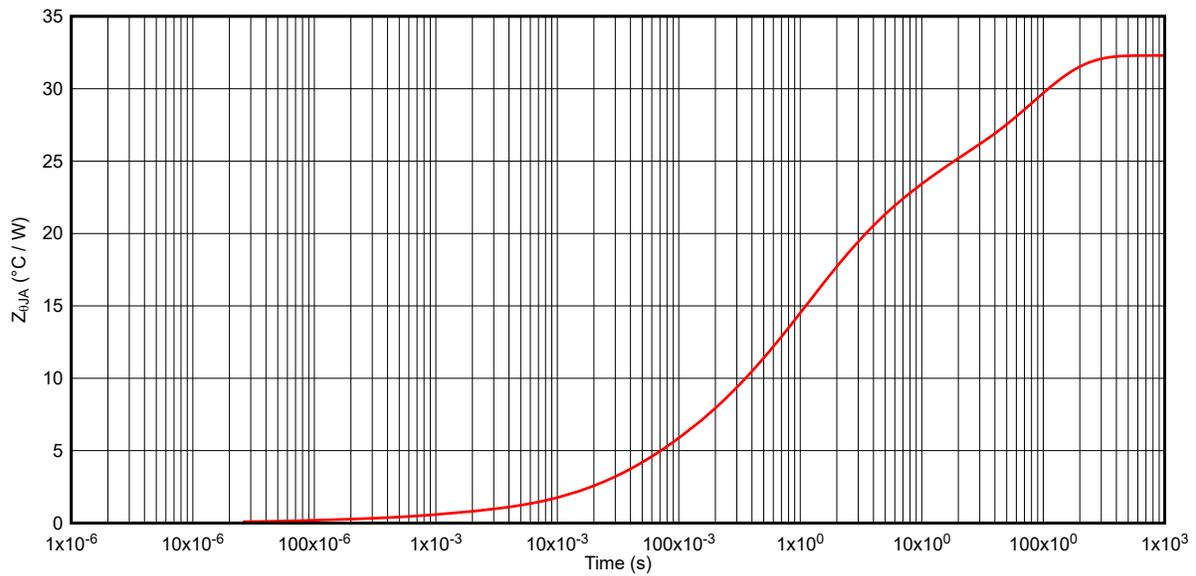
Figure 6-14. TPS1HA08-Q1 Transient Thermal Impedance  $Z_{\theta JA}$
