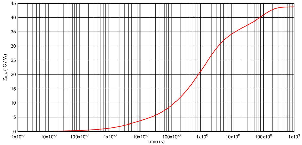
Figure 6-5. TPS1H200-Q1 Transient Thermal Impedance  $Z_{\Theta JA}$
