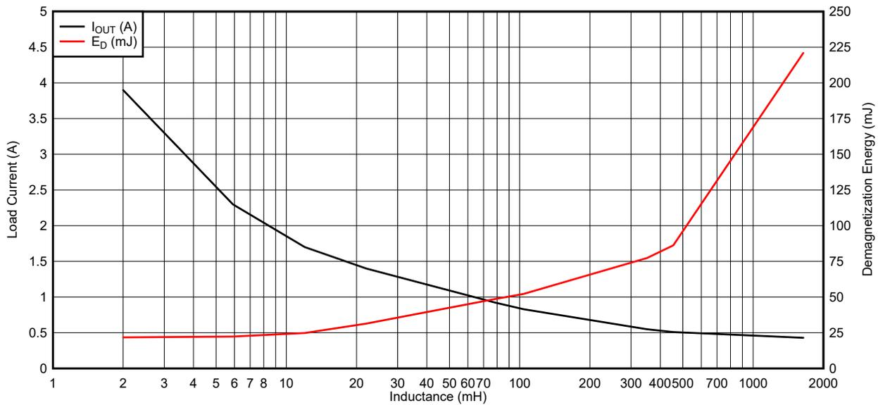
Figure 6-18. TPS2HB50-Q1 Demagnetization Energy Capability
