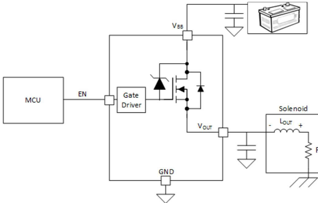
**Figure 4-1. Solenoid Application Example**
