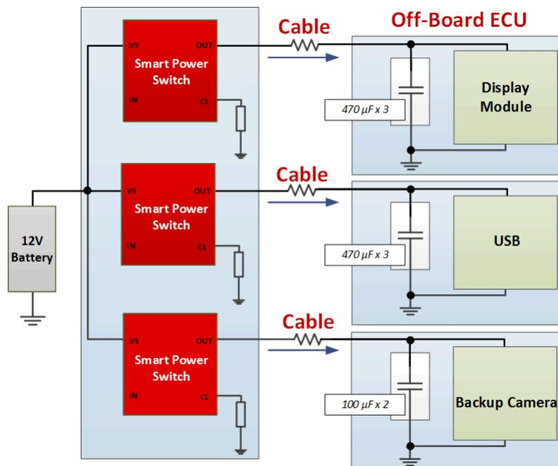
Figure 3-1. Automotive Capacitive Load Driving Example
