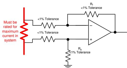
**Figure 2-2. Discrete Current Measurement Implementation**
