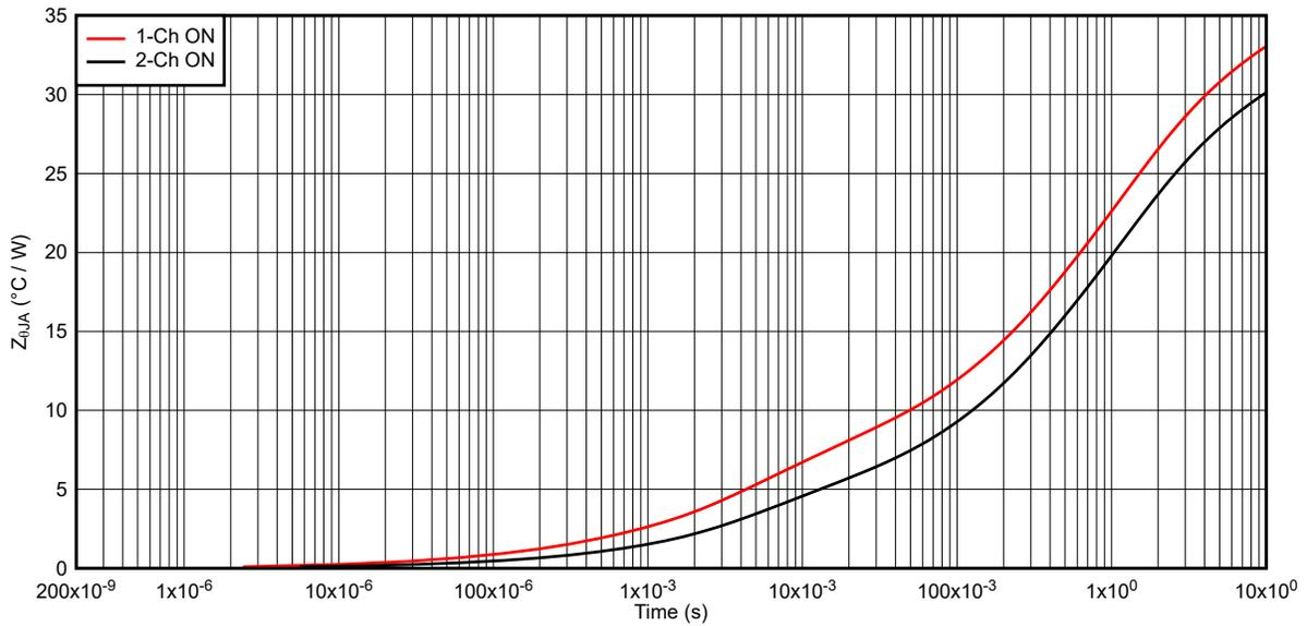
Figure 6-6. TPS2H160-Q1 Transient Thermal Impedance  $Z_{\Theta JA}$
