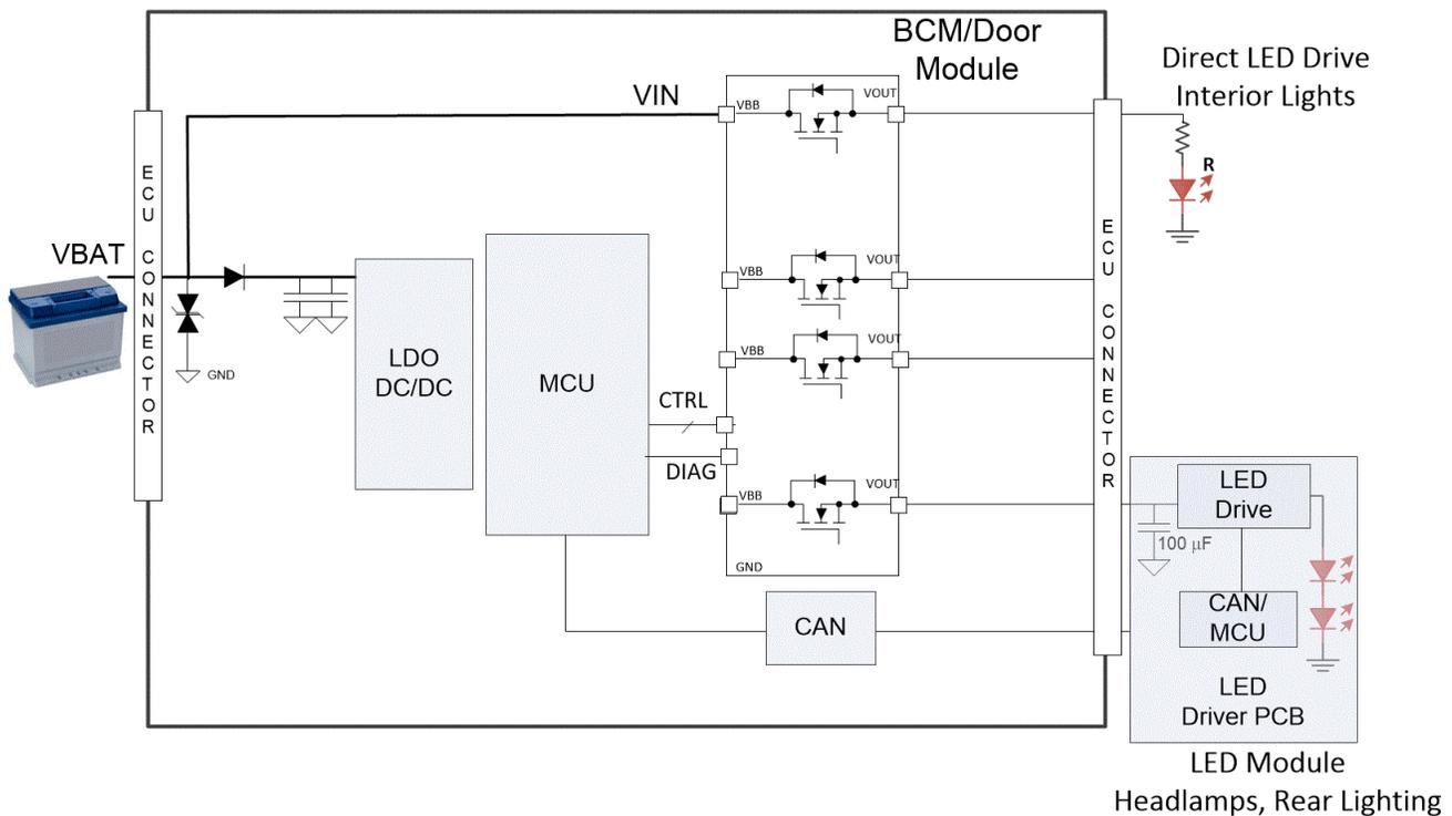
**Figure 5-1. Application Examples of Smart High Side Switches Driving LED Loads**
