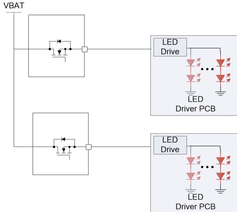
**Figure 5-2. Smart High Side Switches Powering LED Modules**
