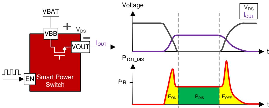
**Figure 2-5. Switching Energy Losses during PWM**
