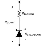
Surge current is generated by the combinational waveform generator outlined in IEC61000-4-X. This current has to be dissipated by the system and more specifically the TVS diode. Since the Flat-Clamp devices have a much lower dynamic resistance the current will be conducted through the device easily while not causing a large clamping voltage for the rest of the system.
