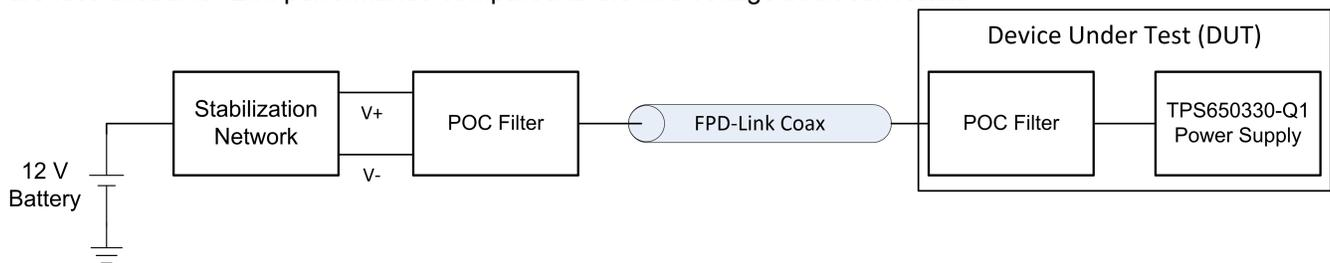
Figure 3-1. CISPR-25 EMC Test Setup
