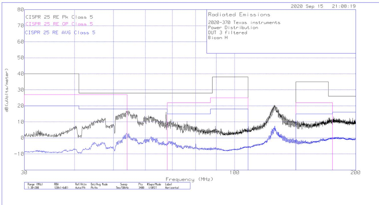
Figure 6-3. Radiated Emissions - Bicon Horizontal Antenna 30 MHz to 200 MHz
