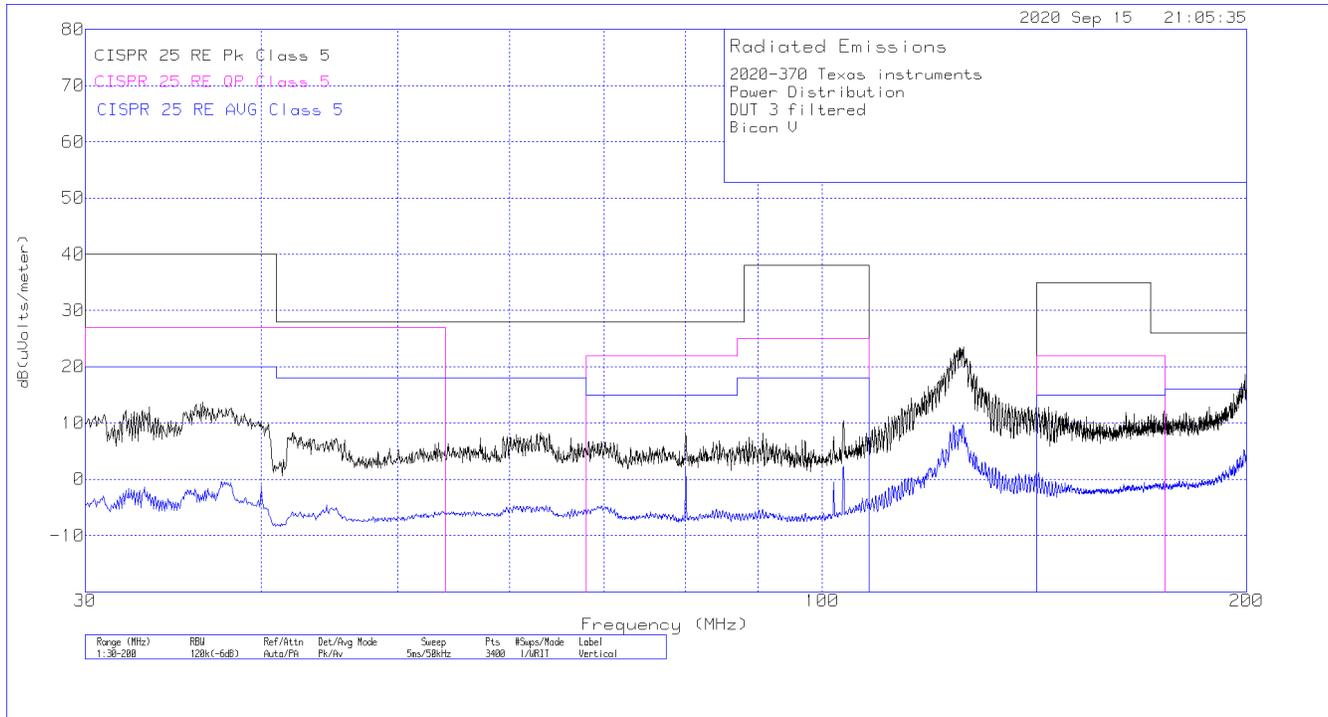
**Figure 6-4. Radiated Emissions - Bicon Vertical Antenna 30 MHz to 200 MHz**
