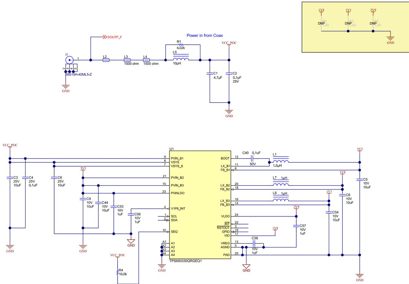
Figure 3-2. DUT Schematics
