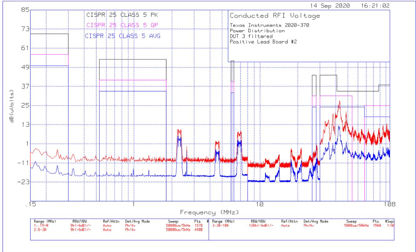
**Figure 6-1. Conducted Emissions 0.15 MHz to 108 MHz**
