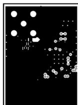
**Figure 3-9. Printed Circuit Board Layer 7 (Ground Plane)**
