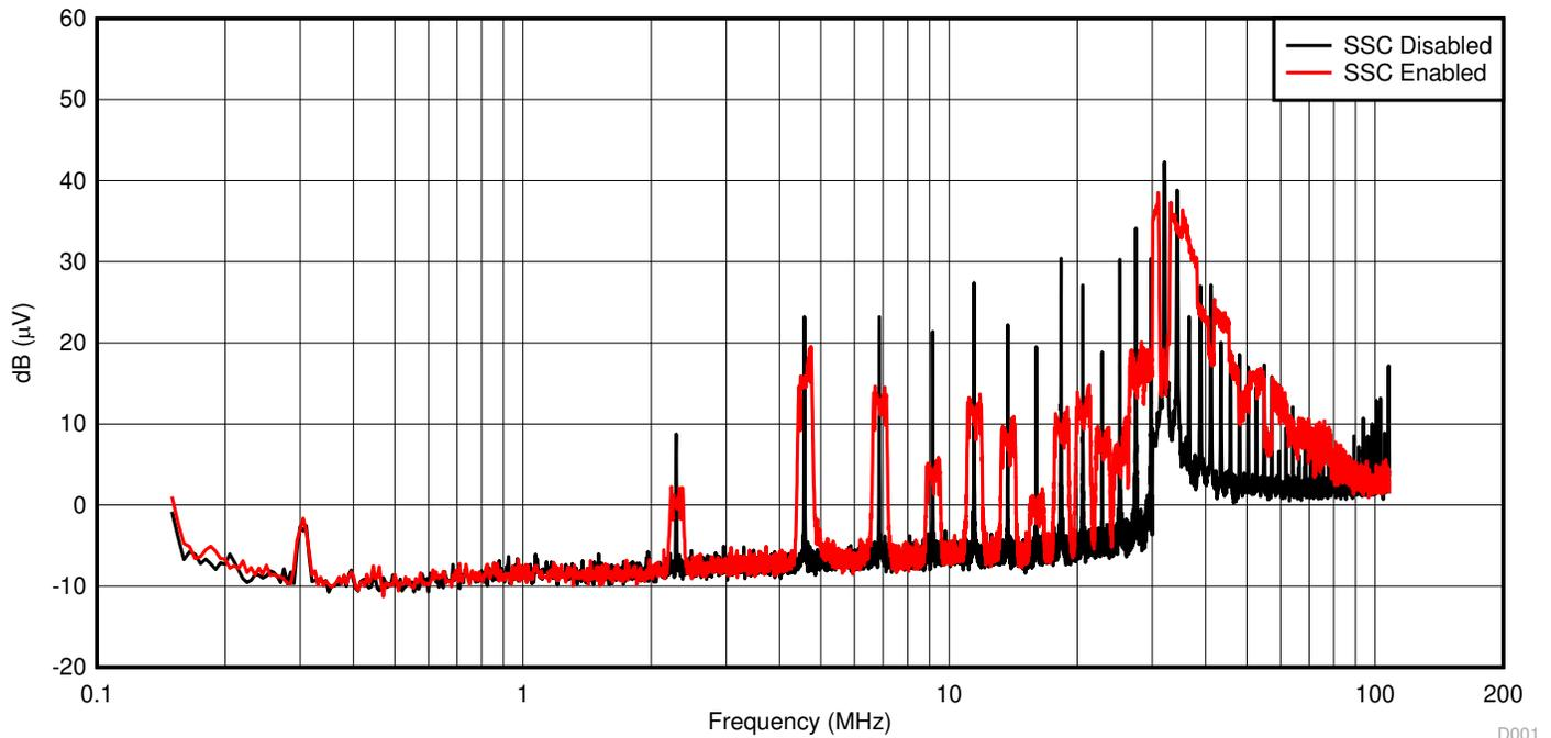
Figure 2-2. TPS650330-Q1 SSC Conducted Emission Comparison
