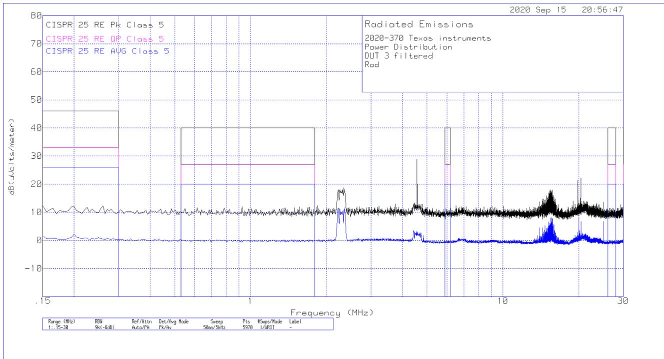
Figure 6-2. Radiated Emissions - Rod Antenna 0.15 MHz to 30 MHz
