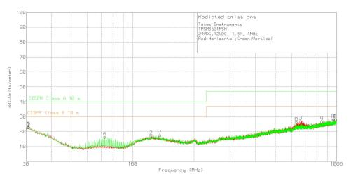
Figure 2-1. Radiated Emissions 24-V Input, 12-V Output, 1.5-A Load
