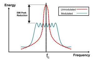
Figure 3-1. EMI Reduction by Spread Spectrum, Frequency Modulation
