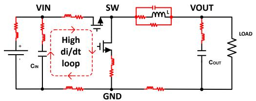
Figure 1-1. Buck Converter With Parasitic Elements
