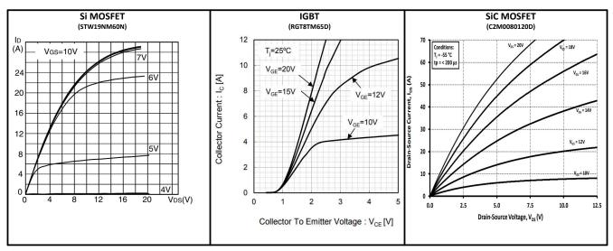
Figure 2-2.  $I_D$  vs  $V_{DS}$  Curves
