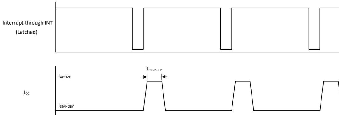
**Figure 2-4. Timing Diagram for Conversion on Demand**
