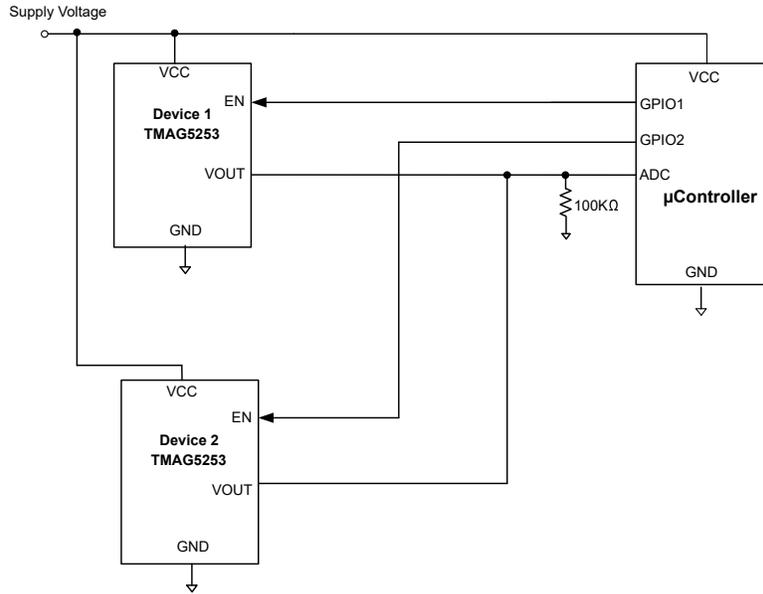
**Figure 3-1. Multiple Sensors Connected Together in Same Bus**
