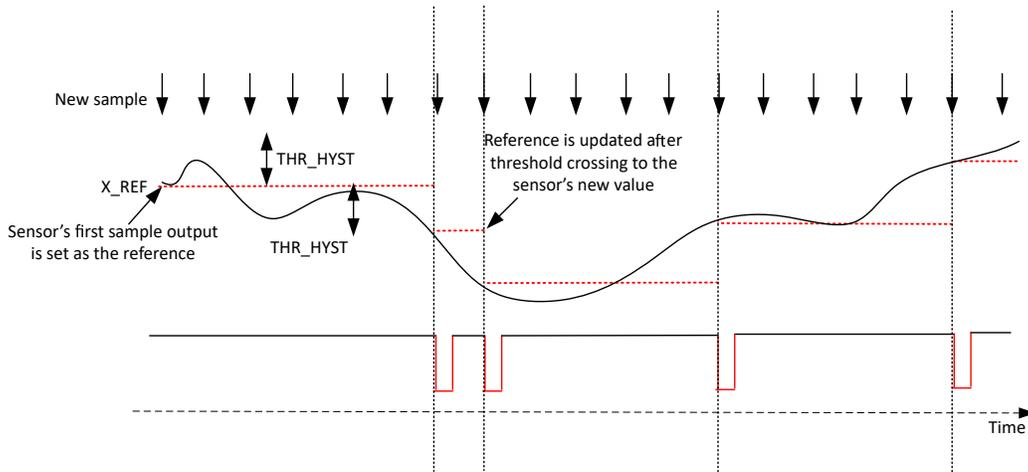
**Figure 2-6. TMAG3001 Wake on Change with Magnetic Axes Measurements**
