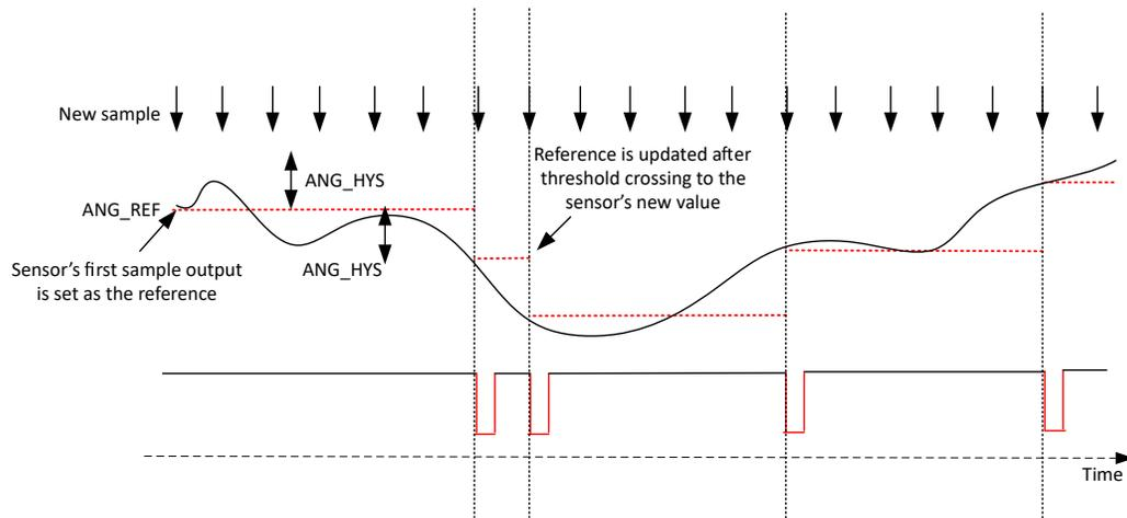
**Figure 2-7. TMAG3001 Wake on Change with Angle Measurements**
