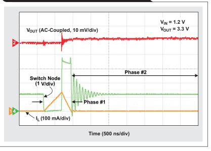
switching time (phase #1), the average input current over this time must be higher than the IC's  $I_Q$ . However, because the duration of phase #1 is very short, the average input current is usually only slightly greater than the input current that is due to the  $I_Q$ .
