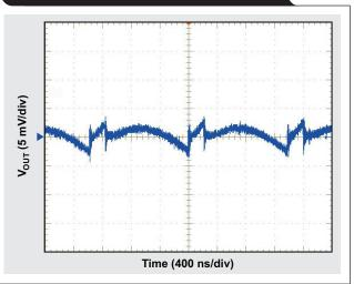
Figure 4. Original switch-node waveform for the TPS54824
