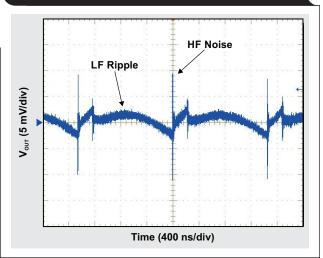
capacitance. The HF noise comes from the coupling of the switch node's high-frequency ringing through the parasitic capacitance of the inductor (the oscilloscope must have enough bandwidth to capture this, typically  $\geq$ 200 MHz).
