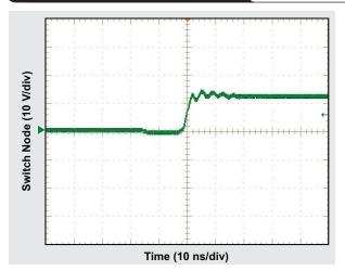
Reducing the ringing also reduces the output ripple because the high-frequency noise correlates to the ringing. Figure 6 shows the output ripple with the boot resistor added.
