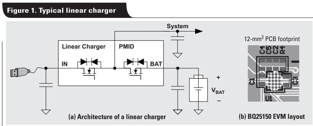
During normal operation with an input present, the first switch turns on and shorts the input to PMID, while the second switch modulates its resistance in order to regulate the current and voltage at the battery output.
