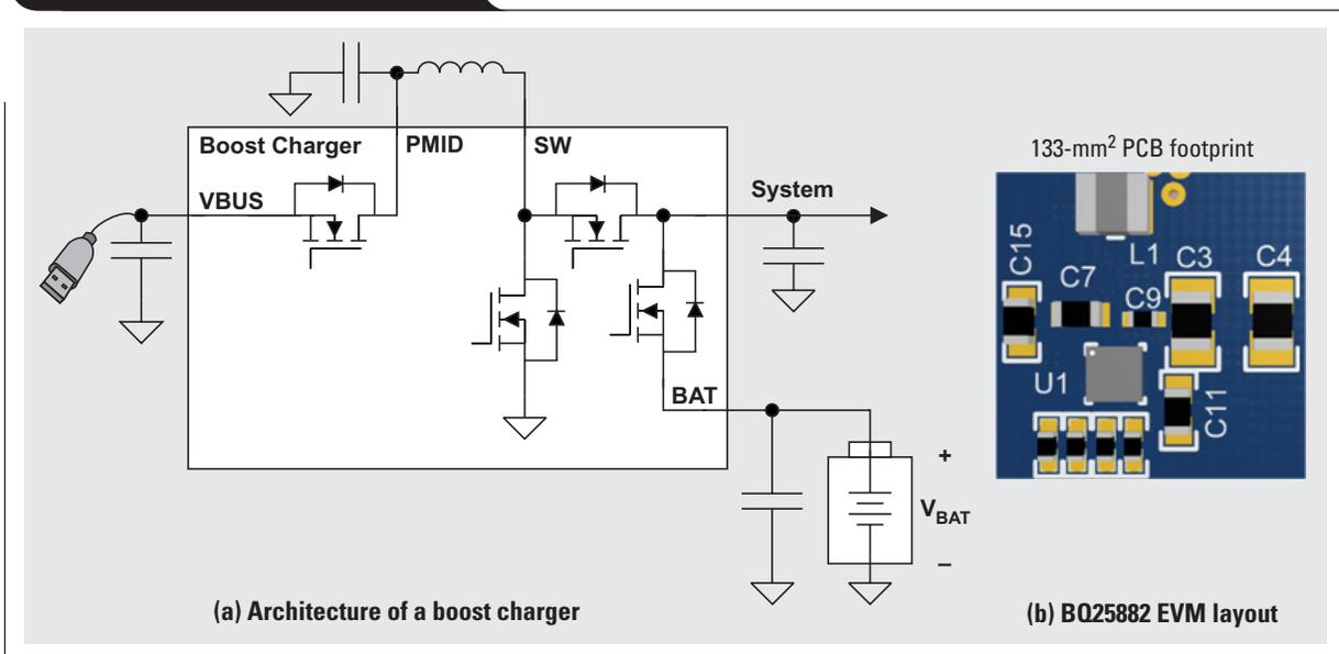
Figure 7. Typical buck-boost charge controller
