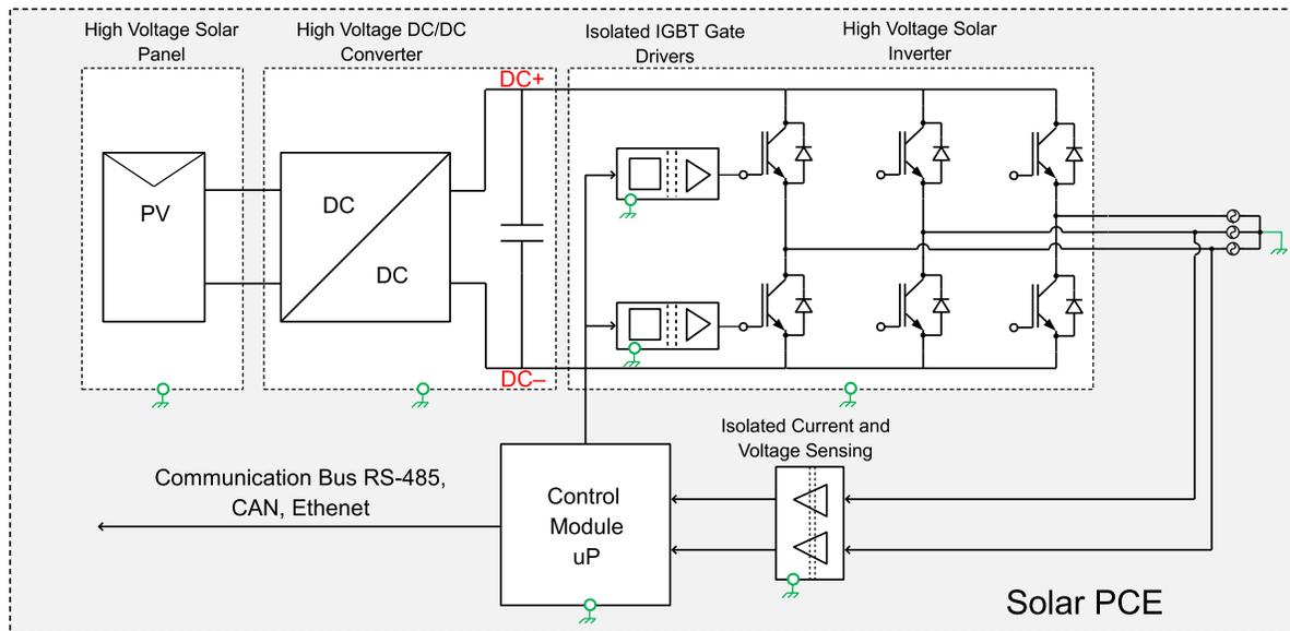
**Figure 1.** Typical system block diagram of a transformer-less solar power conversion system.
