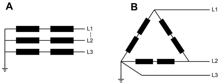
**Figure 4.** (a) A star-earthed TN system that is neutral-earthed; and (b) a corner-earthed TN system where one phase is earthed.
