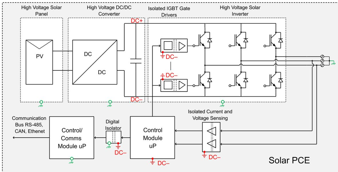
**Figure 2.** Alternative system block diagram of a transformer-less solar power conversion system.
