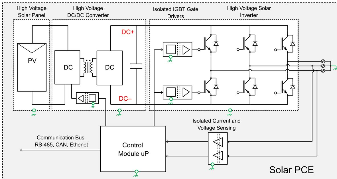
**Figure 3.** System block diagram of a transformer-based solar power conversion system.
