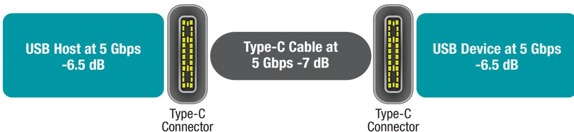
Figure 4. USB 3.0 at 5 Gbps USB Type-C channel-loss budget.
