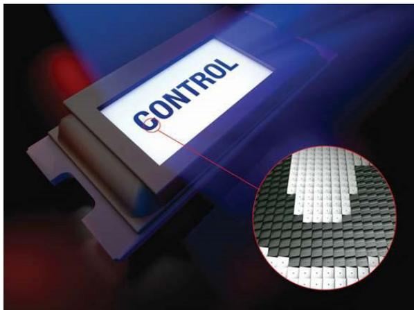
**Figure 1.** DLP technology involves the high-speed control of millions of micromirrors for high-resolution images.
