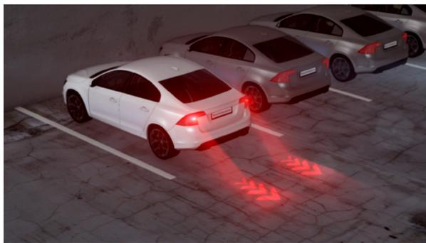
**Figure 4.** A driver can broadcast their intended trajectory by projecting a path on the ground behind their vehicle through the rear lights.
