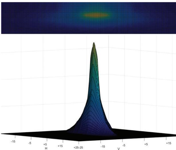
**Figure 3.** Typical high-beam illumination profile with a high-center peak.
