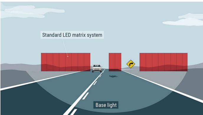
**Figure 2.** Headlight FOV with a background 12-pixel matrix. Each pixel is illustrated with the red segment in the high beam FOV.
