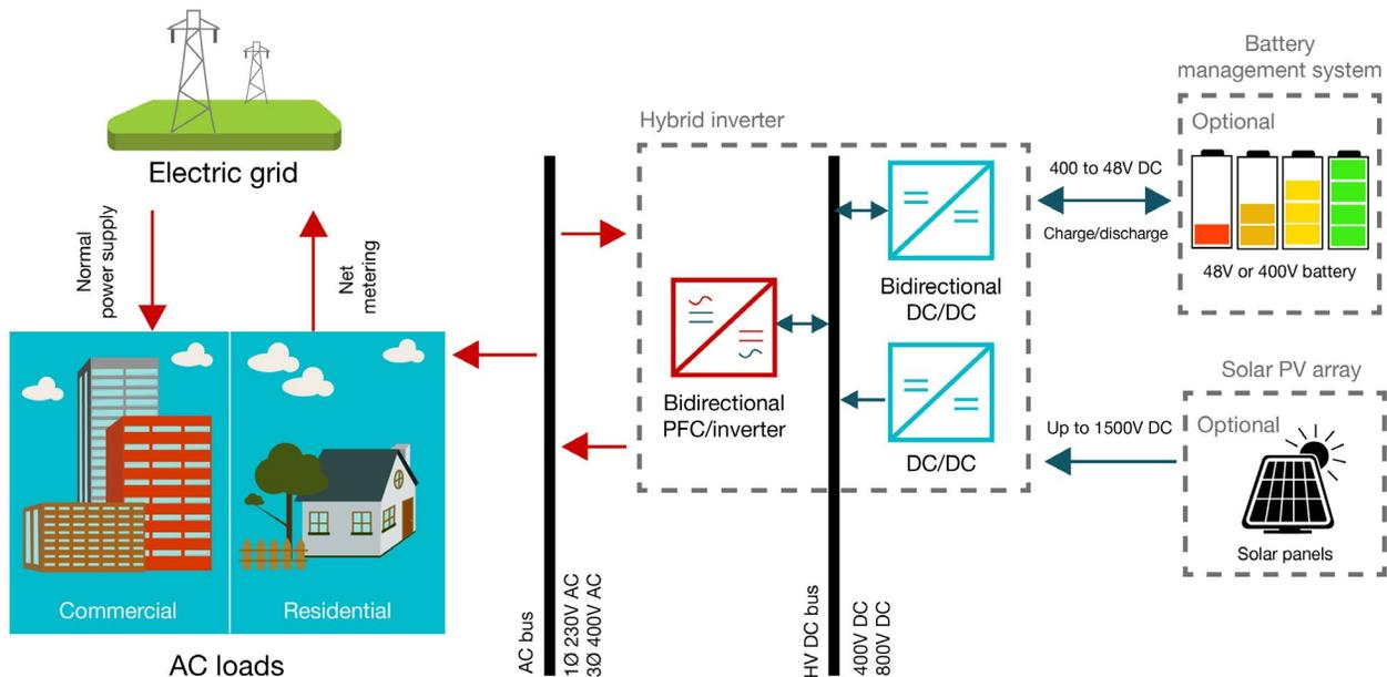
**Figure 1.** Block diagram of a bidirectional PFC and inverter stage.
