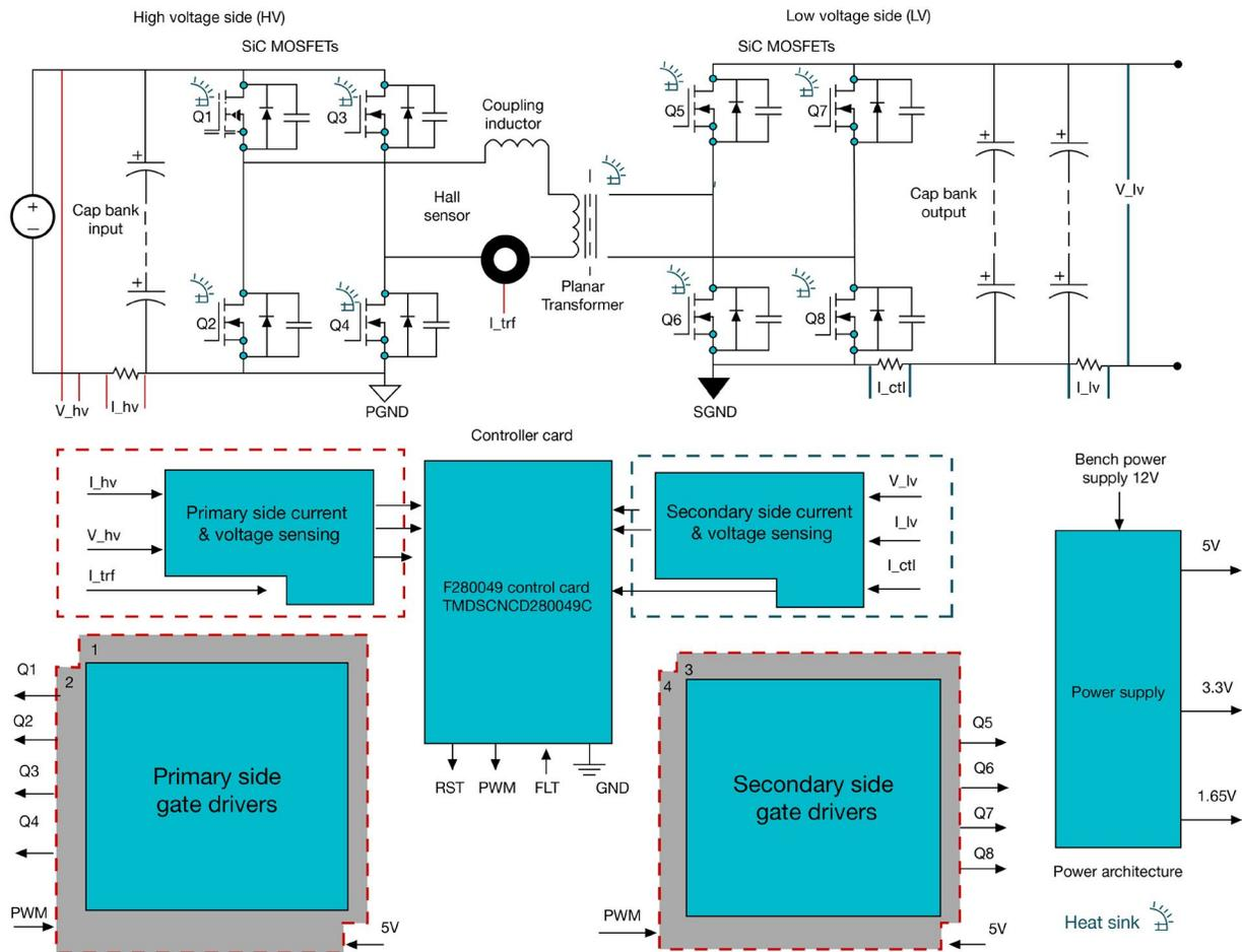
**Figure 2.** A dual active-bridge DC/DC converter design facilitates bidirectional operation to support battery charging and discharging applications.
